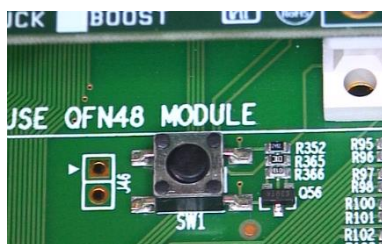
Figure 159: R365 (10 k \Omega ) Added Next to Reset Button
