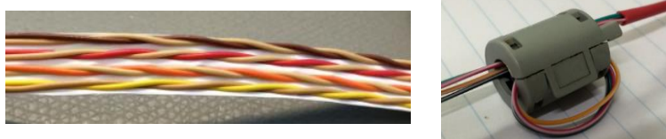
Figure 169: Example of Twisted Pair Cable with 4 Pairs and Ferrite
