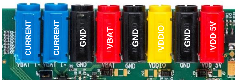
Figure 4: PLT Hardware Power Connections
