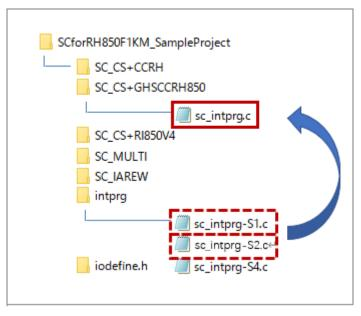
Figure 5.13 Replace the sc\_intprg.c file after rename
