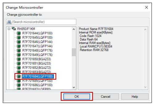
Figure 4.9 Select devices for changing microcontroller
