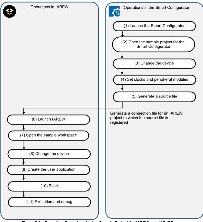
Figure 8.2 Operating Procedure for the Sample Project for IAREW and IAR ICC
