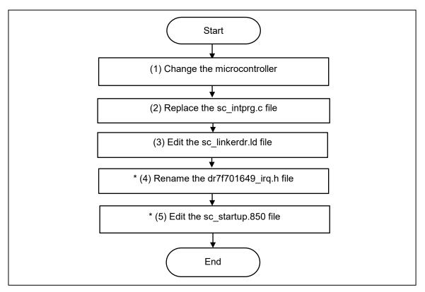
Figure 5.8 Change the Target Device of the Sample Project (CS+ Project)
