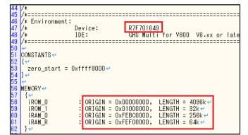
Figure 5.14 Changing the start address and size of the memory
