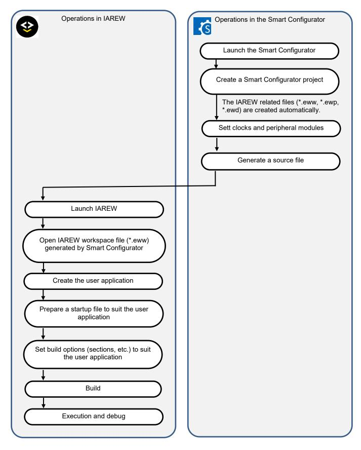
Figure 3.3 Basic Operating Procedure in the IAREW Environment
