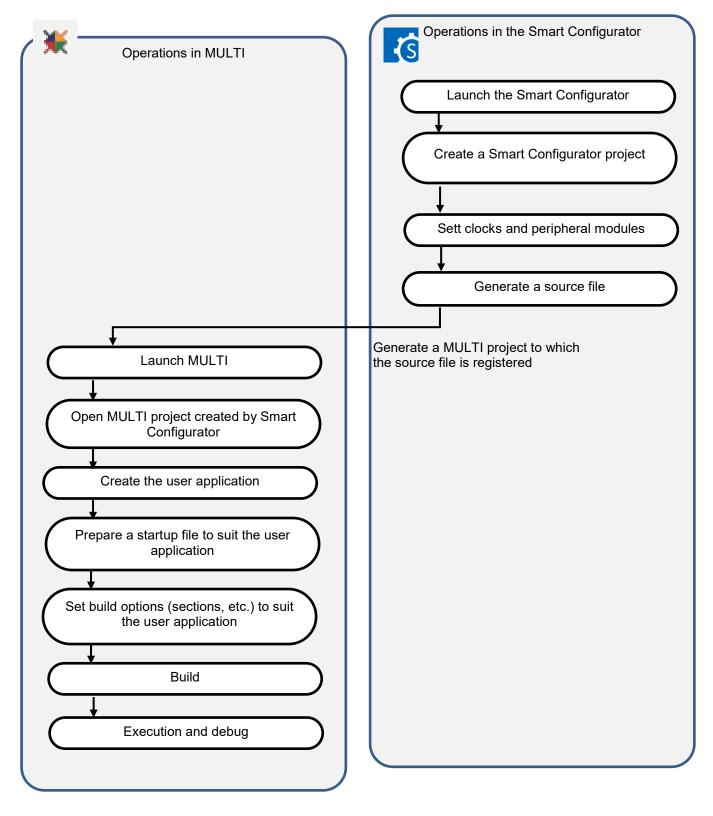
Figure 3.2 Basic Operating Procedure in the MULTI Environment
