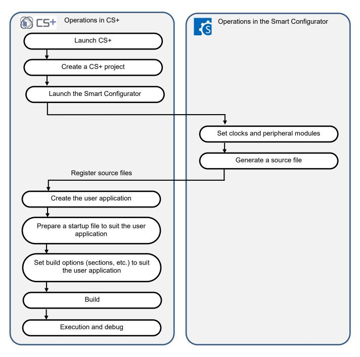
Figure 3.1 Basic Operating Procedure in the CS+ Environment
