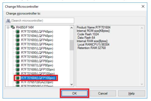
Figure 6.9 Select devices for changing microcontroller
