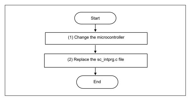
Figure 6.6 Change the Target Device of the Sample Project (CS+ Project)
