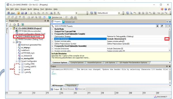
Click on the [Browse...] button in the [Path Edit] dialog box and add iodefine.h and the folder containing the files generated by the Smart Configurator.
