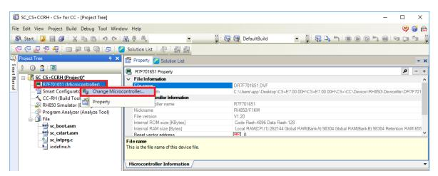
Figure 4.7 Change microcontroller in CS+
