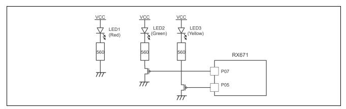
Figure 2-10. LED Circuit
