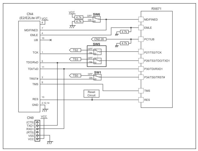
Figure 2-5. RX671 Operating Mode Setting CircuitPower Supply
