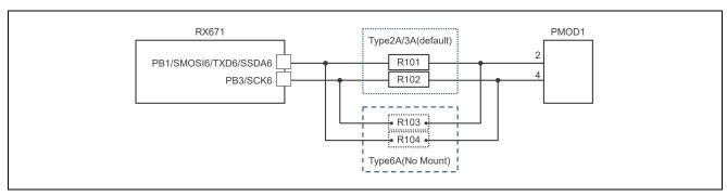
Figure 2-11. PMOD1 Interface Switch Circuit
