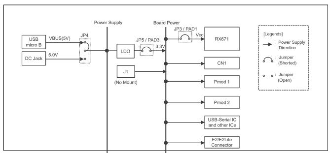
Figure 2-6. Power Source System Diagram
