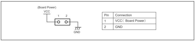
Figure 2-7. J1 Pin Assignments
