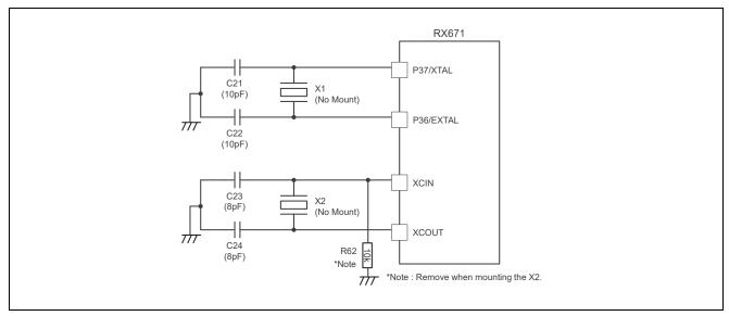
Figure 2-8. Clock Circuit
