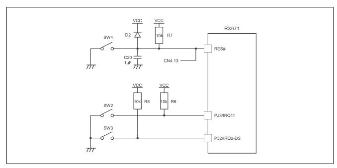
Figure 2-9. Push Switch Circuit
