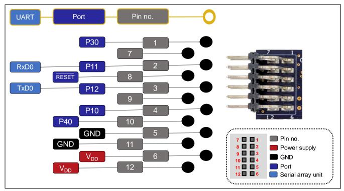
Figure 5-1 Pin Assignments of the Pmod™ Connector
