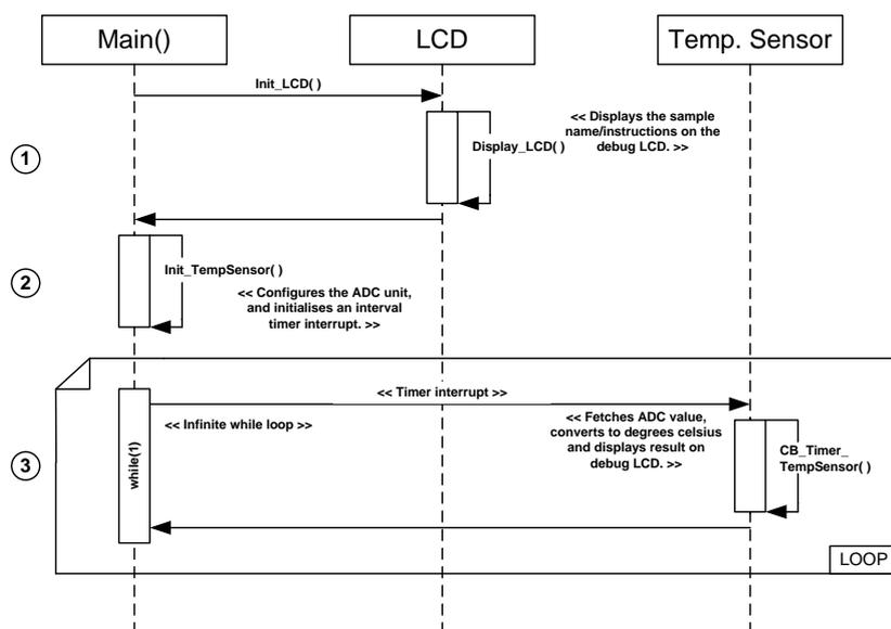
Figure 4-15: Temperature Sensor Sequence Diagram
