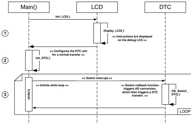
Figure 4-7: DTC Sequence Diagram
