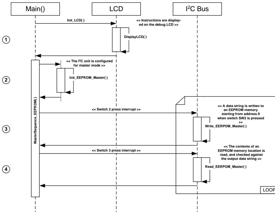
Figure 4-9: IIC\_Master Sequence Diagram
