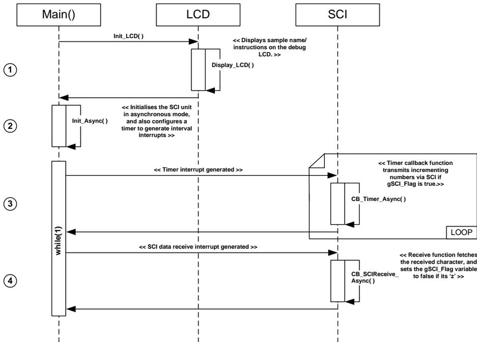
Figure 4-3: Async\_Serial Sequence Diagram
