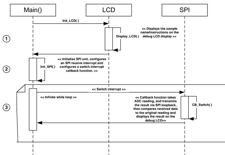
Figure 4-14: SPI Loopback Sequence Diagram
