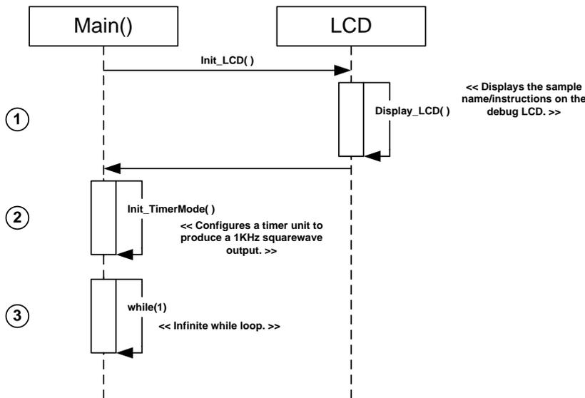
Figure 4-16: Timer Mode Sequence Diagram
