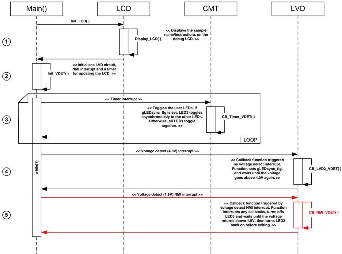
Figure 4-17: LVD Sequence Diagram
