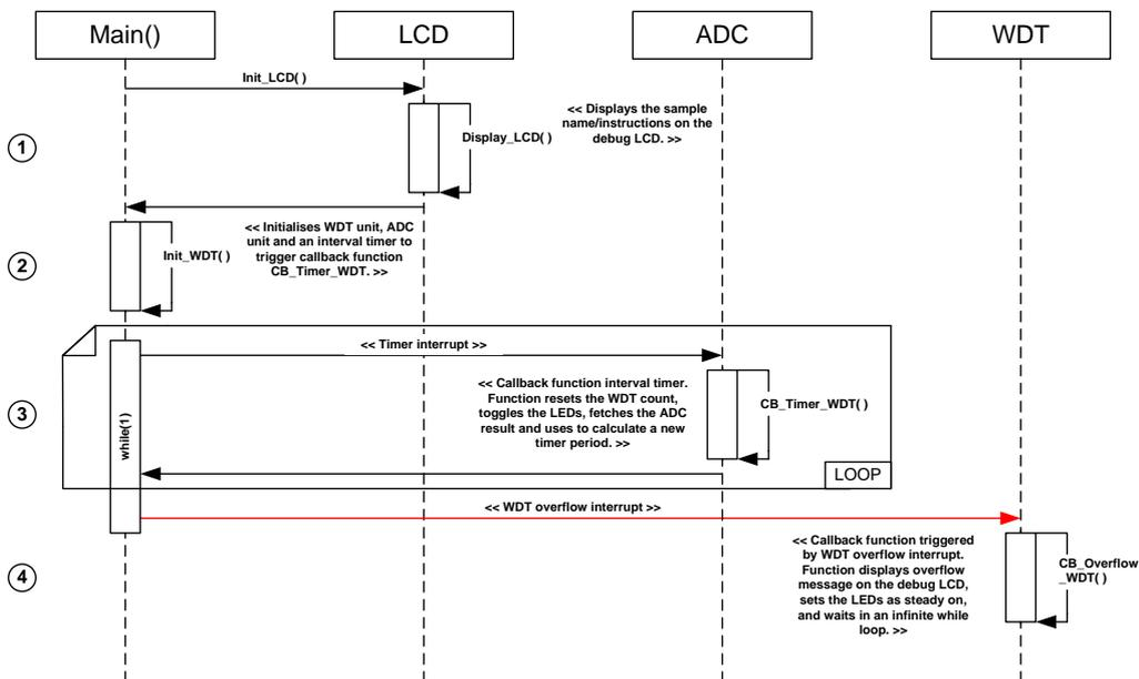
Figure 4-18: WDT Sequence Diagram
