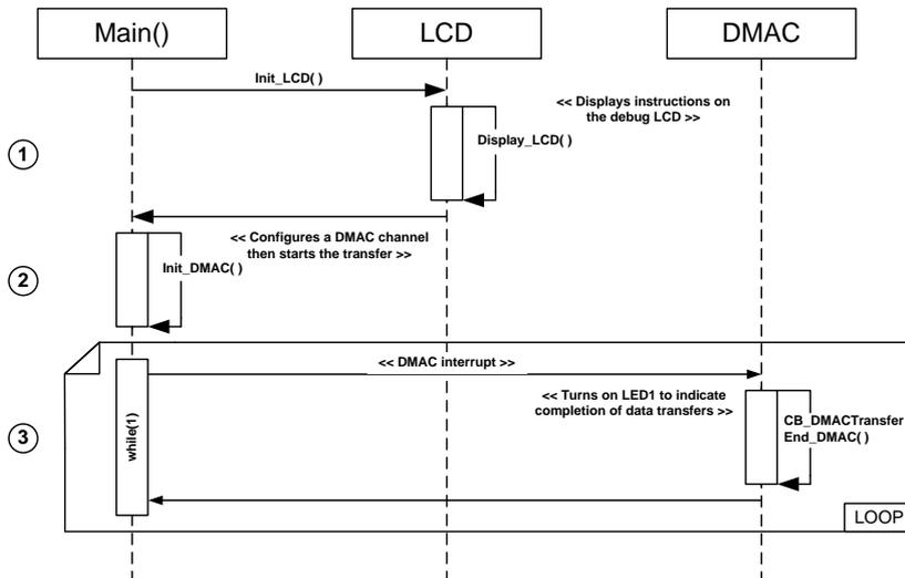
Figure 4-5: DMAC Sequence Diagram
