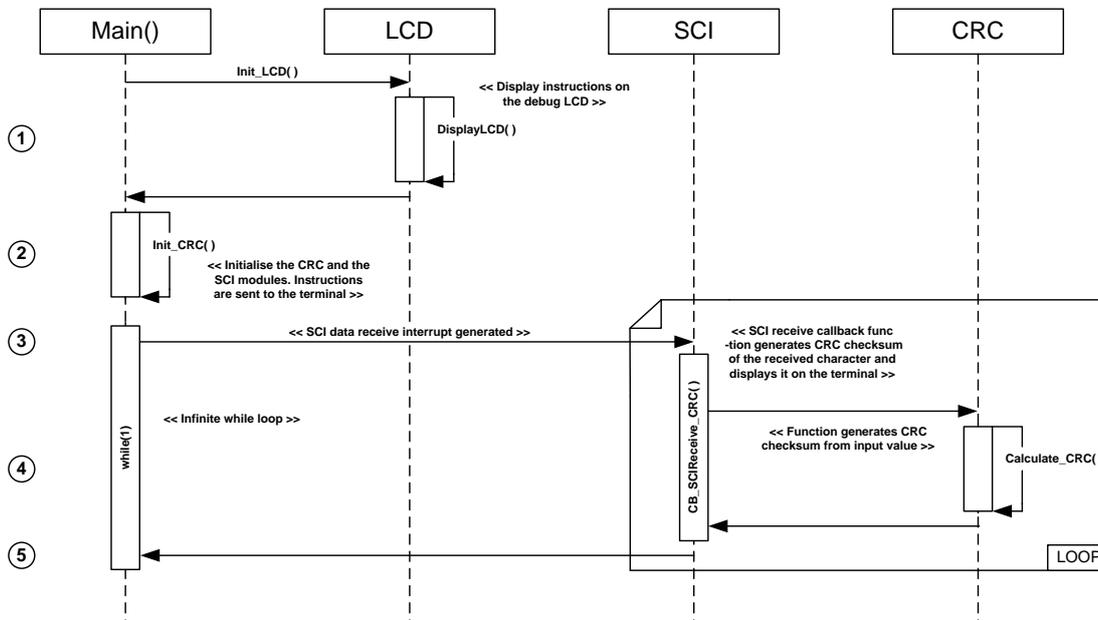
Figure 4-4: CRC Sequence Diagram
