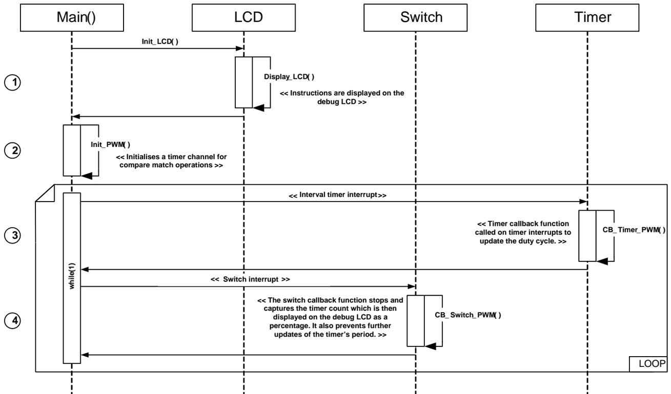
Figure 4-12: PWM Sequence Diagram
