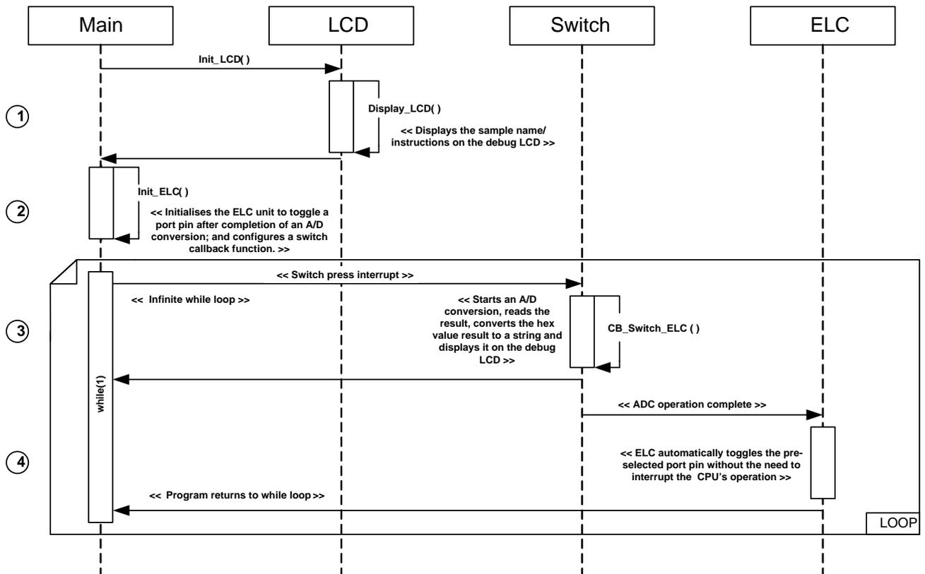
Figure 4-8: Event Link Controller (ELC) Sequence Diagram
