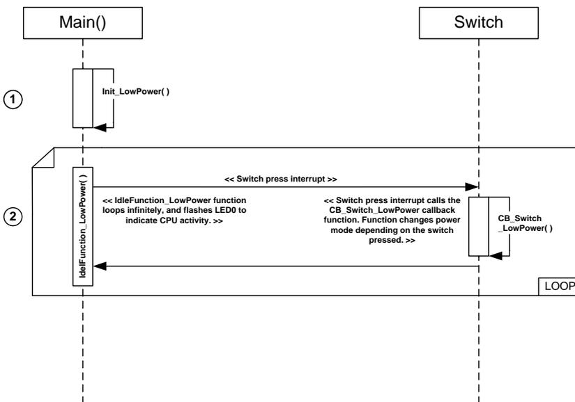
Figure 4-10: Low Power Sequence Diagram
