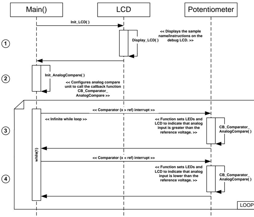
Figure 4-2: Analog\_Compare Sequence Diagram
