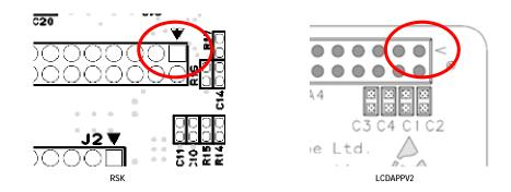
5. The LCDAPPV2 board should be fitted on top of the target RSK, mating the JA4 header and socket together. The nylon pillars should rest on the target RSK PCB.
