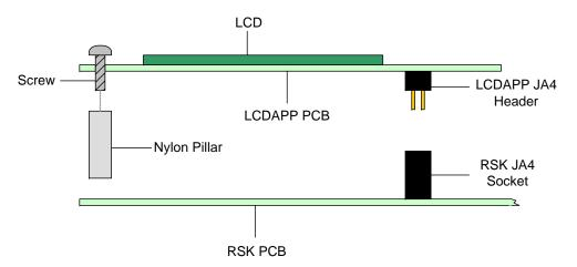
4. Align the LCDAPPV2 board onto of the target RSK, ensuring that pin 1 of JA4 on both boards are in line as shown below.
