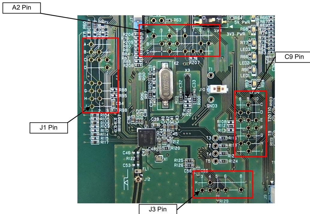
**Figure 5-2: Example of MCU Header pin numbers**
