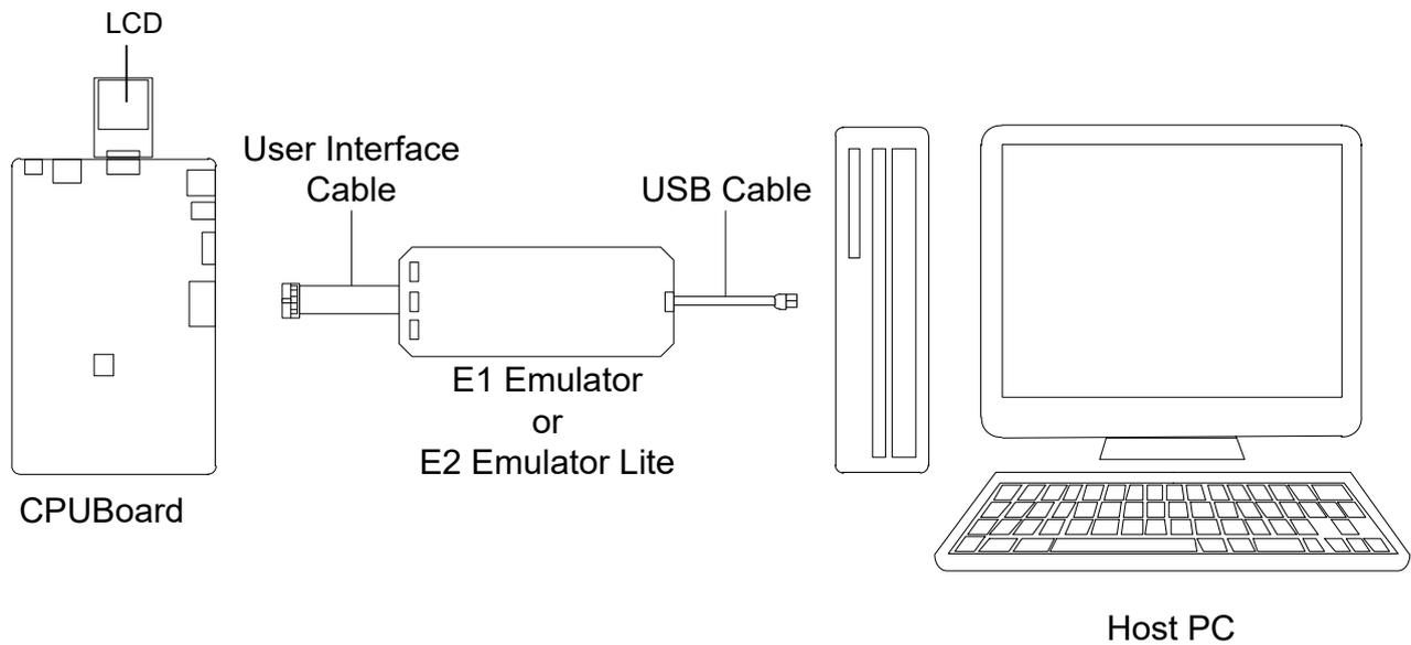
Figure 4-2: Debugger Connection Diagram
