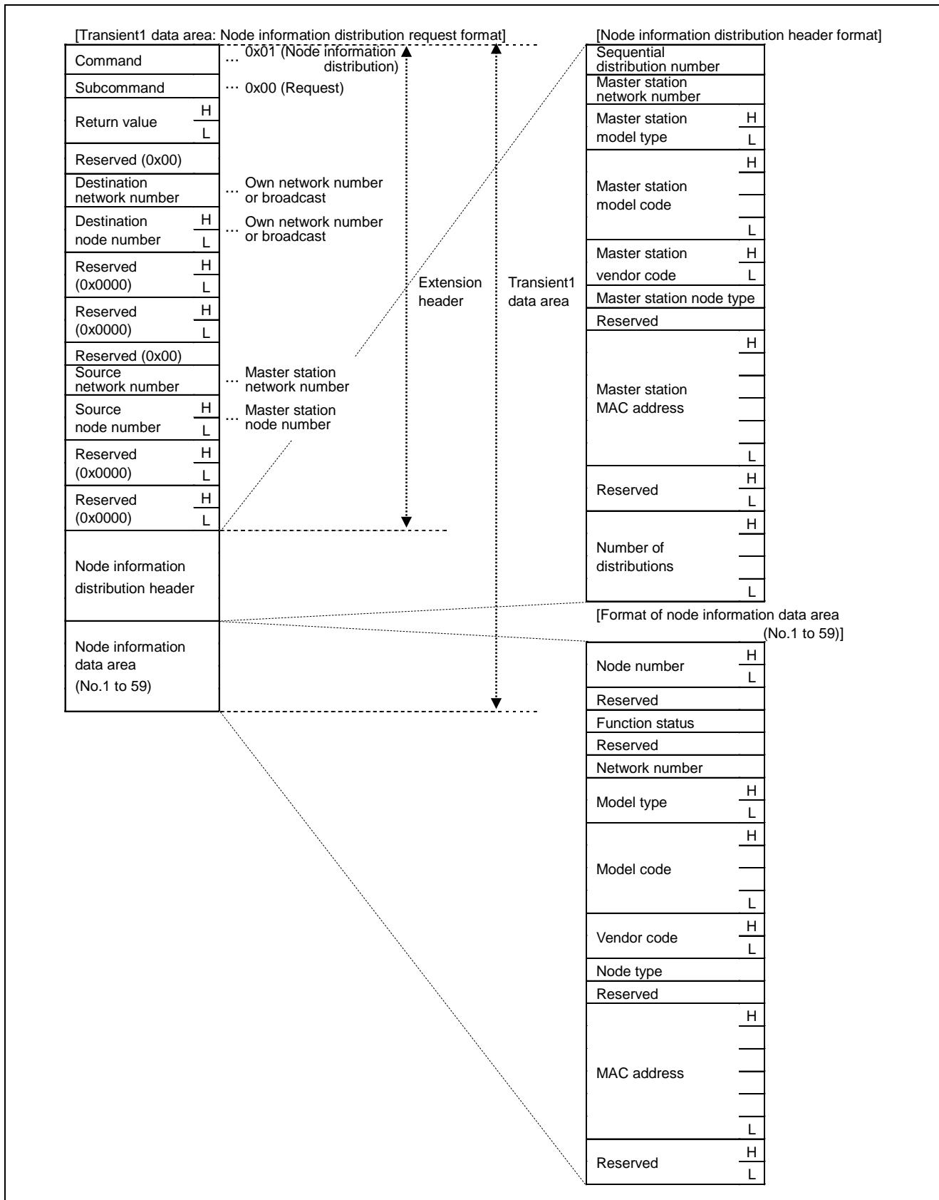
Figure 5.13 Transient1 Data Area: Node Information Distribution Request
