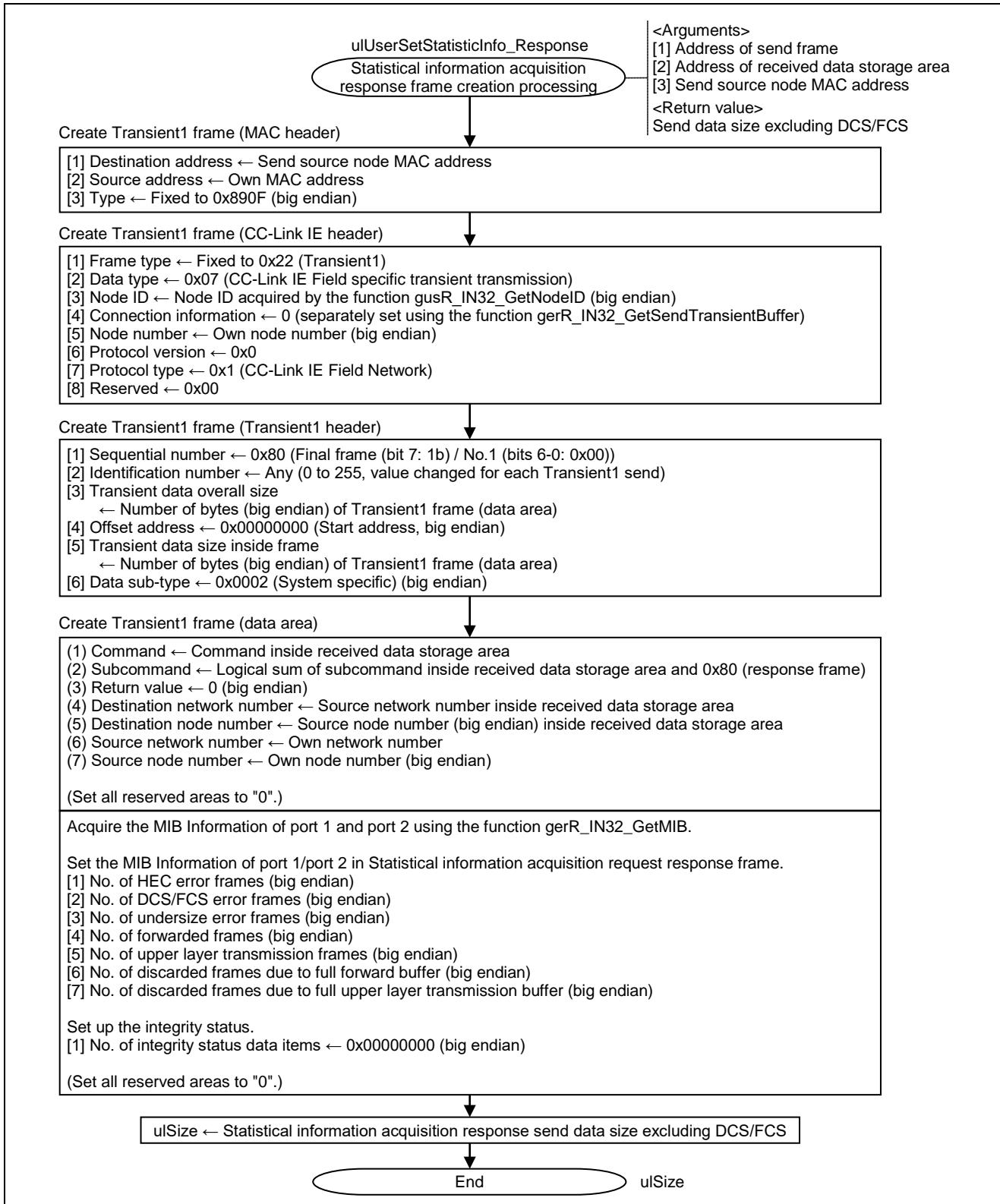
Figure 6.28 Flowchart for Statistical Information Acquisition Response Frame Creation Processing
