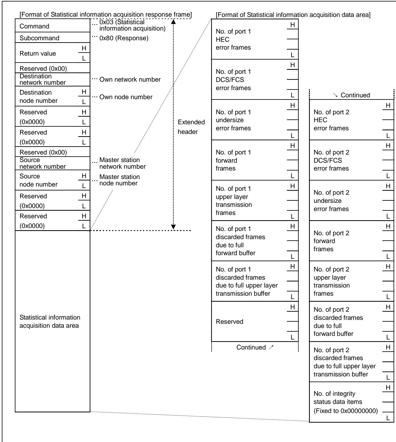
Figure 5.17 Transient1 Data Area: Statistical Information Acquisition Response
