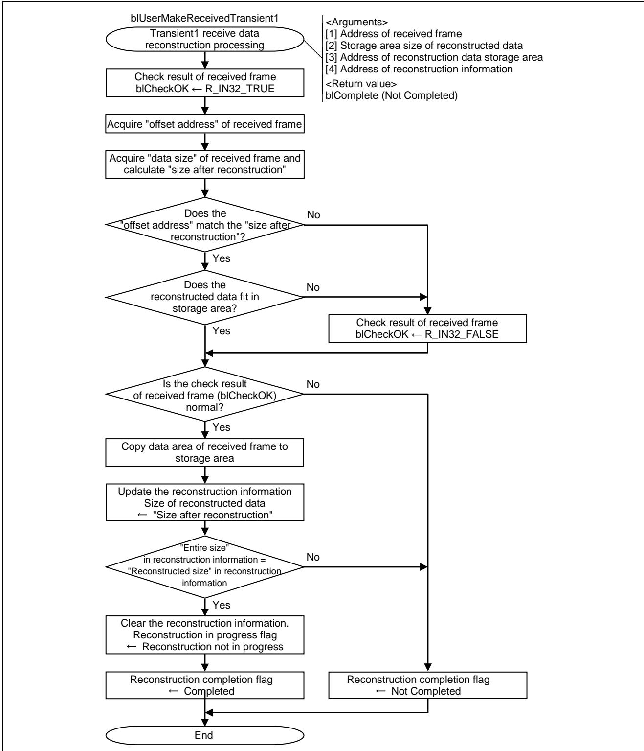
Figure 6.24 Flowchart for Transient1 Receive Data Reconstruction Processing
