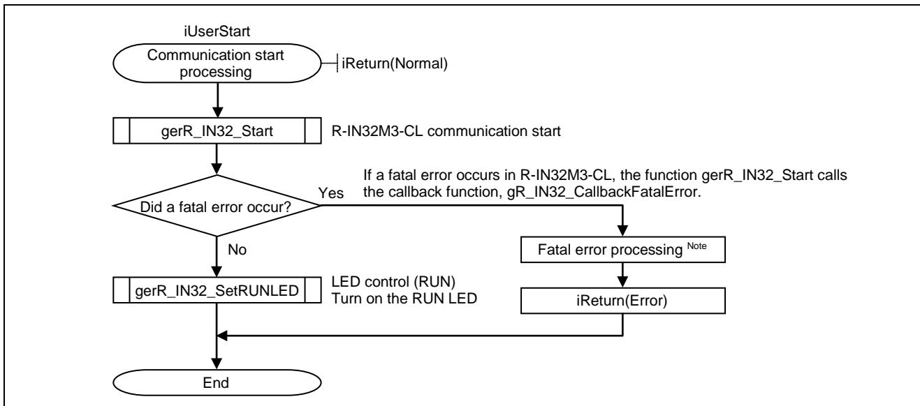
Figure 6.5 Flowchart for Communication Start Processing
