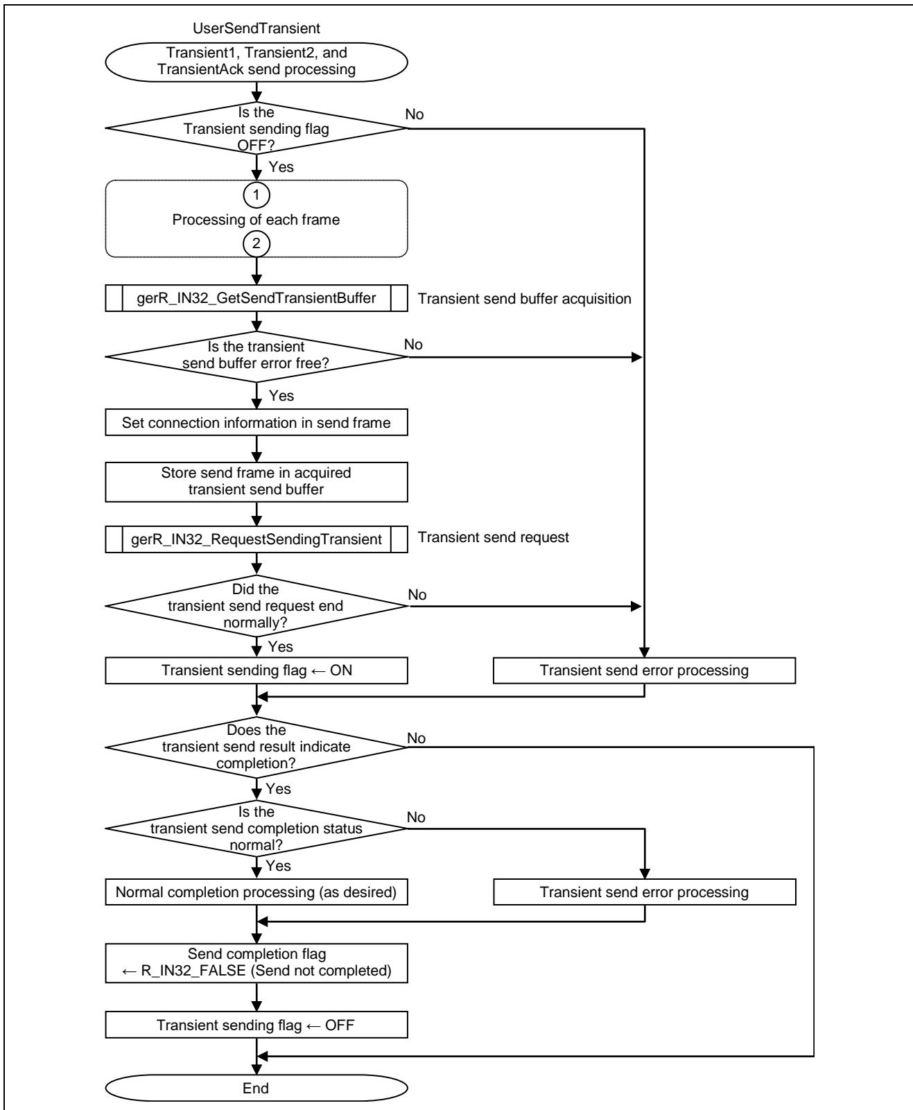
Figure 6.19 Flowchart for Transient1, Transient2, and TransientAck Send Processing (1/2)
