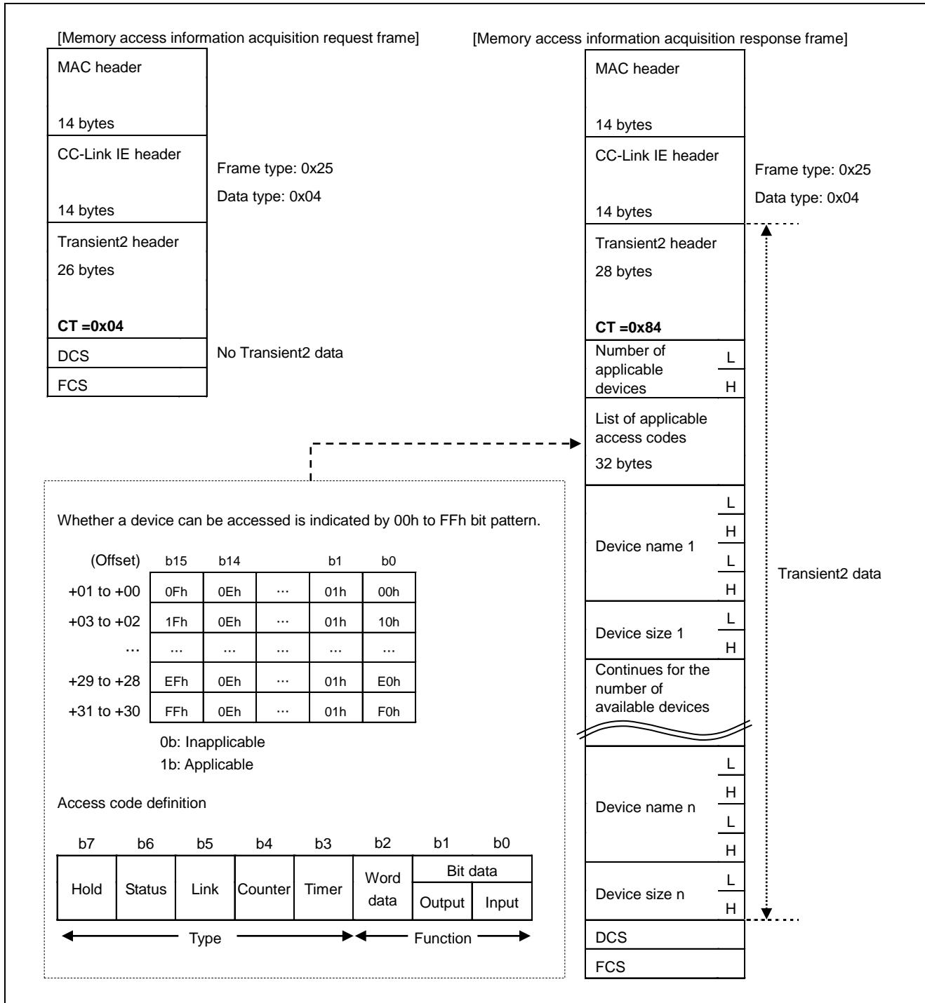
Figure 5.23 Overview of Memory Access Information Acquisition Frame Format
