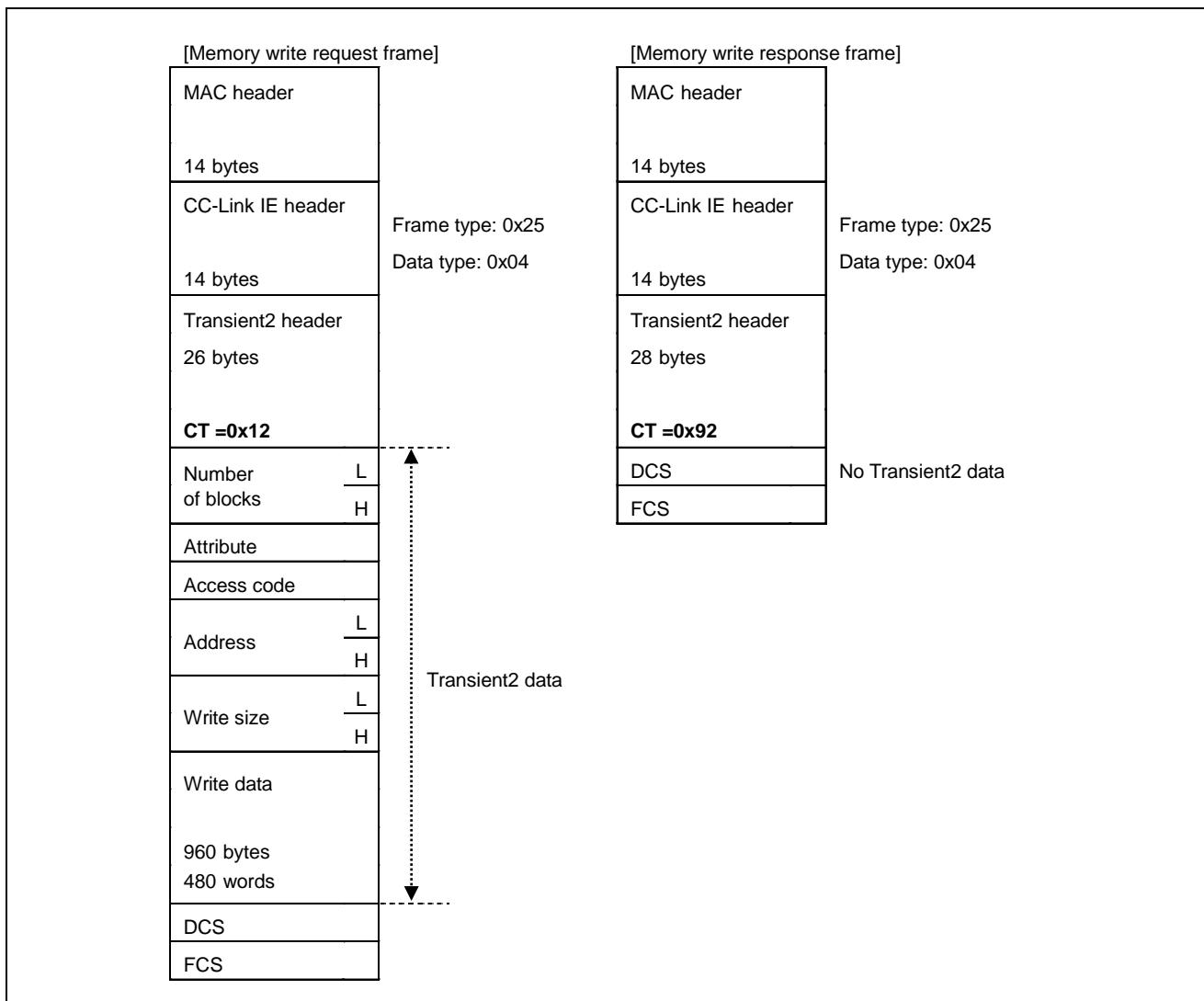
Figure 5.27 Overview of Memory Write Frame Format
