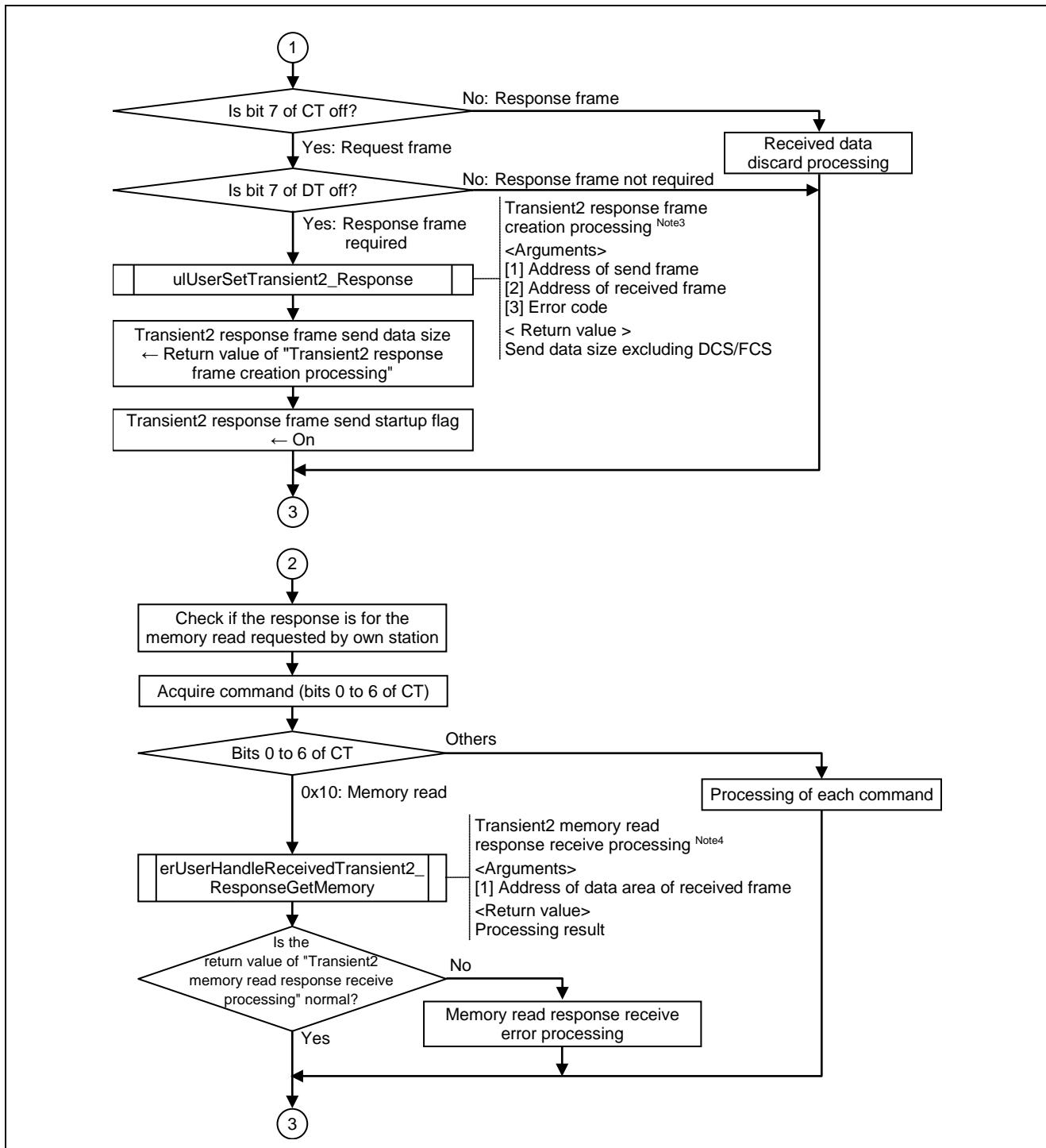
Figure 6.35 Flowchart for Transient2 Receive Data Processing (2/2)
