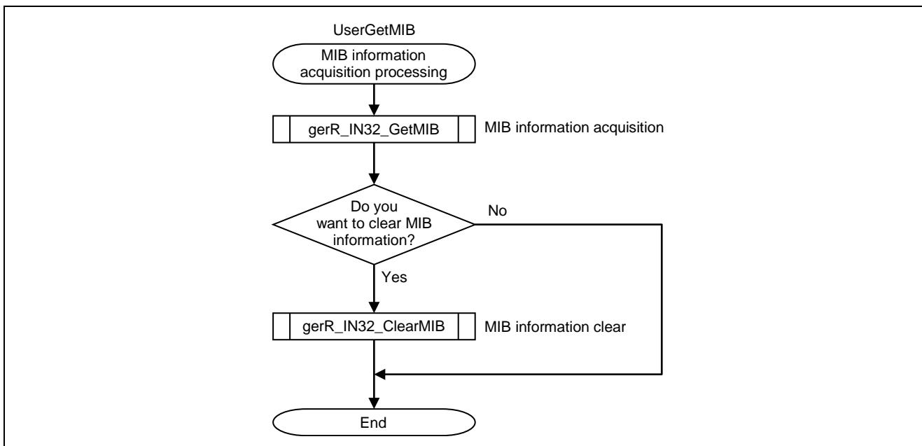
Figure 6.16 Flowchart for MIB Information Acquisition Processing
