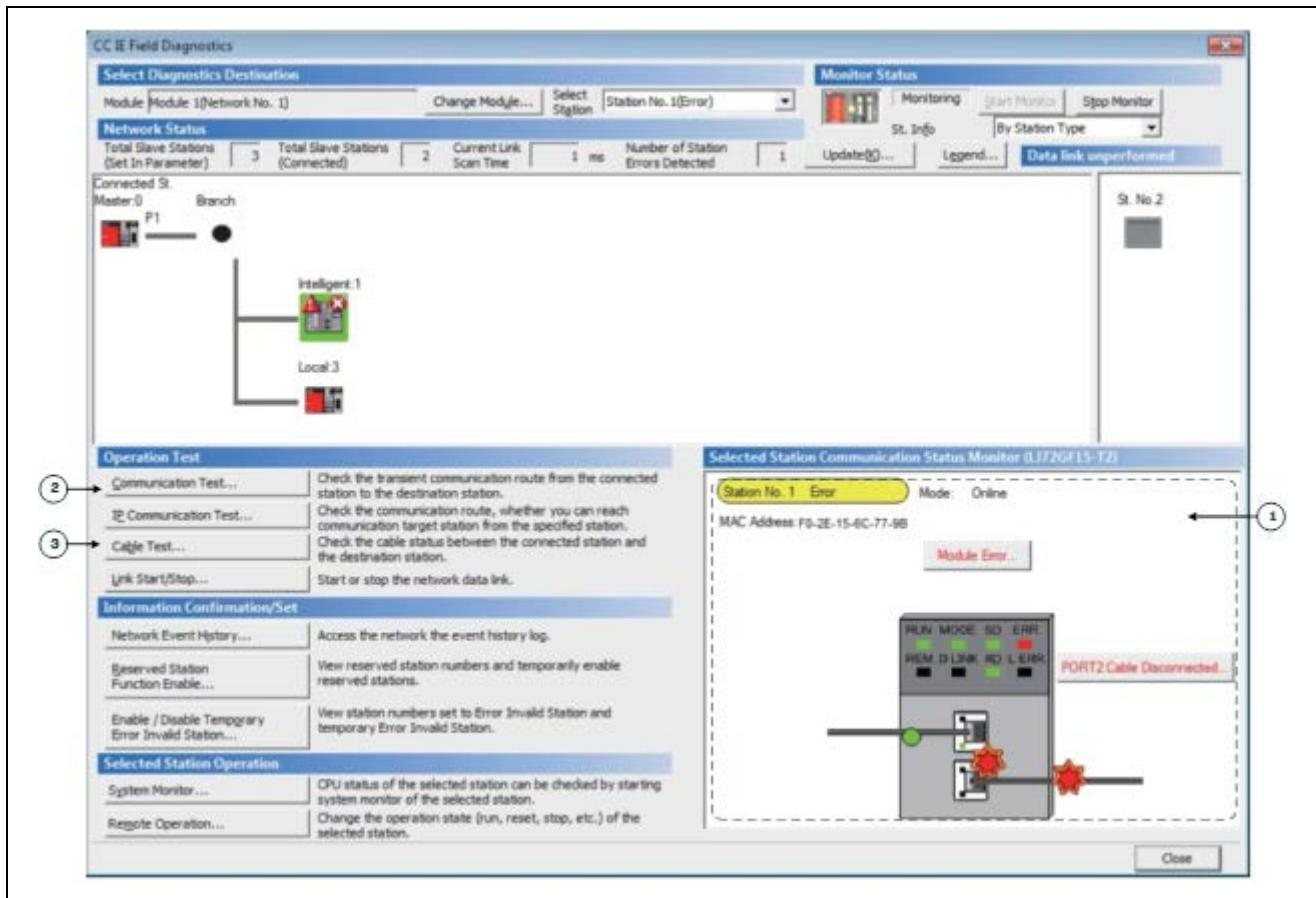
Figure 2.1 Diagnostic Window/Operation Locations (GX Works2)
