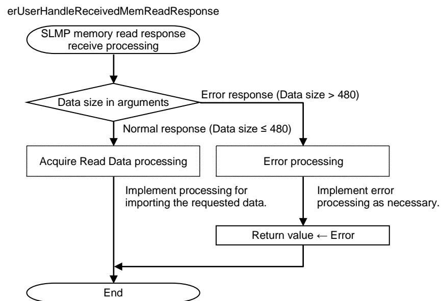
Figure 6.48 Flowchart for SLMP Memory Read Response Receive Processing
