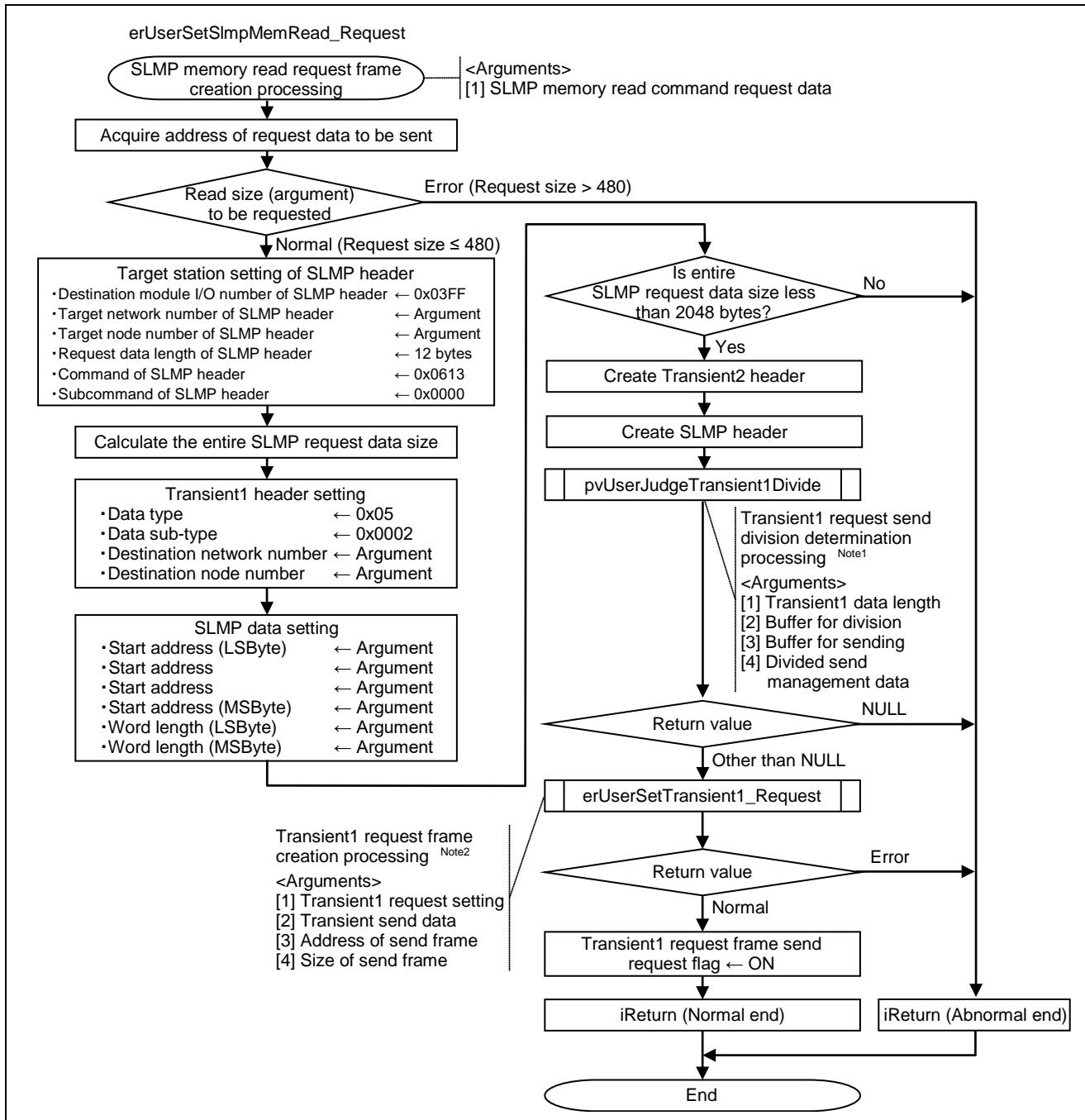
Figure 6.45 Flowchart for SLMP Memory Read Request Frame Creation Processing
