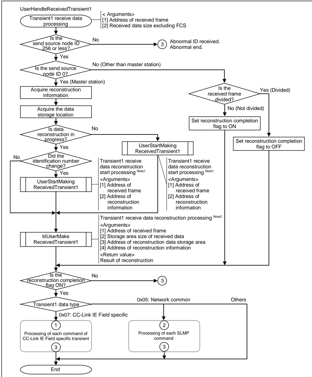
Figure 6.21 Flowchart for Transient1 Receive Data Processing (1/3)
