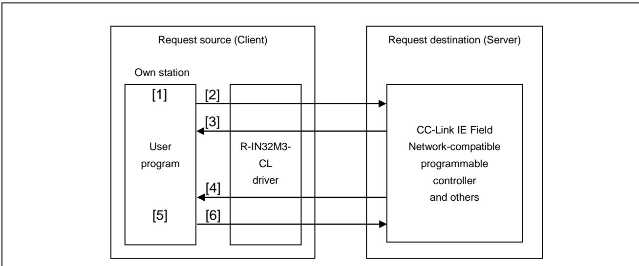
Figure 5.7 Transient2 Request Sending Procedure
