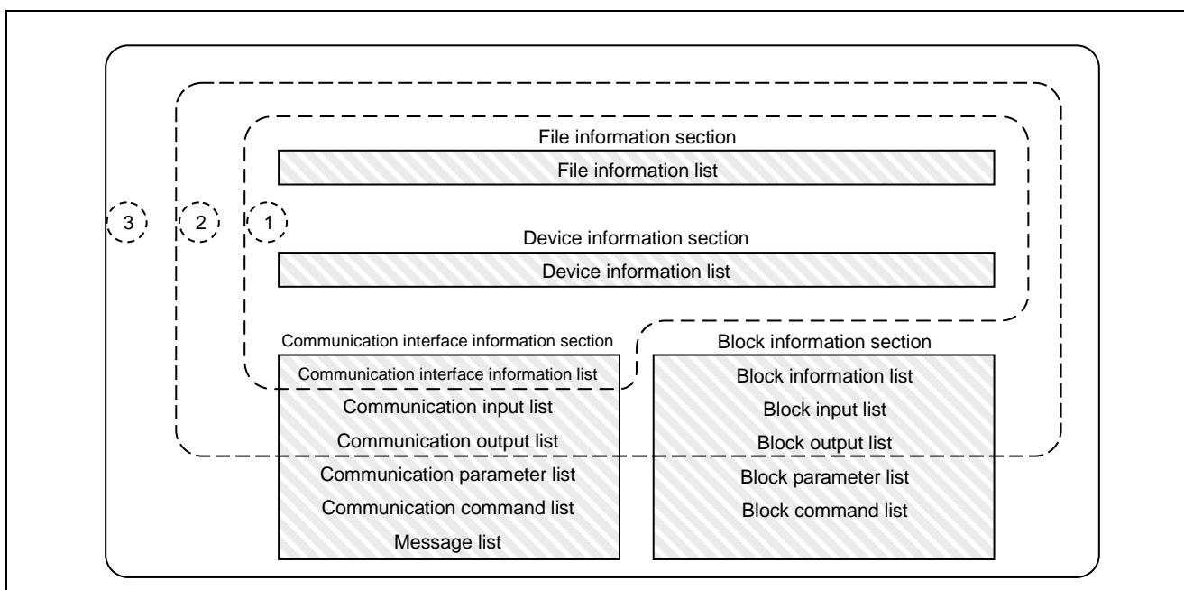
Figure 1.3 CSP+ File Section Configuration
