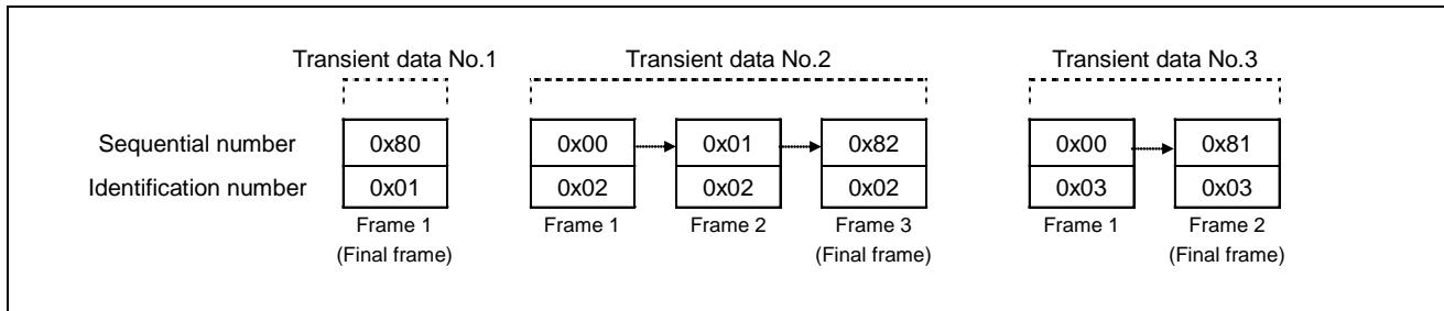
Figure 5.11 Transient1 Header: Relationship Between Sequential Number and Identification Number of Transient Data
