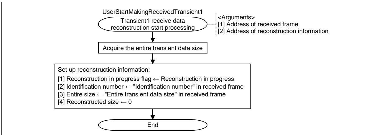
Figure 6.23 Flowchart for Transient1 Receive Data Reconstruction Start Processing
