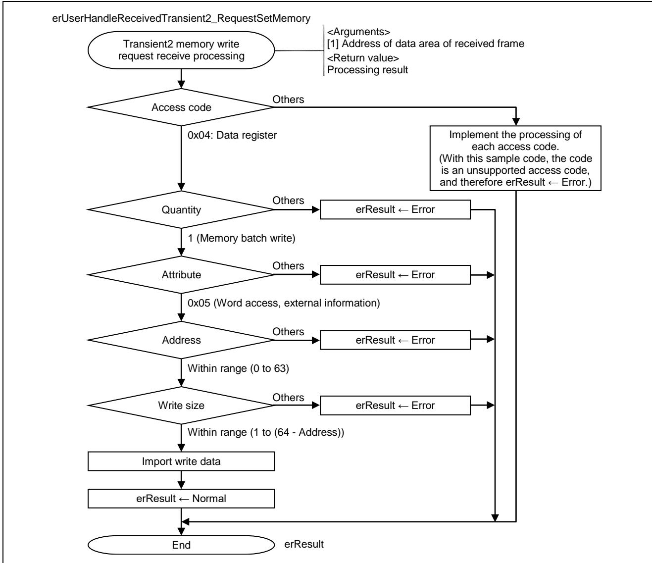
Figure 6.41 Flowchart for Transient2 Memory Write Request Receive Processing
