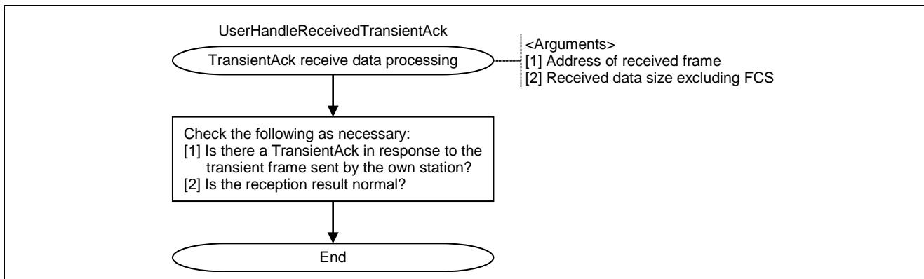
Figure 6.37 Flowchart for TransientAck Receive Data Processing
