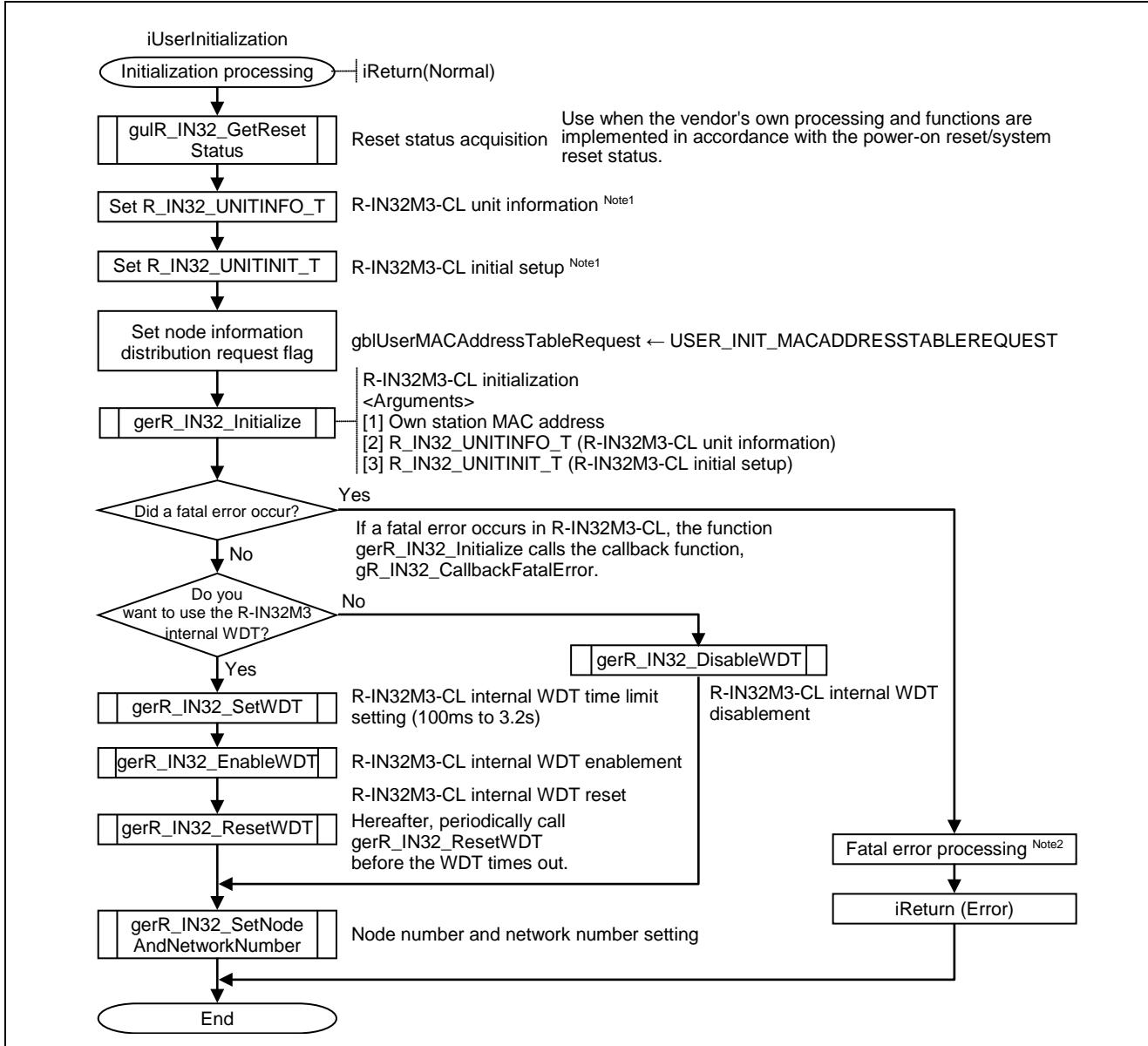
Figure 6.4 Flowchart for Initialization Processing
