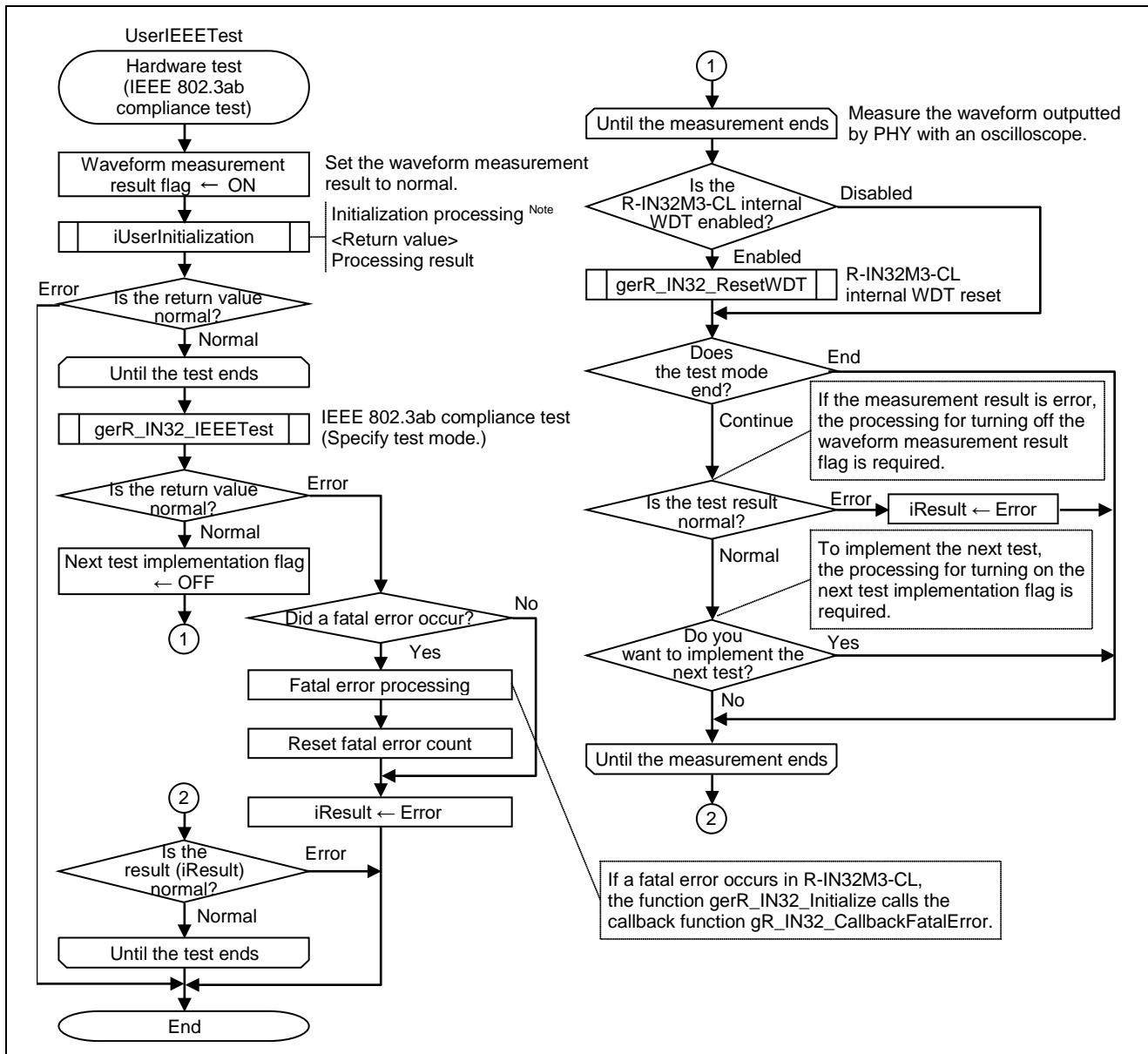
Figure 6.49 Flowchart for Hardware Test (IEEE 802.3ab Compliance Test)
