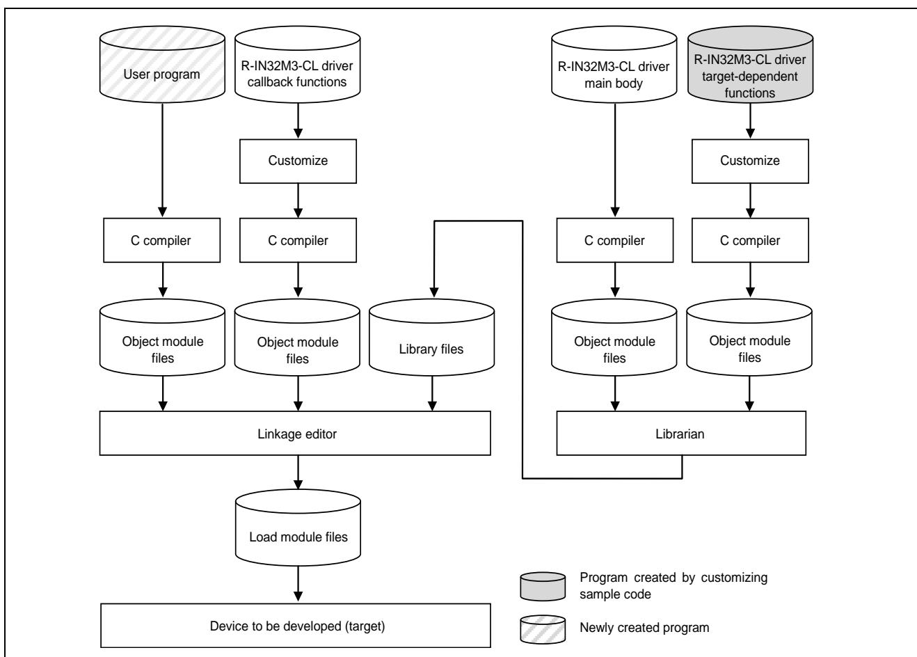
Figure 6.2 Firmware Development Procedure
