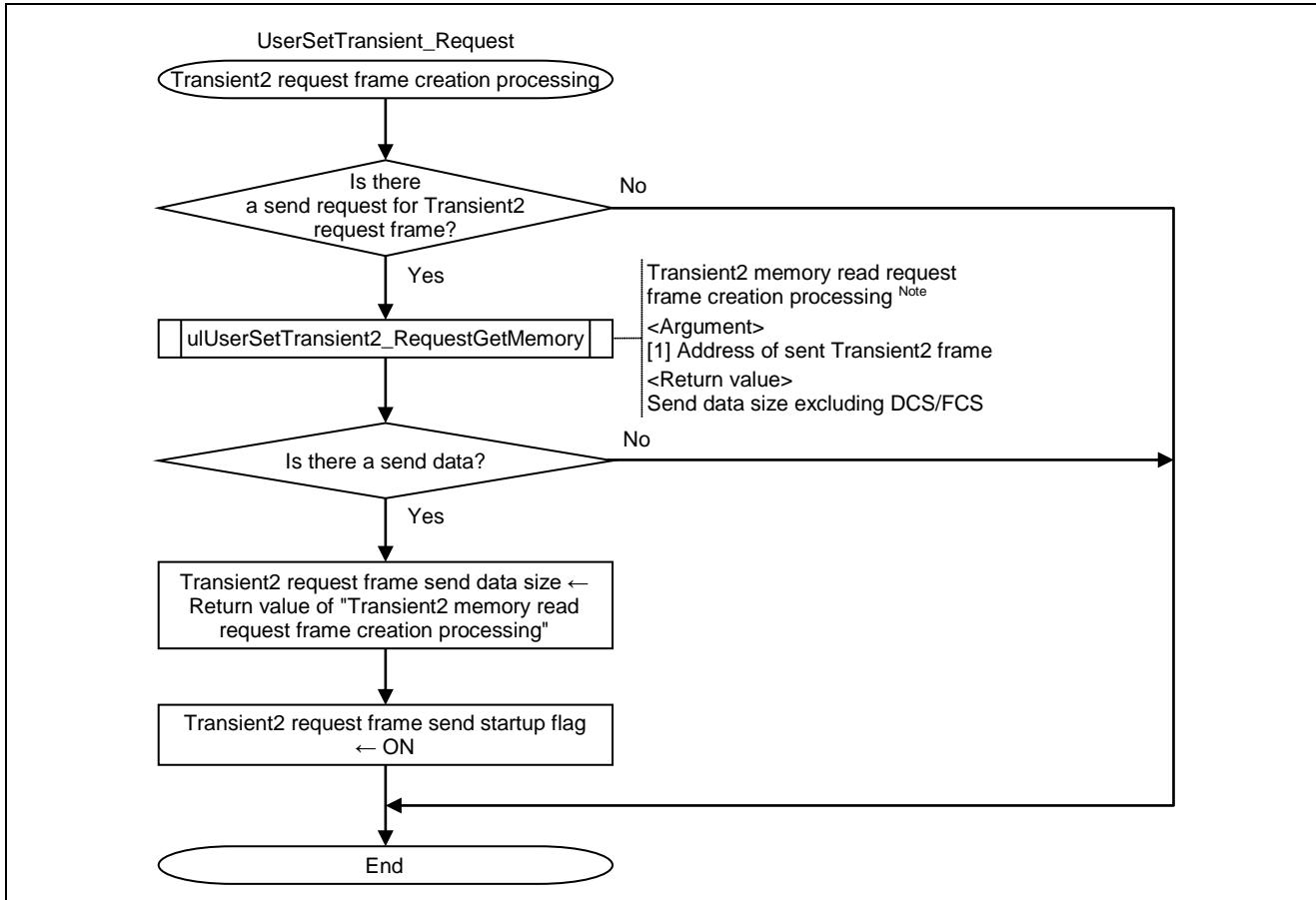
Figure 6.18 Flowchart for Transient2 Request Frame Creation Processing
