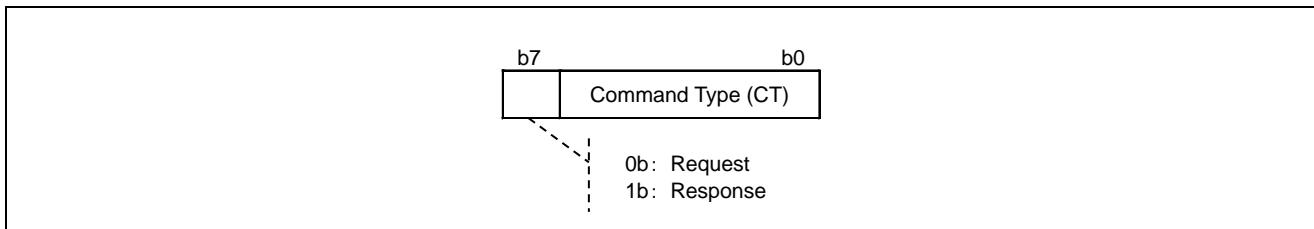
Figure 5.22 Data Structure of Command Type (CT)
