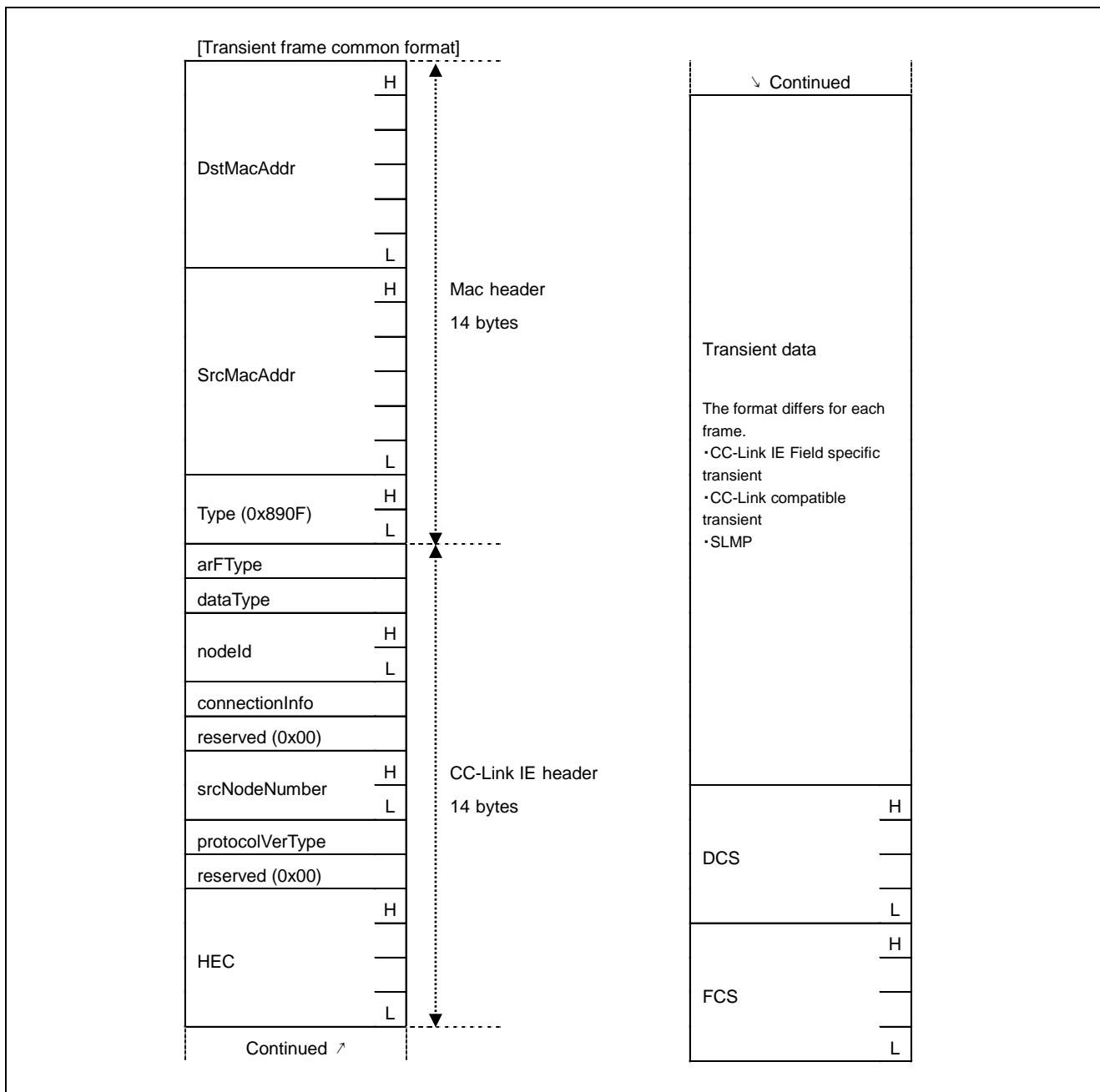
Figure 5.8 Transient Frame Common Format
