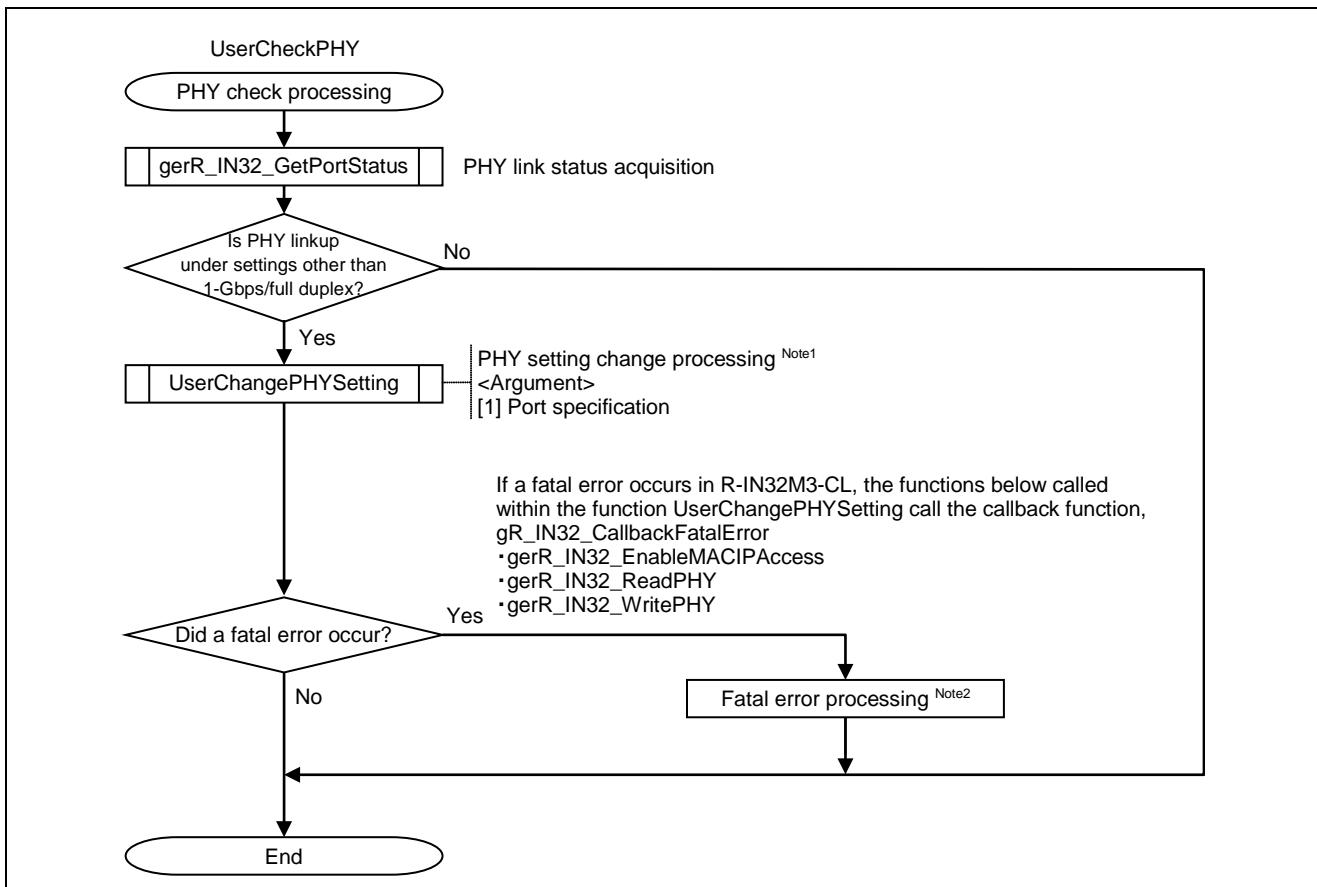
Figure 6.6 Flowchart for PHY Check Processing
