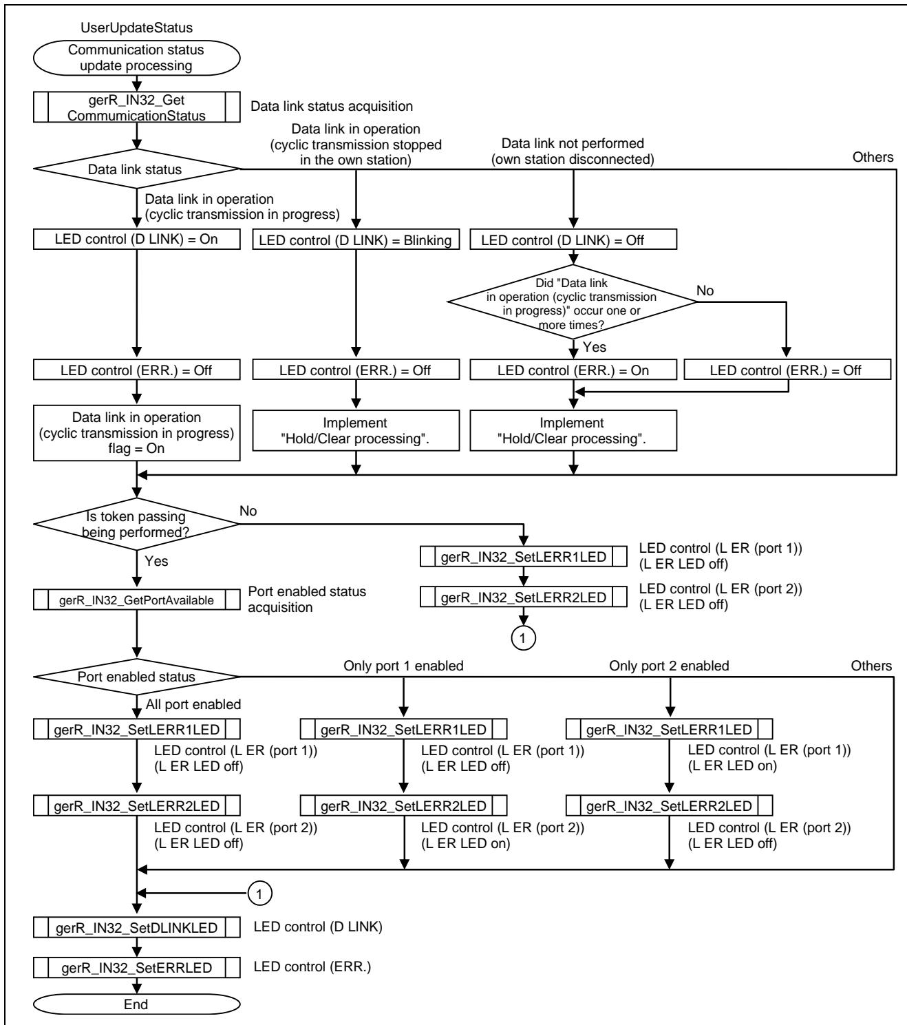
Figure 6.14 Flowchart for Communication Status Update Processing
