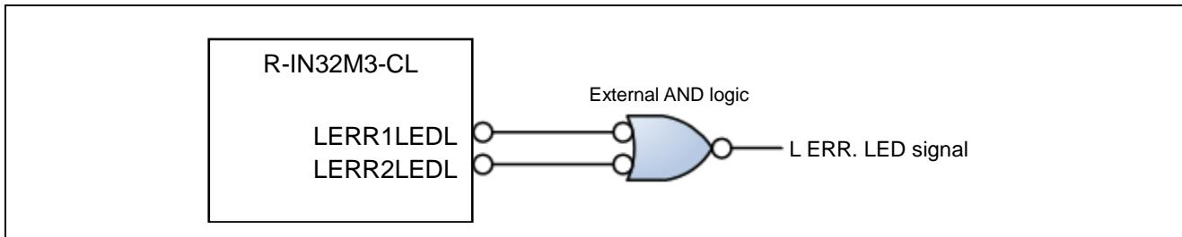
Figure 4.1 External AND Logic for Turning L ERR. On
