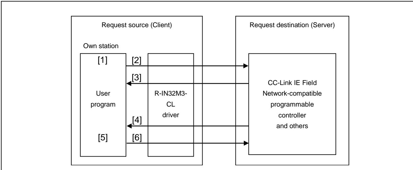
Figure 5.5 Transient1 Request Sending Procedure
