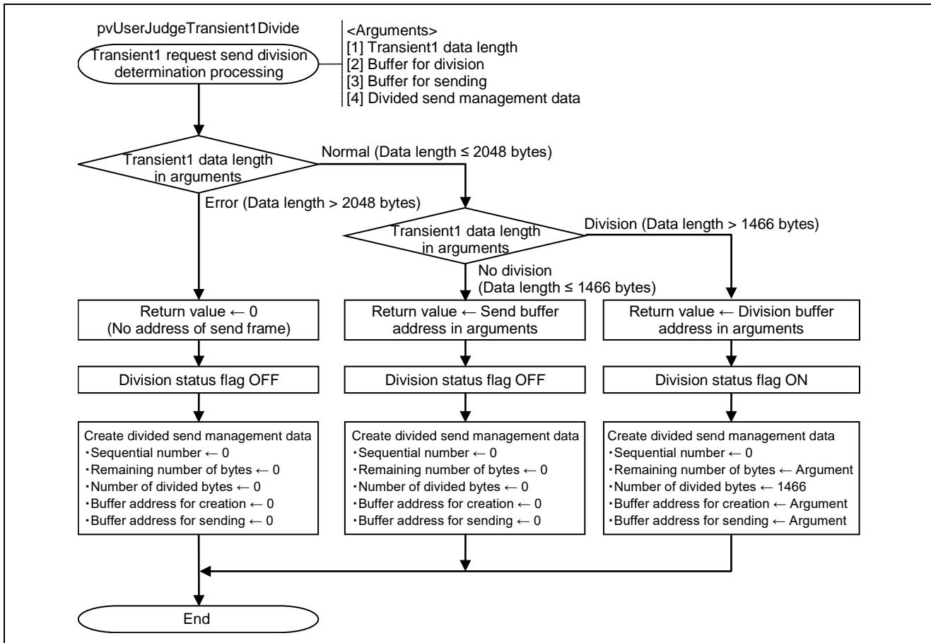
Figure 6.46 Flowchart for Transient1 Request Send Division Determination Processing
