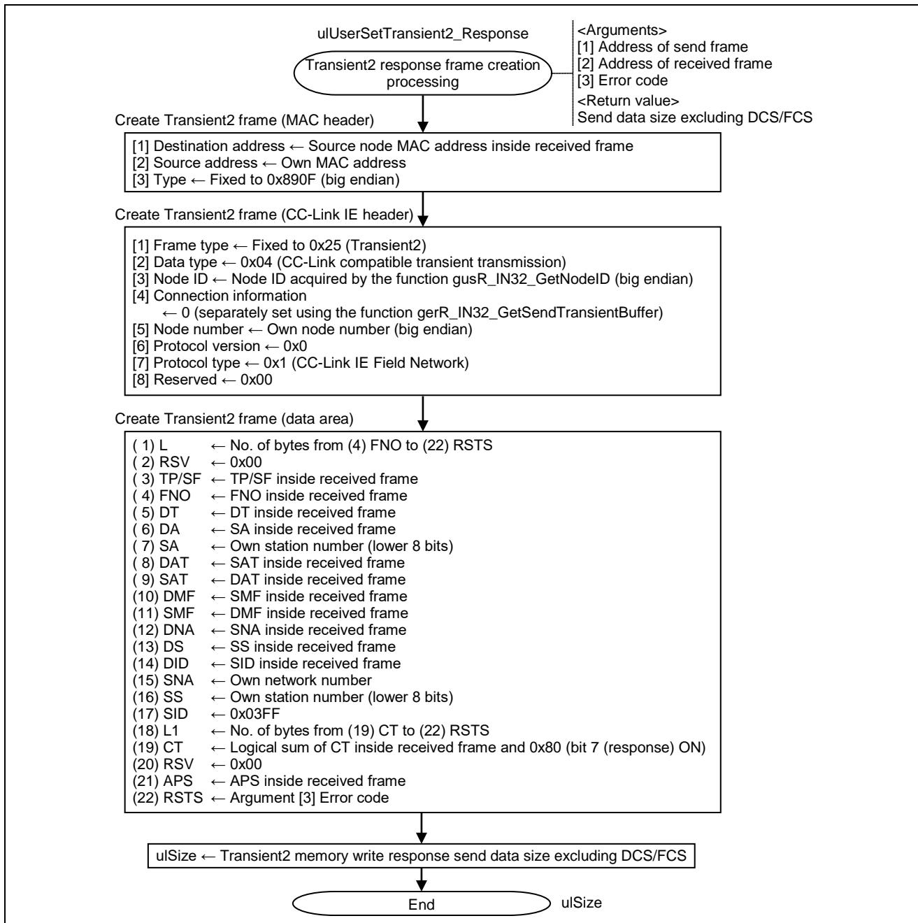
Figure 6.39 Flowchart for Transient2 Response Frame Creation Processing
