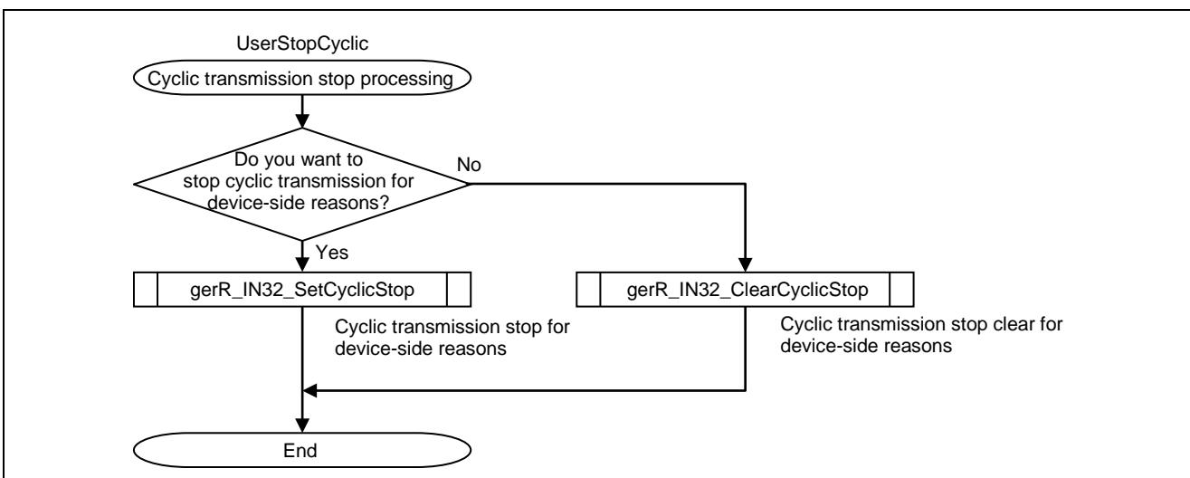
Figure 6.9 Flowchart for Cyclic Transmission Stop Processing
