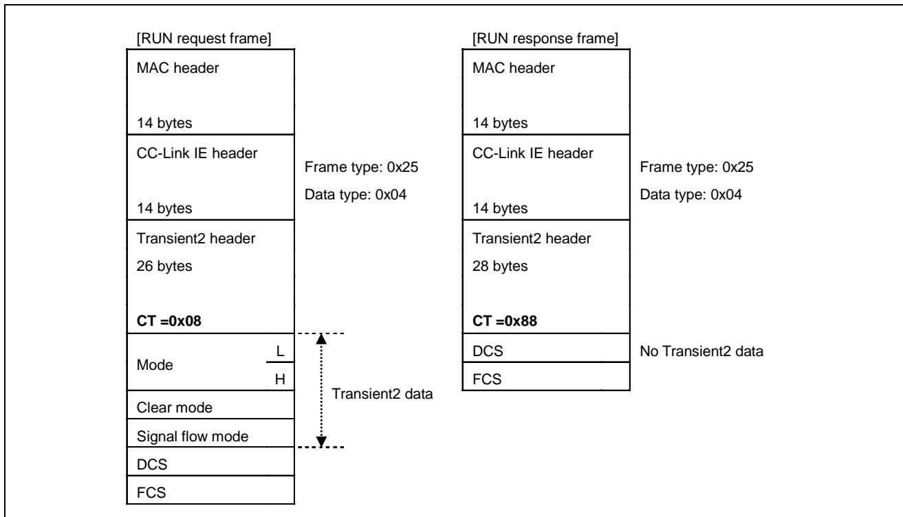
Figure 5.24 Overview of RUN Frame Format
