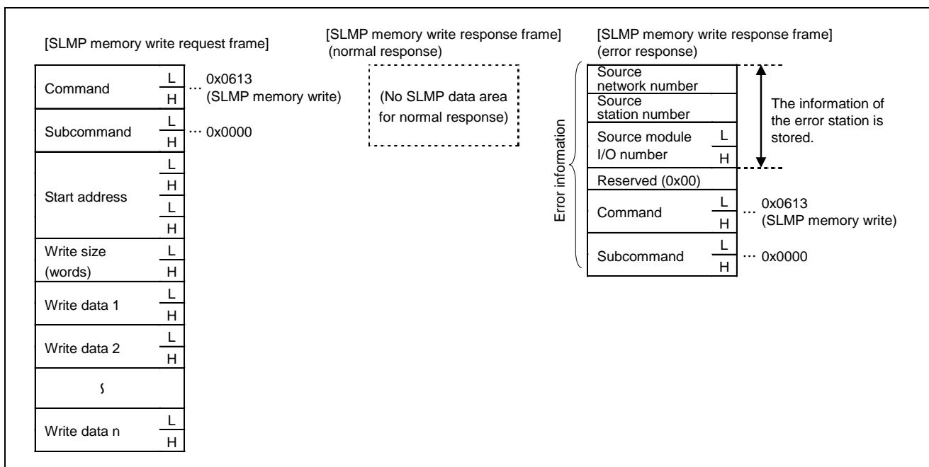
Figure 5.32 SLMP Memory Write Frame
