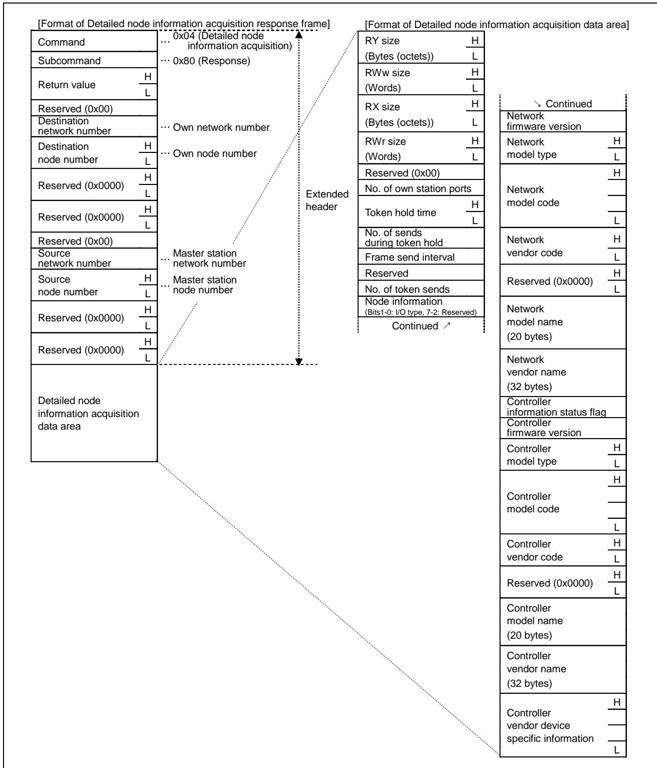
Figure 5.19 Transient1 Data Area: Detailed Node Information Acquisition Response
