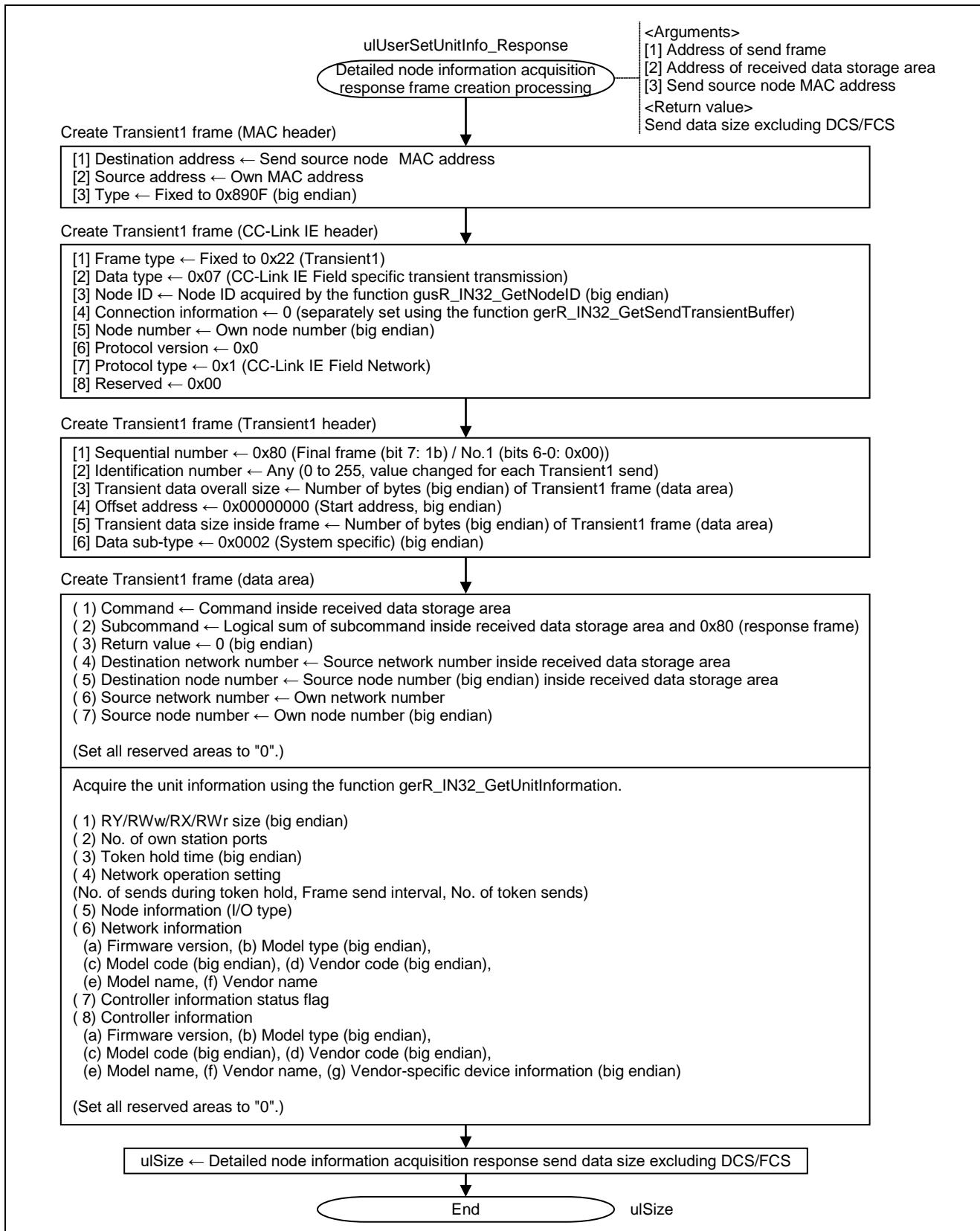
Figure 6.30 Flowchart for Detailed Node Information Acquisition Response Frame Creation Processing
