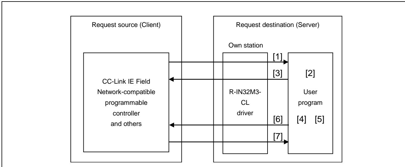
Figure 5.4 Transient1 Request Reception Procedure
