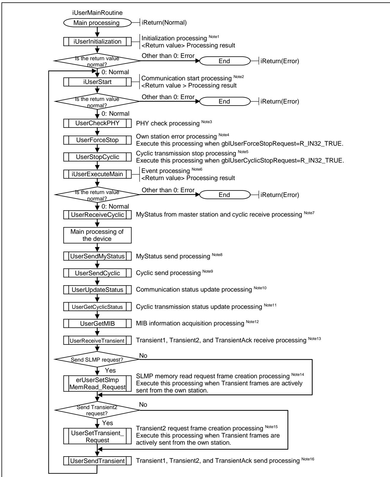
Figure 6.3 Flowchart for Main Processing
