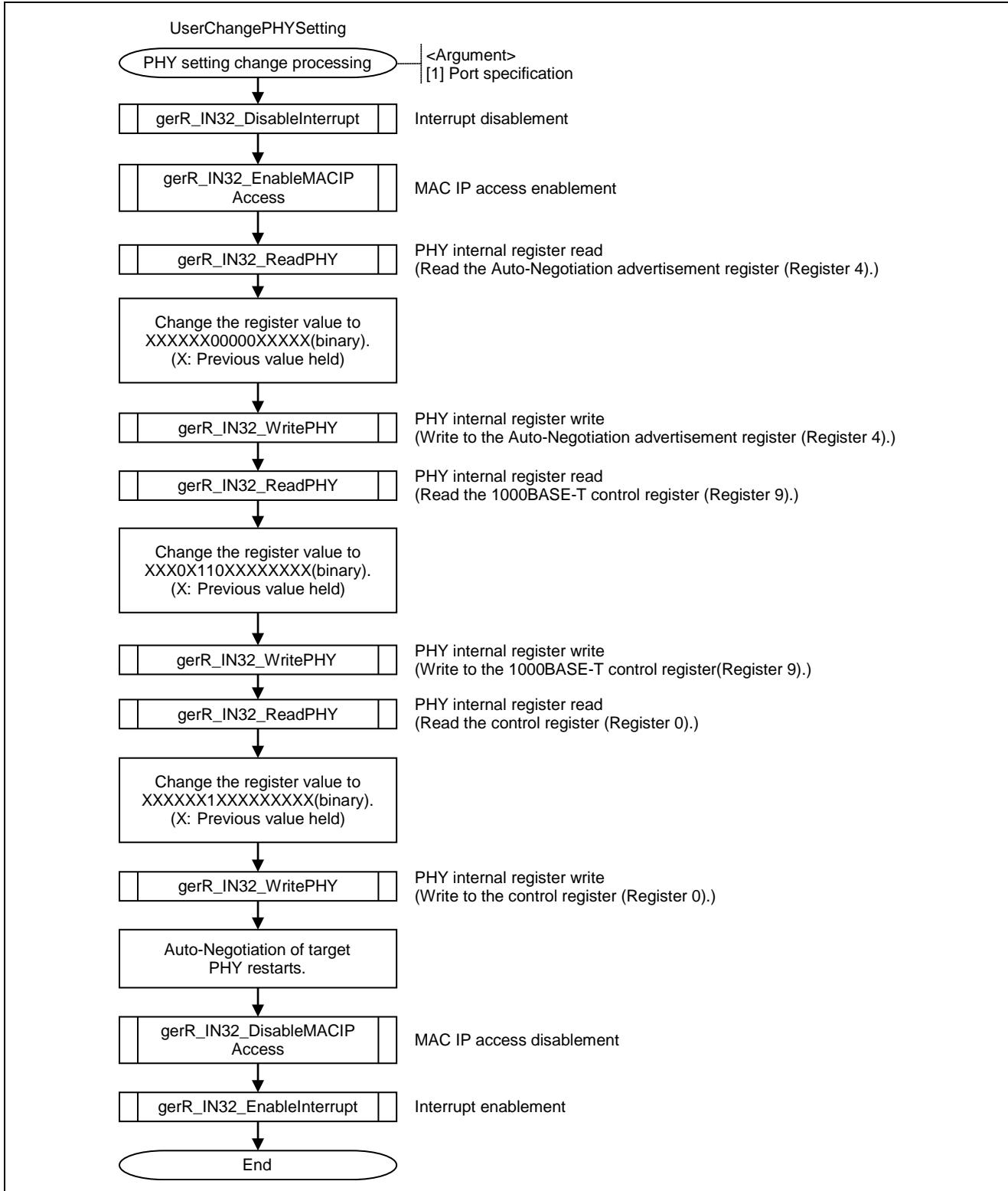
Figure 6.7 Flowchart for PHY Setting Change Processing
