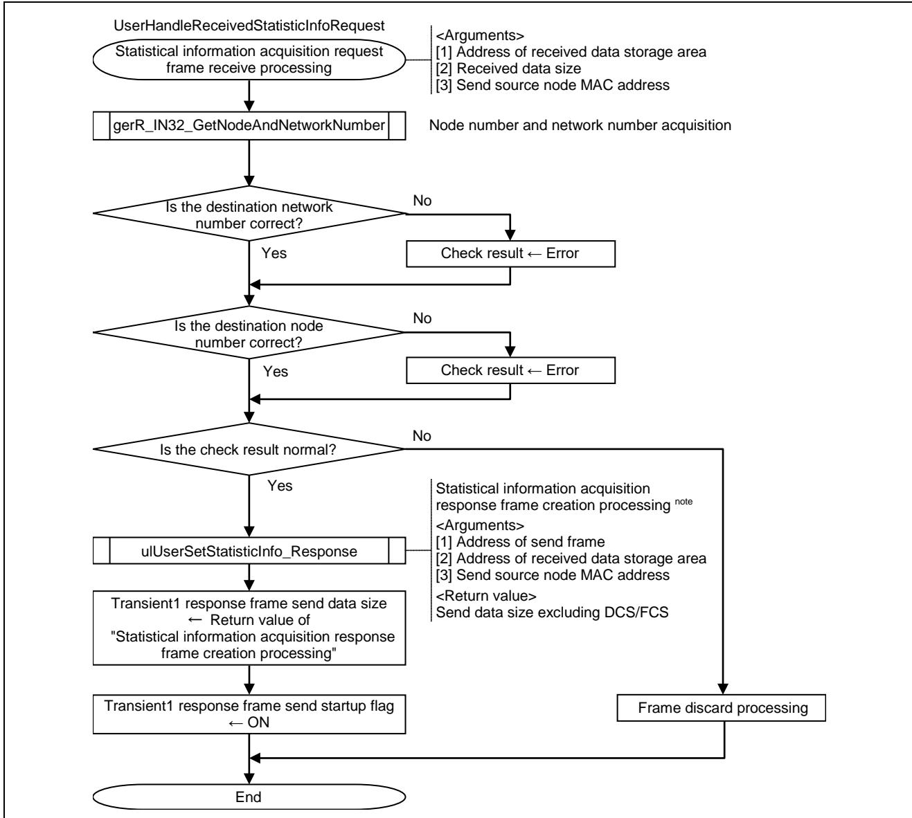
Figure 6.27 Flowchart for Statistical Information Acquisition Request Frame Receive Processing
