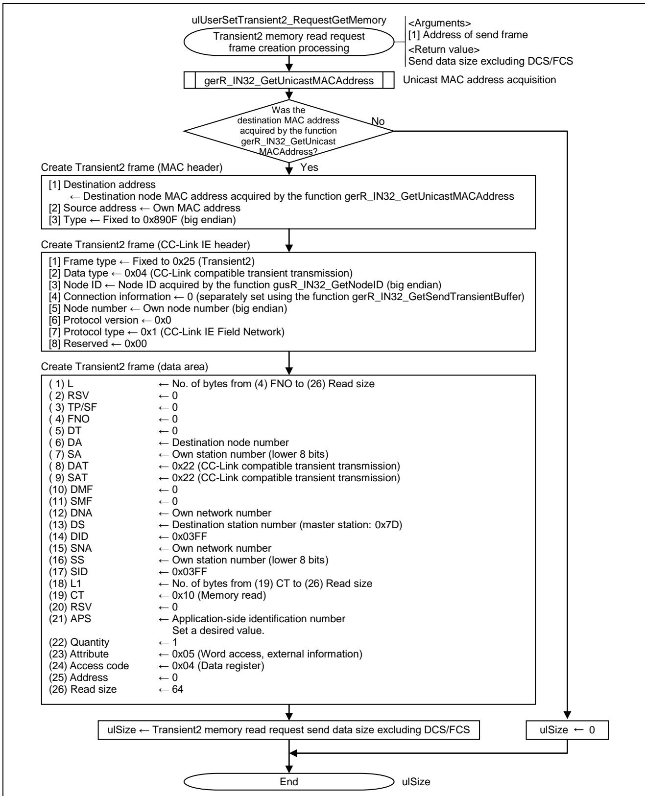
Figure 6.40 Flowchart for Transient2 Memory Read Request Frame Creation Processing
