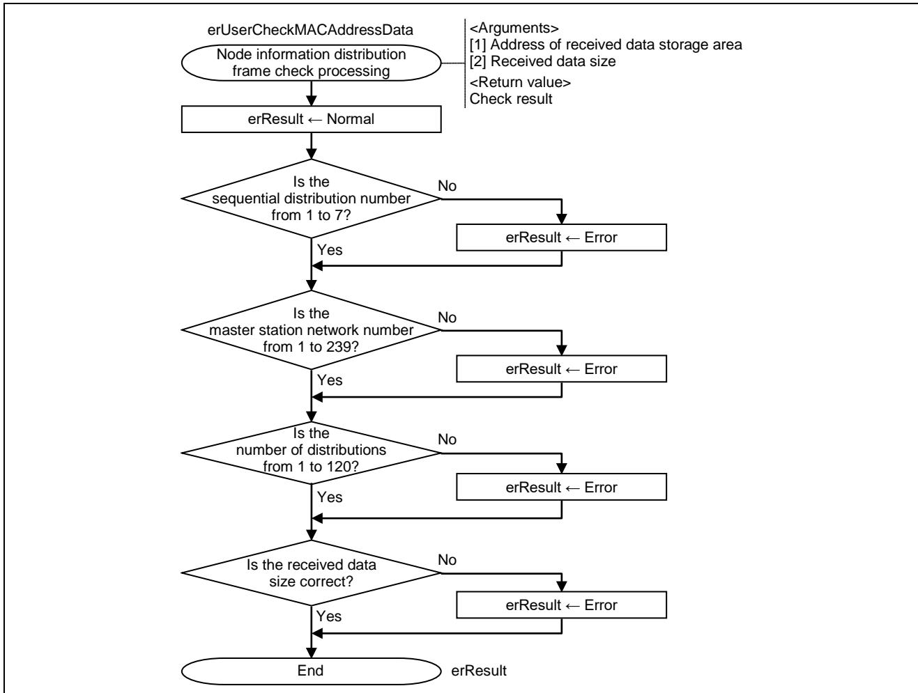
Figure 6.26 Flowchart for Node Information Distribution Frame Check Processing
