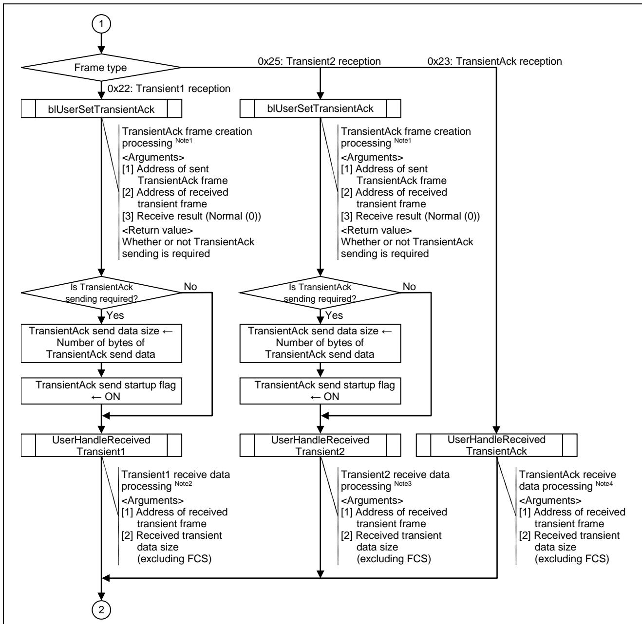
Figure 6.17 Flowchart for Transient1, Transient2, and TransientAck Receive Processing (2/2)
