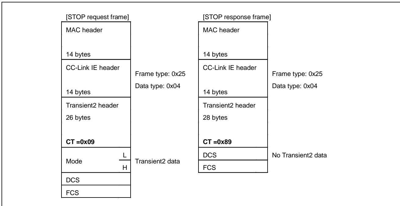
Figure 5.25 Overview of STOP Frame Format
