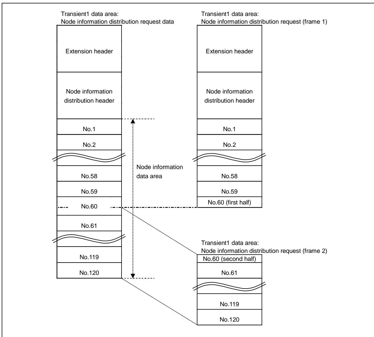
Figure 5.12 Transient1 Data Area: Divided Frames at Node Information Distribution Request
