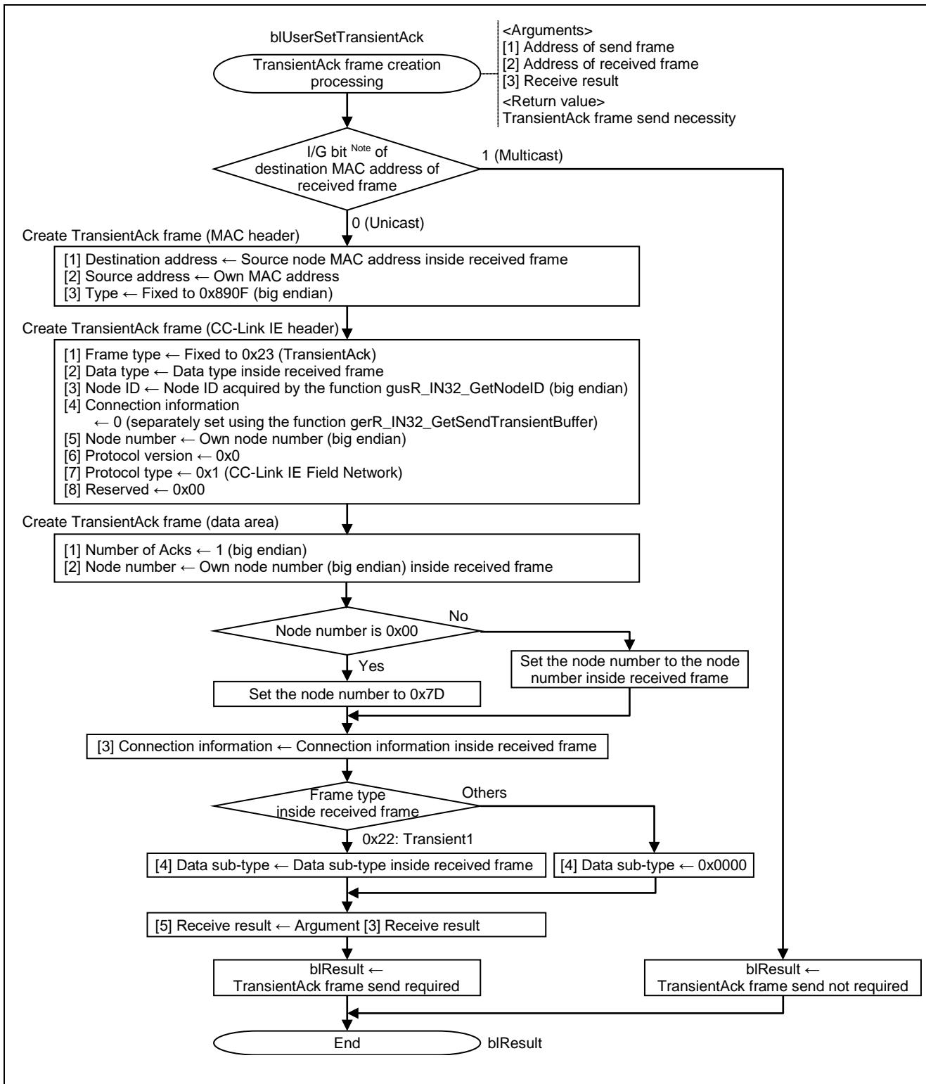
Figure 6.38 Flowchart for TransientAck Frame Creation Processing
