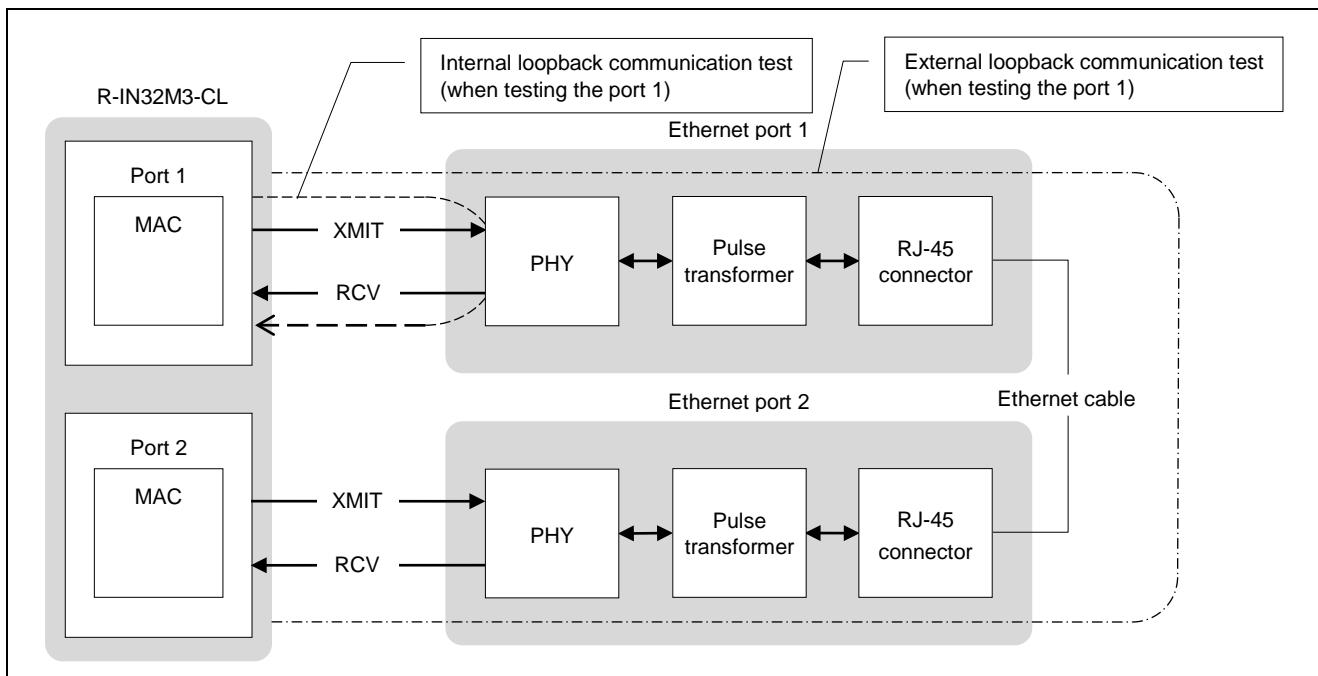
Figure 6.50 Port Schematic Diagram
