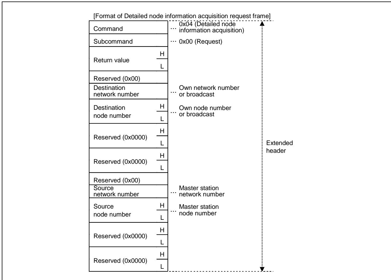
Figure 5.18 Transient1 Data Area: Detailed Node Information Acquisition Request
