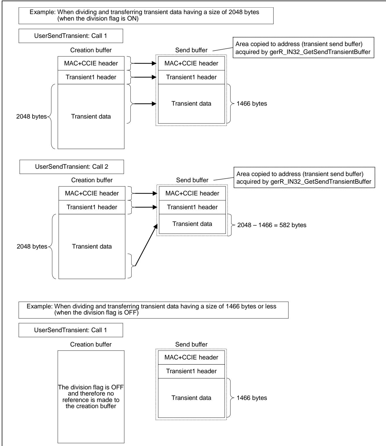
Figure 6.20 Transient Frame Divided Sending Procedure
