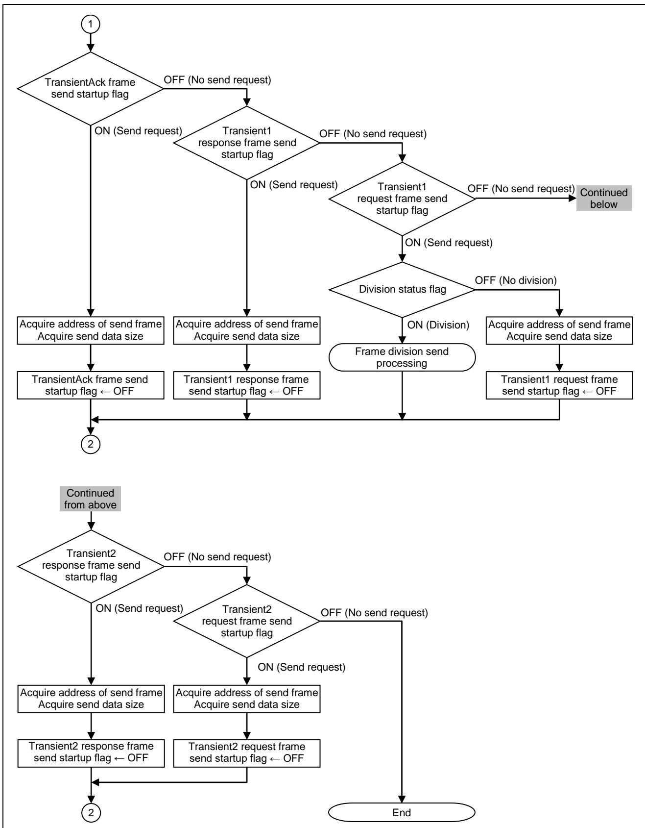
Figure 6.19 Flowchart for Transient1, Transient2, and TransientAck Send Processing (2/2)
