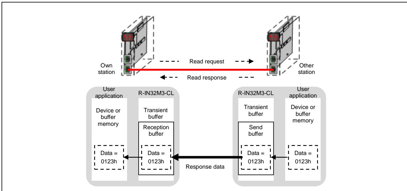
Figure 5.2 Flow of Transient Data
