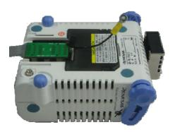
Figure 2-10. Connect the QB-RL78G1C to the probe
