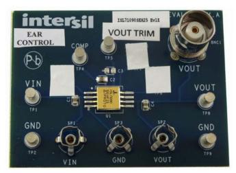
FIGURE 1. VOLTAGE REFERENCE EVALUATION BOARD
