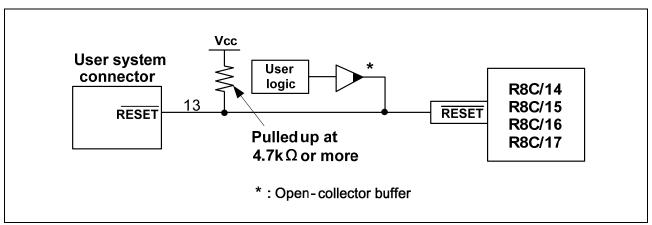
Figure 5.3 Example of a Reset Circuit
