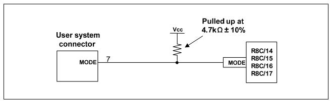
Figure 5.2 E8 Emulator and MODE Pin Connection
