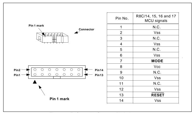
Figure 4.1 E8 Connecting Connector Pin Assignments
