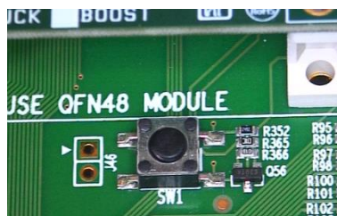
Figure 130: R365 (10 k \Omega ) Added Next to Reset Button
