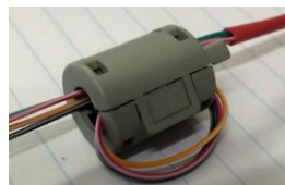
Figure 164: Example of Twisted Pair Cable with 4 Pairs and Ferrite
