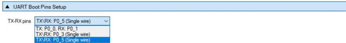
Figure 45: UART Boot Pins Setup - DA14531
