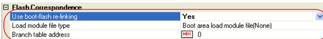
Select [Boot area load module file(None)] (default) in the [Load module file type] property. Specify the start address of the branch table (address in the flash area) in the [Branch table address] property. The range that can be specified for the value is 0 to FFFFFFFF (hexadecimal number). "0" is set by default.
