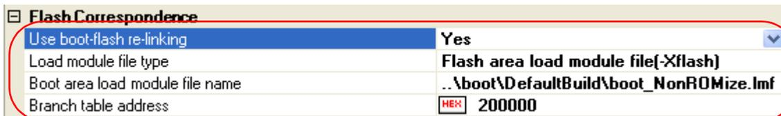
Select [Flash area load module file(-Xflash)] in the [Load module file type] property. The [Boot area load module file name] property will be displayed.
