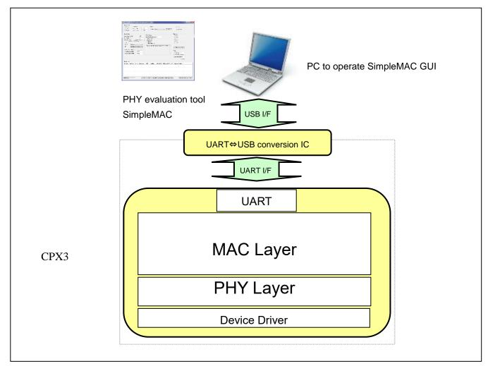
Figure 1-5 PLC evaluation software configuration
