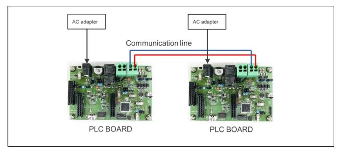
Figure 2-3 Condition 2: PC board connection example of DC power supply from the AC adaptor (1)
