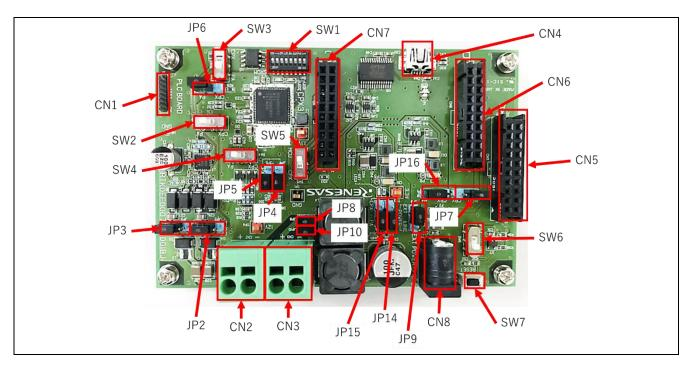
Figure 1-8 PLC board connector, JP, and SW
