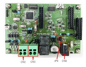
Figure 2-1 Board power supply setting parts
