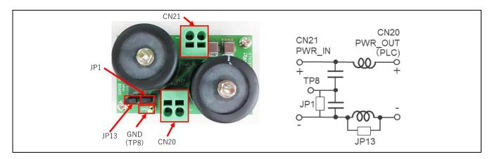
Figure 3-3 Connector, JP and TP for Power filter board
