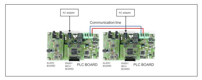
Figure 2-6 Condition 5 : PLC board + RX651 MCU board + Audio board
