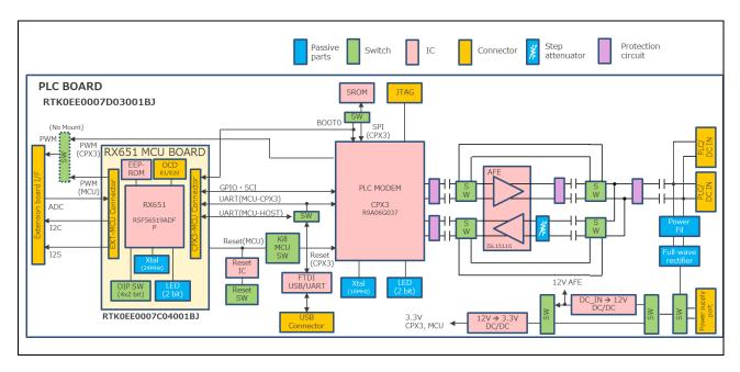
Figure 1-6 PLC board, RX651 MCU board Function block diagram
