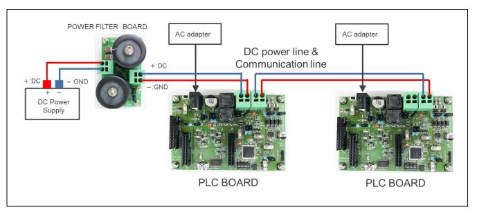
Figure 2-4 Condition 3: PC board connection example of DC power supply from the AC adaptor (2)
