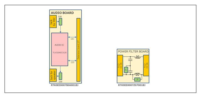
Figure 1-7 Audio board, Power Filter Board Function block diagram
