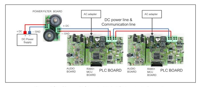
Figure 2-5 Condition 4: PLC board + RX651 MCU board + Audio board
