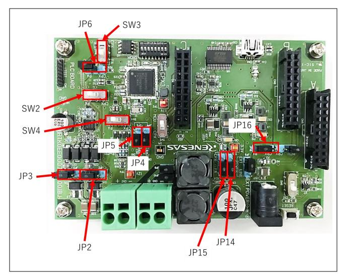
Figure 3-1 Parts used for switching drive system
