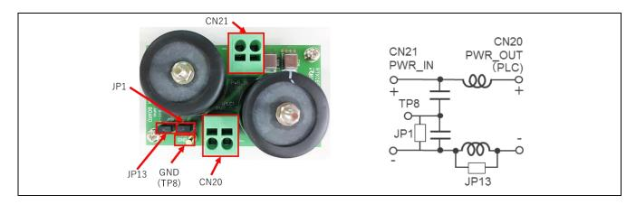
Figure 1-11 Power filter board connector, JP and TP
