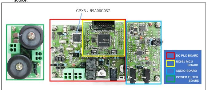
Figure 1-1 Configuration of PLC board, RX651 MCU board, Audio board and Power filter board
