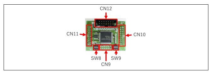
Figure 1-9 RX651 MCU board connector and SW
