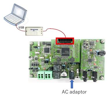
Figure 3-2 E1emulator - RX651 MCU board connection configuration
