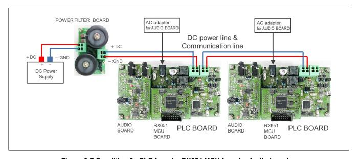
Figure 2-7 Condition 6 : PLC board + RX651 MCU board + Audio board
