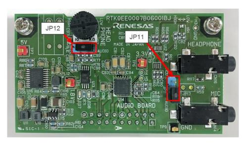
Figure 2-9 Audio board setting parts
