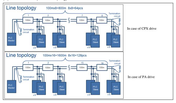
Figure 1-2 Connection example of Line topology
