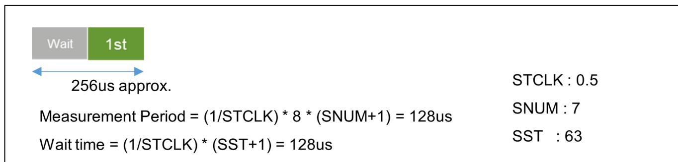
Figure 153: Current Measurement Period
