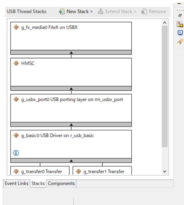
Figure 165: FileX on USBX Stack
