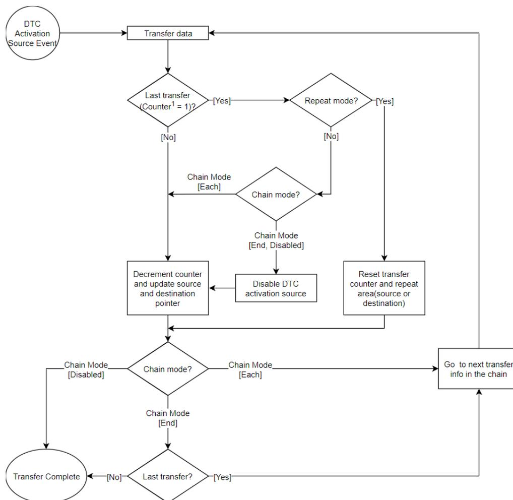
1. Counter refers to transfer\_info\_t.length in normal and repeat mode and transfer\_info\_t.num\_blocks in block mode.
