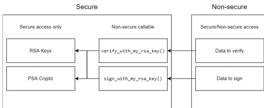
Figure 219: PSA Crypto Non-secure callable example
