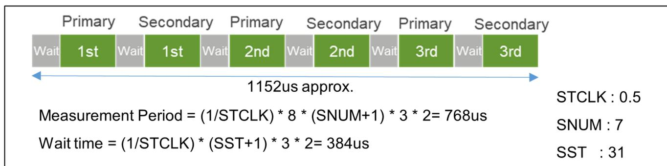
Figure 152: Mutual-capacitance Measurement Period
