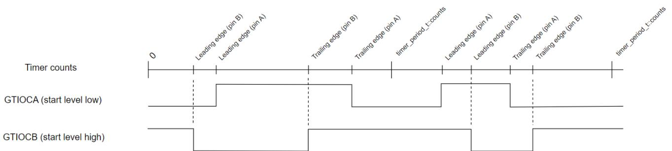
Figure 227: GPT One-Shot Pulse Output (without dead time)
