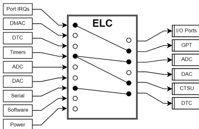
Figure 224: Event Link Controller Conceptual Diagram
