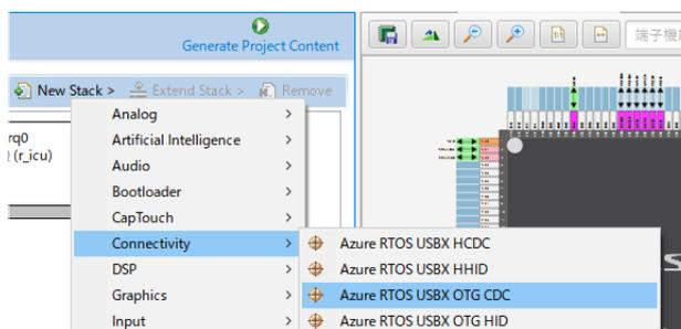
Figure 166: Select USB Device Class for OTG
