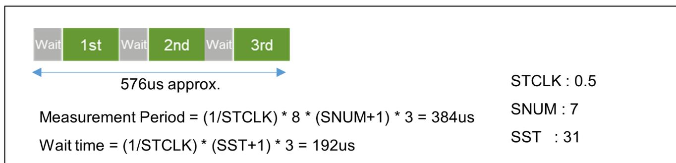
Figure 151: Self-capacitance Measurement Period (CTS2)
