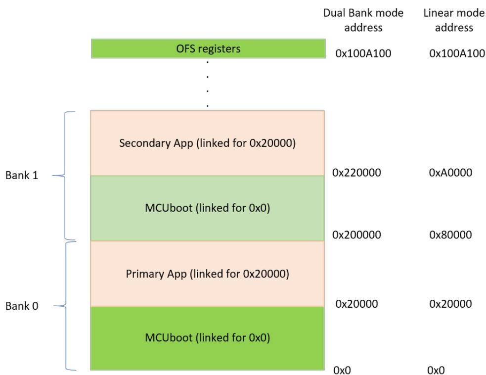
Figure 142: MCUboot Dual Bank layout for 1 MB Memory
