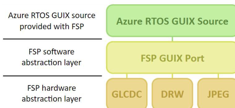
Figure 201: Azure RTOS GUIX Port Block Diagram
