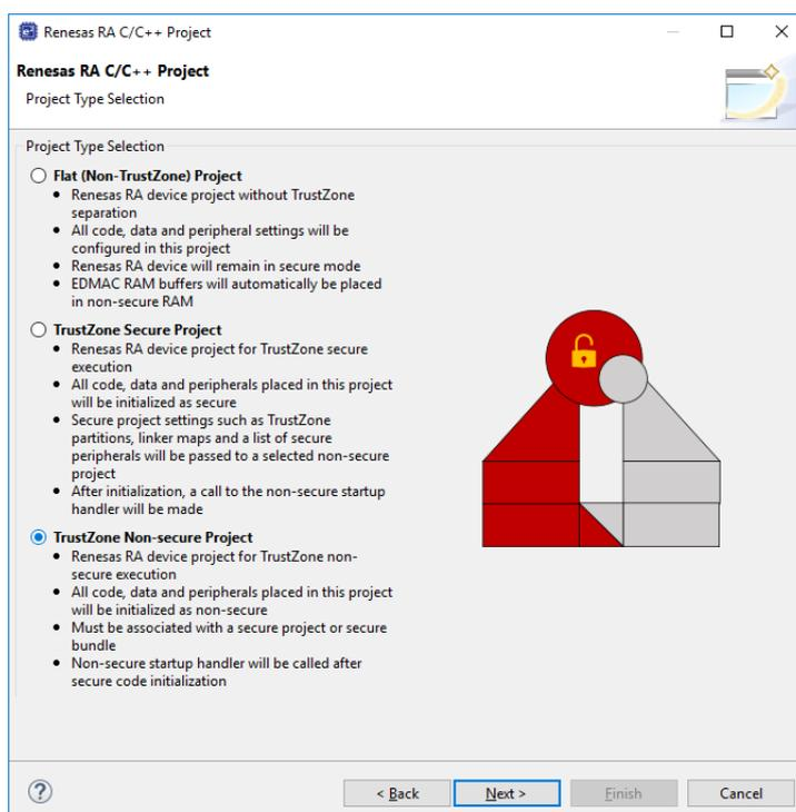
Figure 102: Non-Secure Project (following Arm notation as red)
