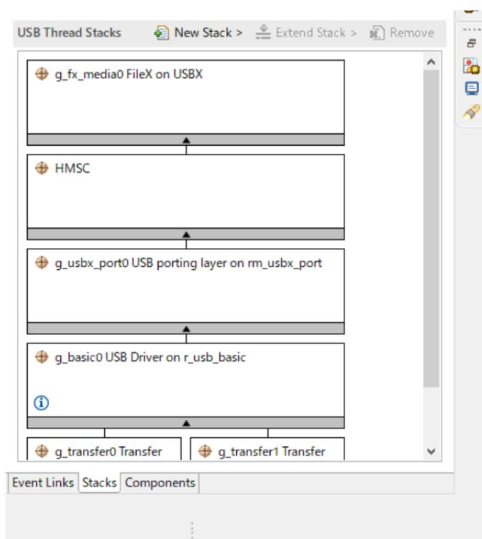
Figure 216: FileX on USBX Stack
