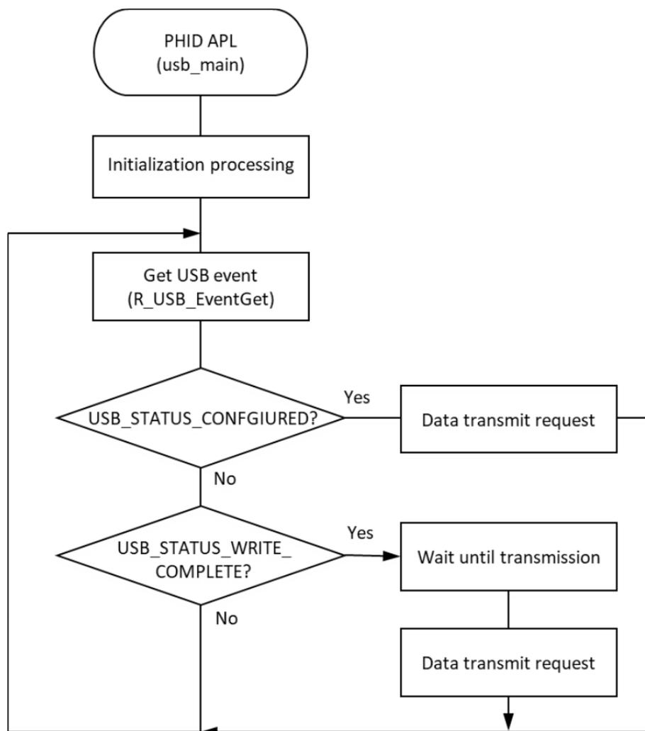
Figure 193: Main Loop processing for non-RTOS example
