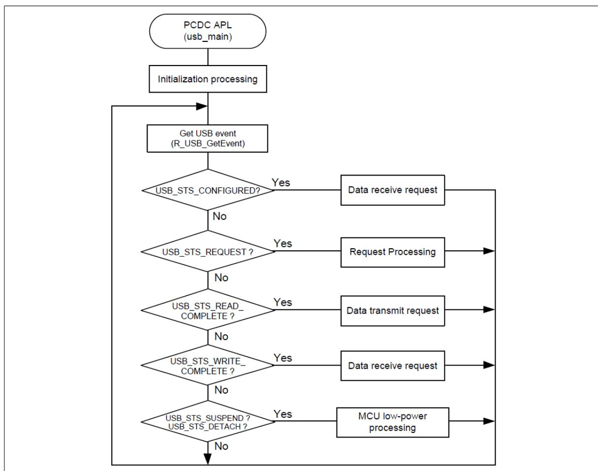
Figure 191: Main Loop processing (Echo mode)
