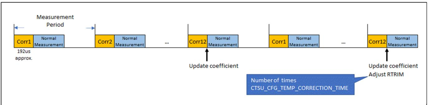
Figure 158: Temperature Correction Measurement Timing Chart
