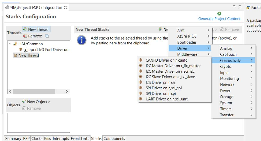
Figure 31: Adding Modules and Drivers to a thread
