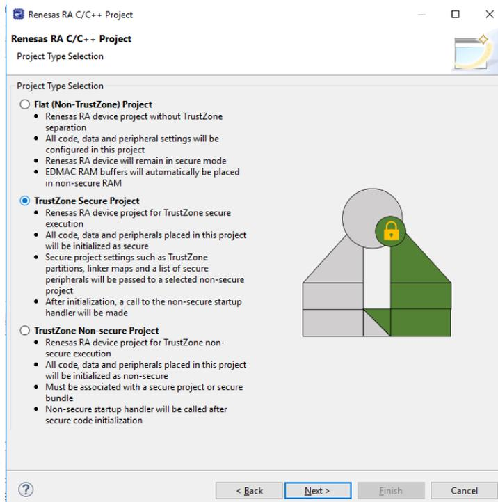
Figure 101: Secure Project (following Arm notation as green)
