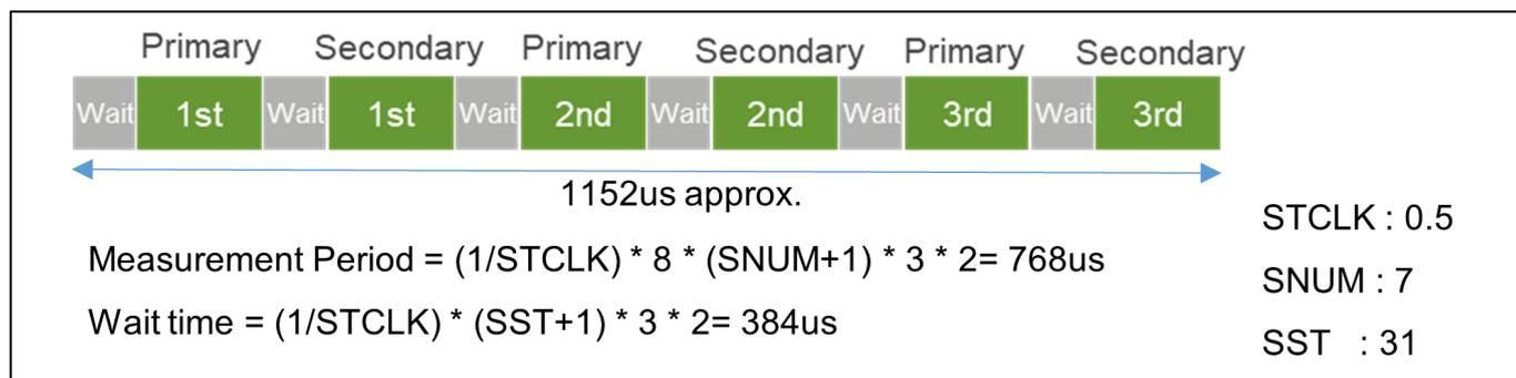
Figure 156: Mutual-capacitance Measurement Period
