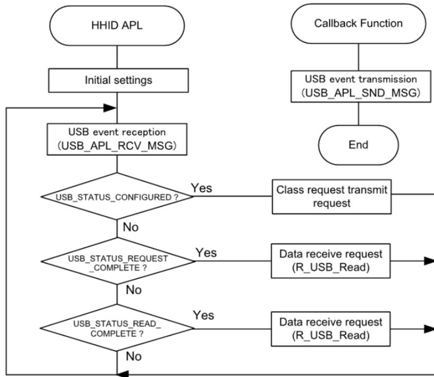
Figure 183: Main Loop (Normal mode)
