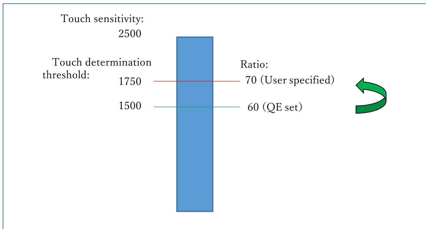
Figure 206: Example of changing the threshold ratio
