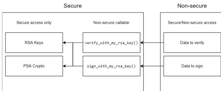
Figure 204: PSA Crypto Non-secure callable example
