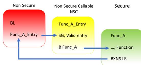
Figure 99: Calling from Non-Secure to Secure Functions
