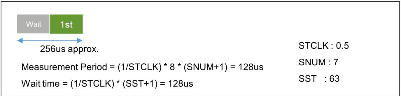
Figure 157: Current Measurement Period
