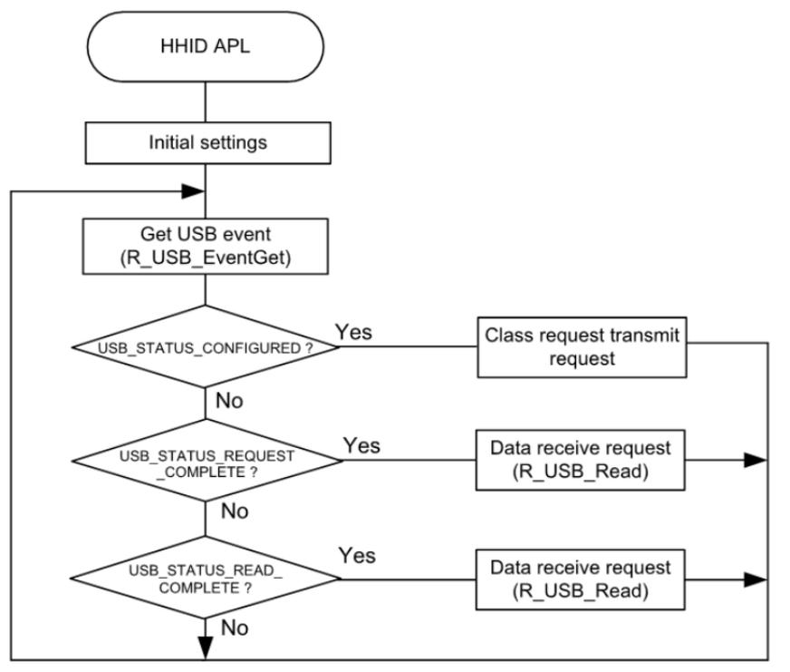
Figure 182: Main Loop (Normal mode)
