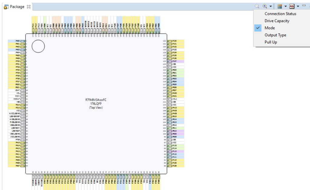
Figure 21: e2 studio Pin configurator package view
