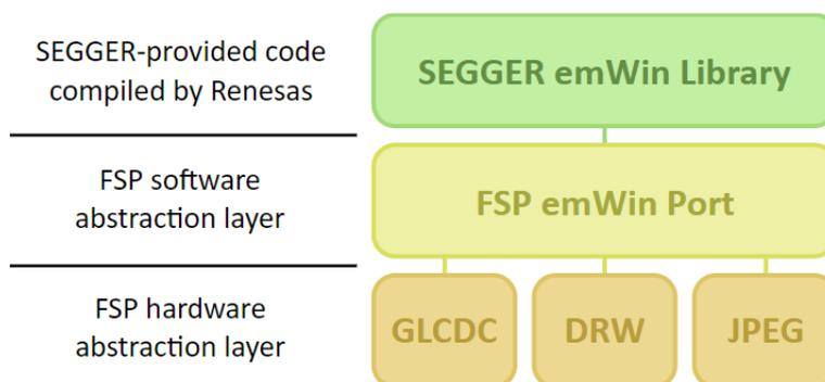
Figure 200: SEGGER emWin FSP Port Block Diagram
