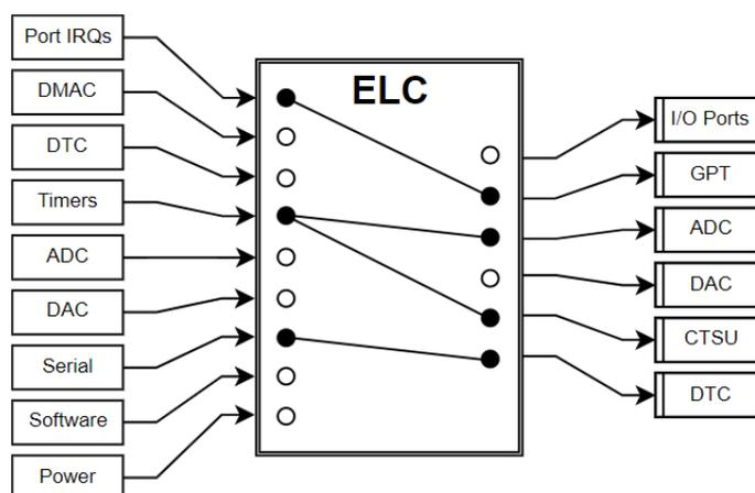
Figure 160: Event Link Controller Conceptual Diagram
