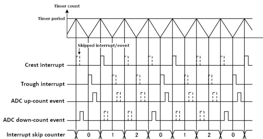
Figure 170: Crest interrupt skipping in triangle-wave PWM modes (skip count 2)
