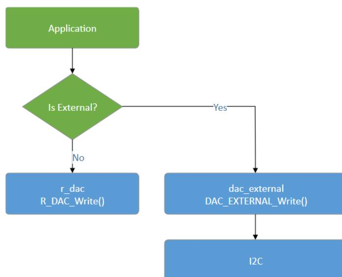
Figure 136: DAC Write with two write modules
