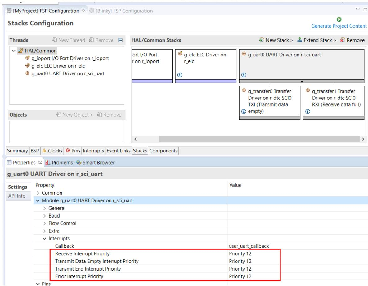
Figure 22: Configuring Interrupts in the Stacks tab
