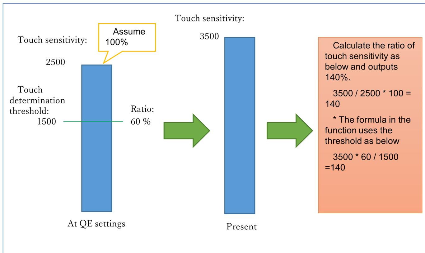
Figure 207: Example of increase touch sensitivity for thin overlay panels
