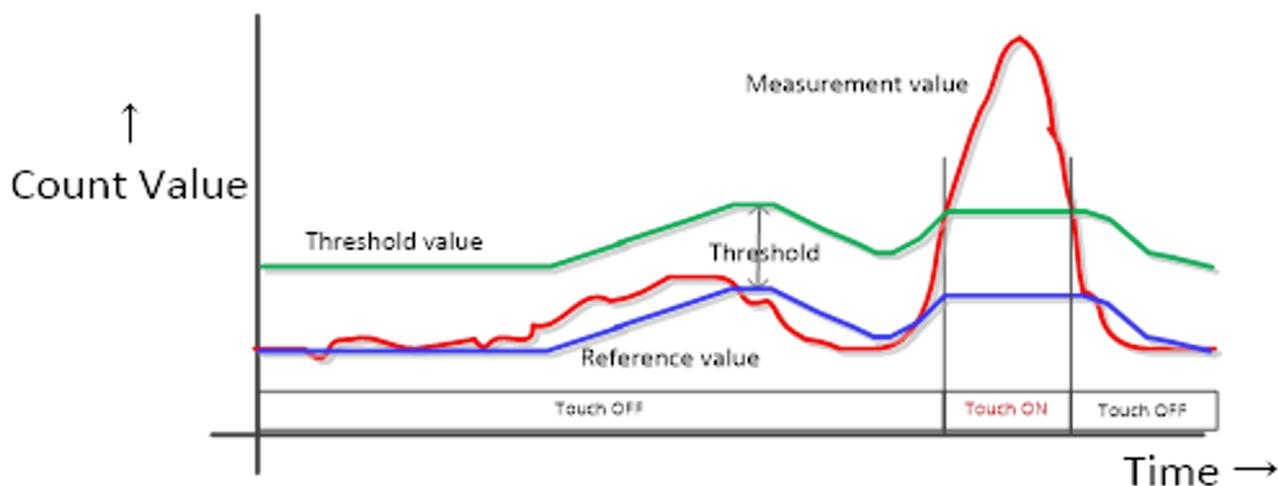
Figure 205: Button Touch Determination
