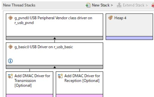
Figure 198: USB Peripheral Vendor Class Stack
