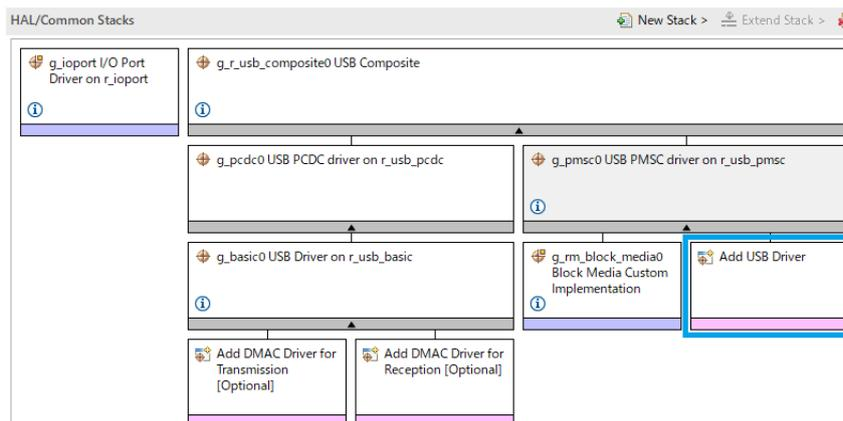
Figure 178: Delete USB Basic Instance
