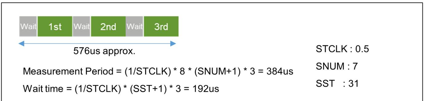
Figure 155: Self-capacitance Measurement Period (CTS2)
