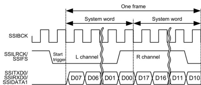
Figure 174: SSI Frame Diagram (8-bit word, 8-bit samples)
