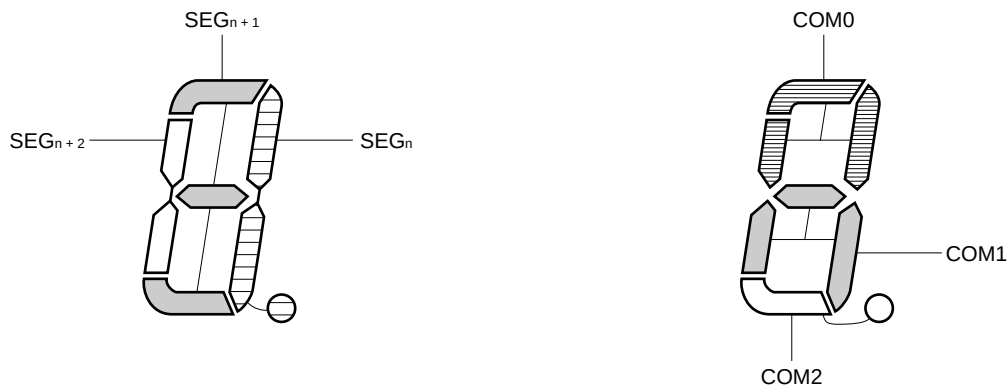
Figure 5-90. 3-Time-Division Type LCD Display Pattern and Electrode Wiring
