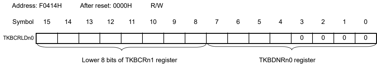
Figure 10 - 15 Format of 16-bit Timer KB Compare 1L & Dithering Count Register n0 (TKBCRLDn0)
