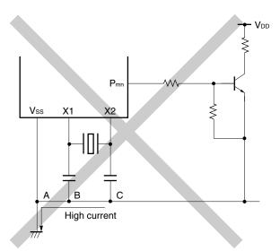
Figure 5-4. Examples of Incorrect Resonator Connection (2/2)
