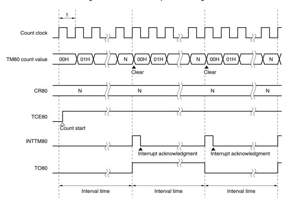
Figure 7-4. Interval Timer Operation Timing
