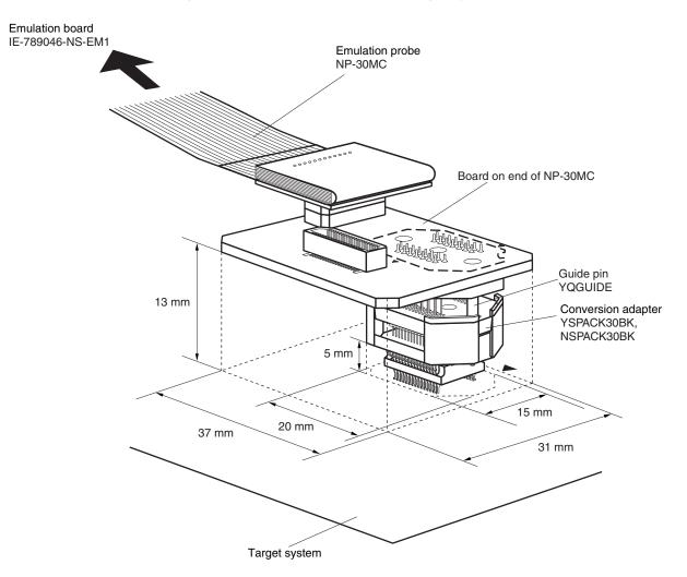
Figure B-2. Connection Condition of Target System
