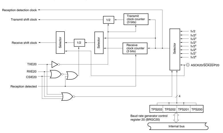
Figure 9-2. Block Diagram of Baud Rate Generator 20
