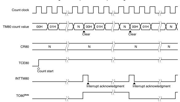
Figure 7-6. Square-Wave Output Timing
