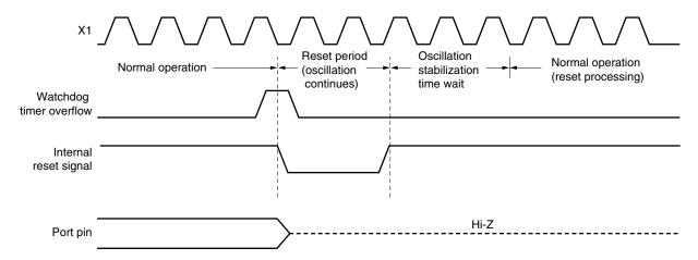
Figure 12-4. Reset Timing by RESET Input in STOP Mode
