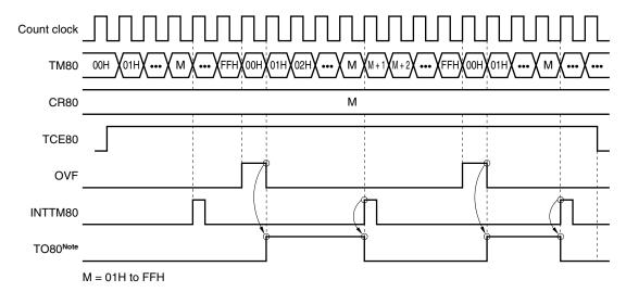
Figure 7-7. PWM Output Timing
