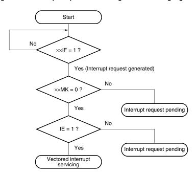
Figure 10-9. Interrupt Request Acknowledgment Processing Algorithm
