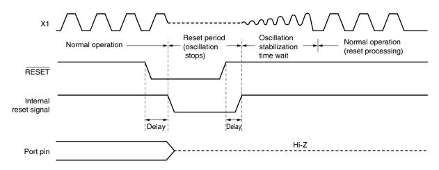
Figure 12-3. Reset Timing by Watchdog Timer Overflow
