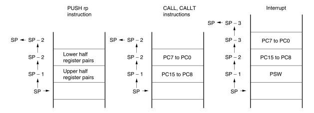
Figure 3-13. Data to Be Restored from Stack Memory
