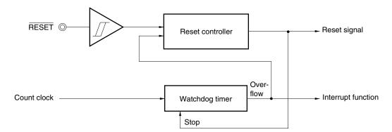
Figure 12-1. Block Diagram of Reset Function
