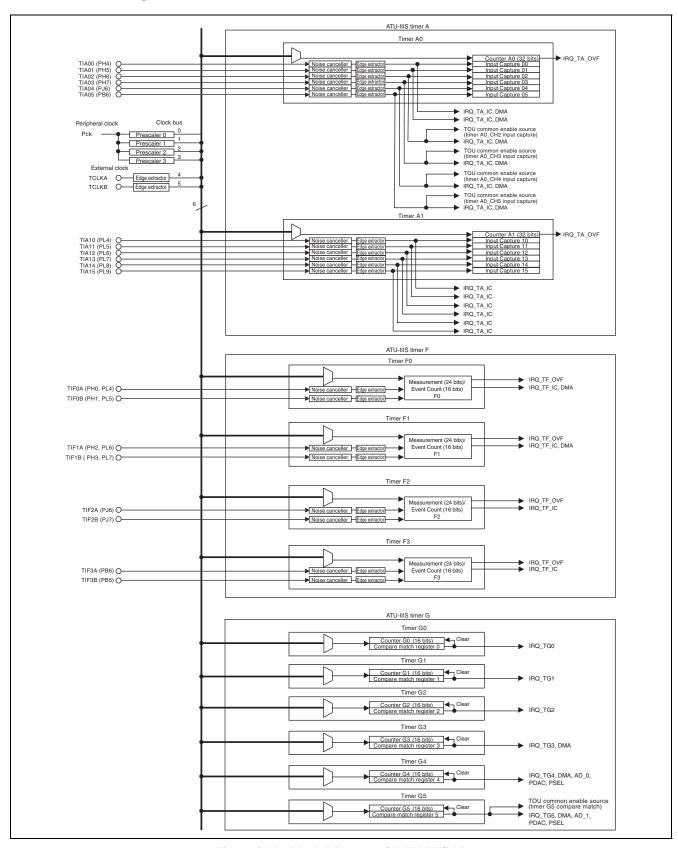
Figure 21.1 Block Diagram of ATU-IIIS (1)
