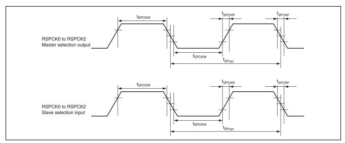
Figure 38.27 RSPI Clock Timing
