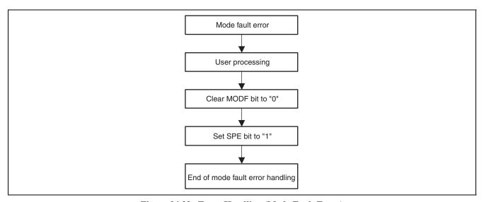
Figure 24.32 Error Handling (Mode Fault Error)
