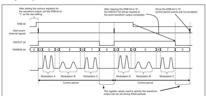
Figure 30.6 shows the relationship between the PDAC start event and both operation enable the operation monitor (during normal operation).
