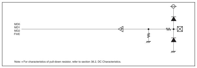
Figure 18.8 Port Peripheral Circuit Diagram (Input Port 4)
