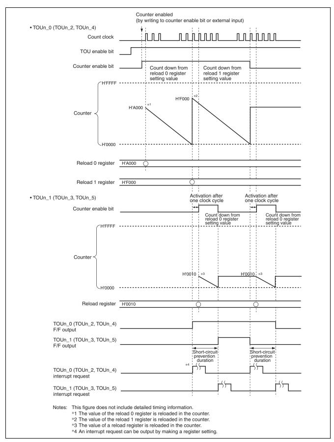
Figure 21.44 Overview of Short-Circuit Prevention Function Operation
