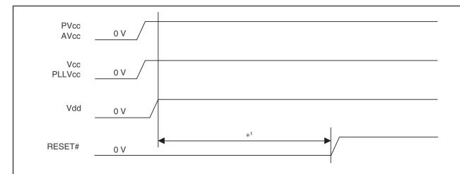
Notes: \*1 After applying all power supply levels and holding the RESET# pin at the "L" level for the oscillator stabilization time, apply a "H" level to the RESET# pin (reset clear).
