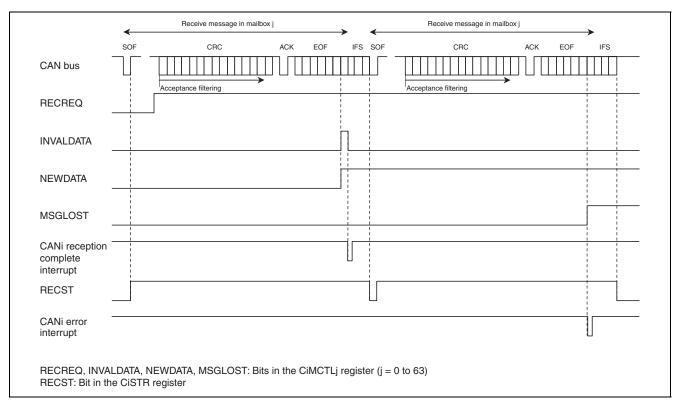
Figure 26.19 Operation Example of Data Frame Reception in Overrun Mode (i = 0 to 4)
