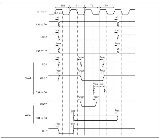
Figure 38.19 SRAM Bus Cycle with Byte Control (No Waits, No Address Setup/Hold, RDS = 1, RDH = 1, WTS = 1, WTH = 1)
