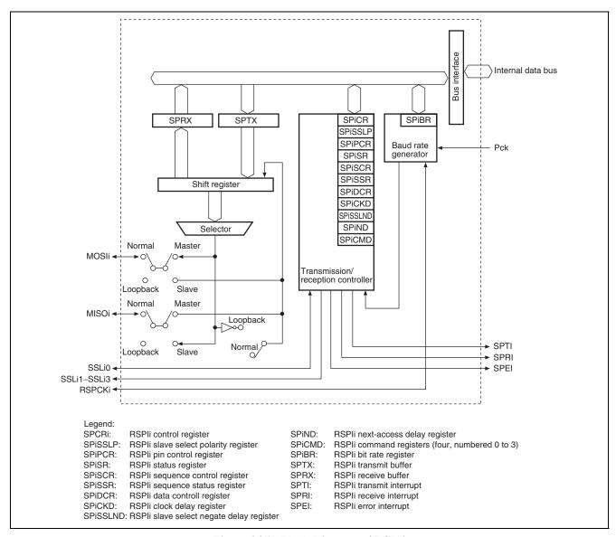
Figure 24.1 Block Diagram of RSPIi
