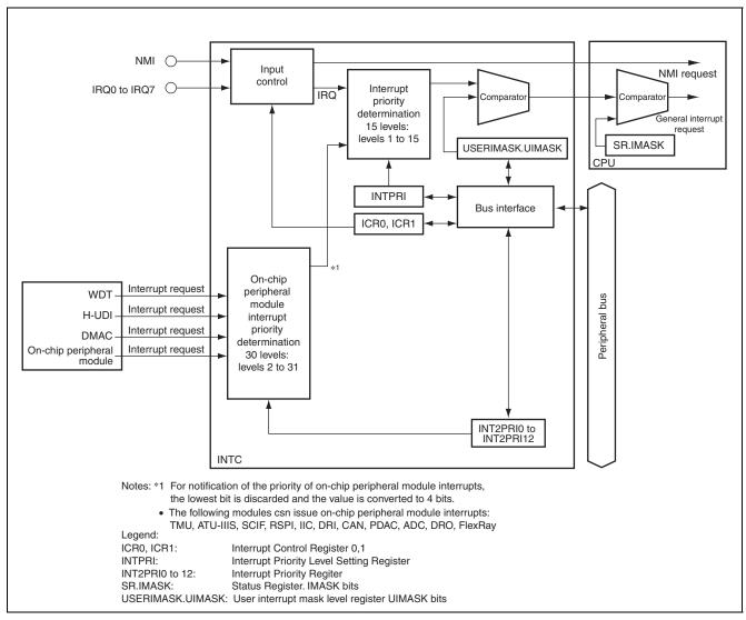
Figure 15.1 Block Diagram of INTC
