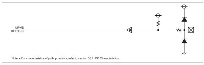
Figure 18.7 Port Peripheral Circuit Diagram (Input Port 3)
