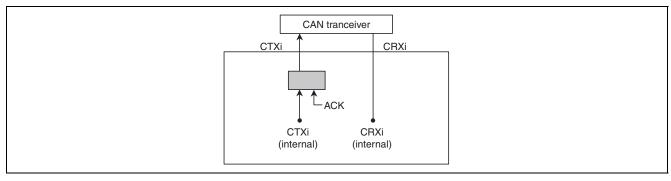
Figure 26.7 Connection when Self-Test Mode 0 is Selected
