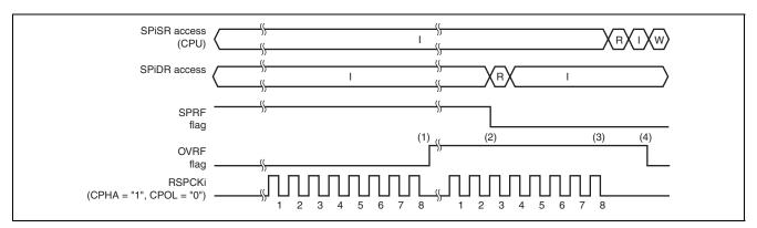
Figure 24.18 SPRF and OVRF Bit Operation Example
