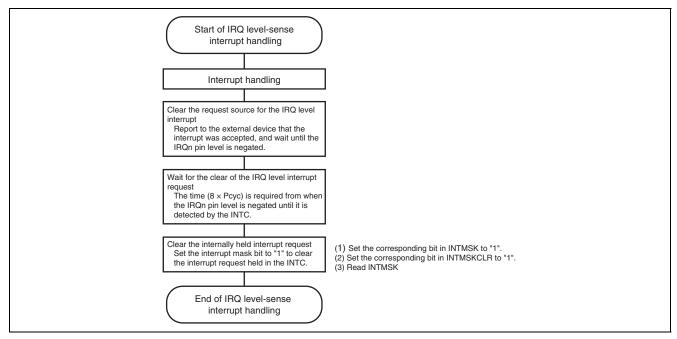
Figure 15.9 Example of Interrupt Handling Routine
