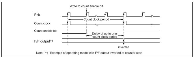
Figure 21.26 Count Clock Delay
