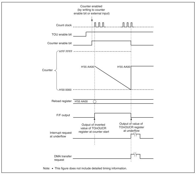
Figure 21.34 Operation Example of One-Shot Output Mode
