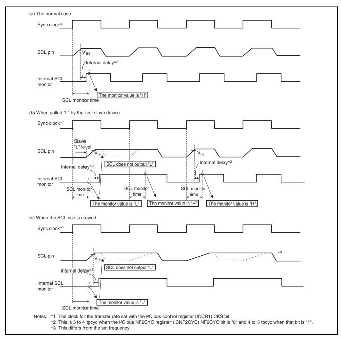
Figure 25.23 Bit Synchronous Circuit Timing
