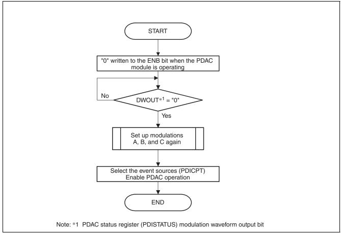
Figure 30.14 Example Procedure for Register Modification During PDAC Operation
