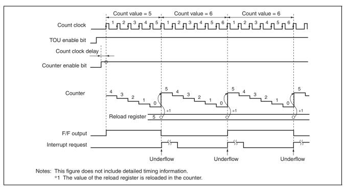
Figure 21.35 Example of Counter Operation in Continuous Output Mode
