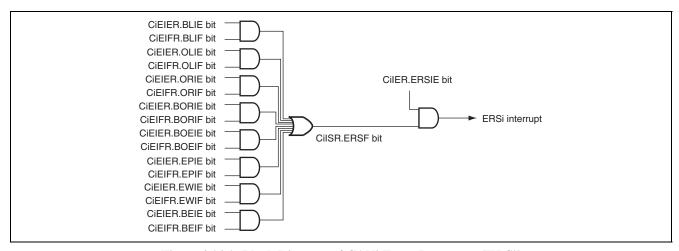
Figure 26.26 Block Diagram of CANi Error Interrrupt [ERSi]
