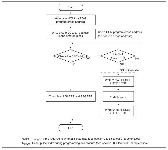
Figure 12.15 Procedure for Writing to the Lock Bit
