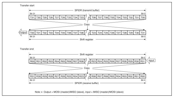
Figure 24.15 LSB First Transfer (32-Bit Data)
