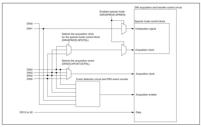
Figure 28.13 Signal Connections to Turn on/off Special Mode
