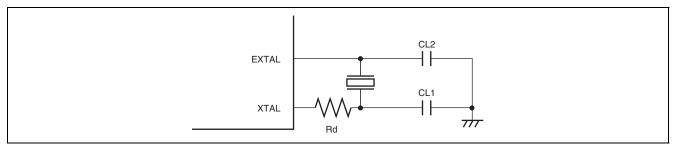
Figure 14.2 Crystal Resonator Connection Example
