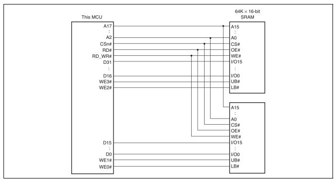
Figure 19.10 32-Bit Data Width Byte Control SRAM Connection Example
