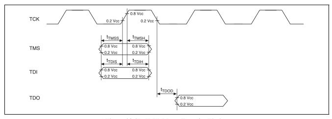
Figure 38.45 H-UDI Data Transfer Timing
