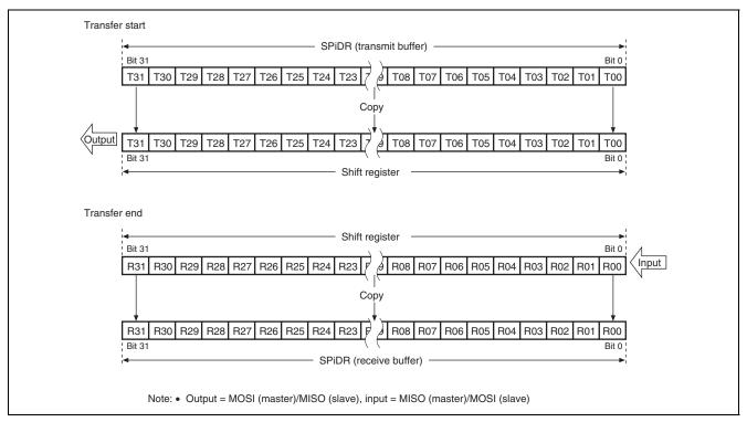
Figure 24.13 MSB First Transfer (32-Bit Data)
