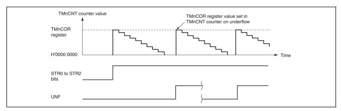
Figure 22.3 TMnCNT Counter Auto-Reload Operation
