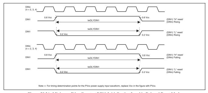
Figure 38.36 Minimum Edge Count at DIN1 Initialization Level in Delayed Reset Mode (Minimum Width at Initialization Level)
