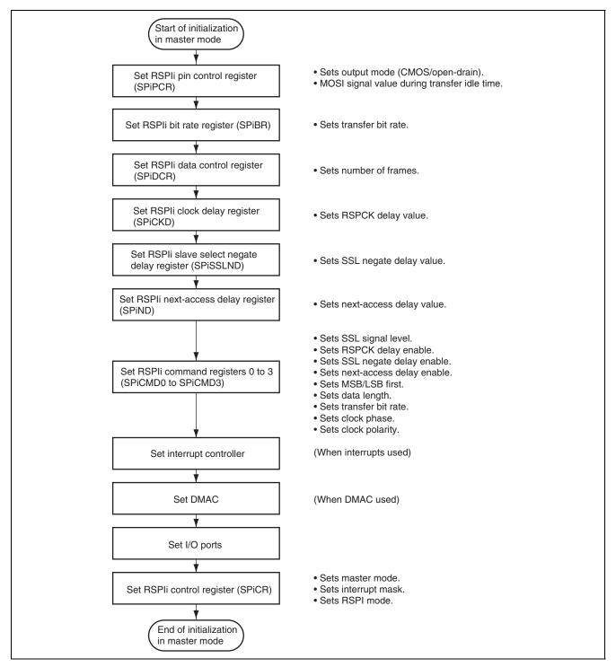
Figure 24.27 Flowchart of Initialization in Master Mode
