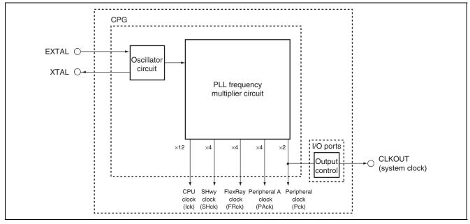
Figure 14.1 Block Diagram of CPG
