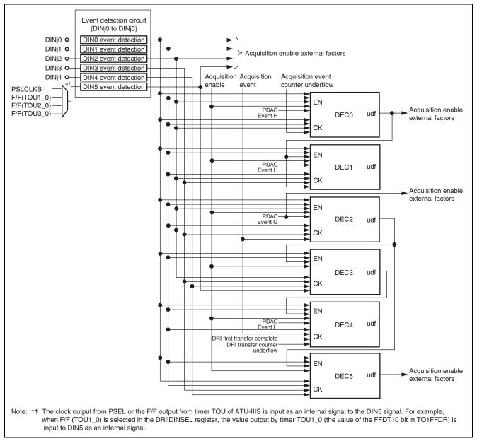
Figure 28.11 DEC Connection Diagram
