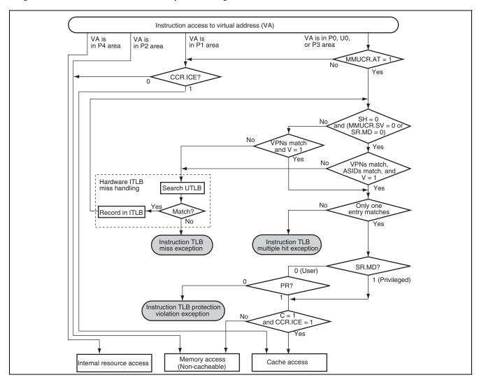
Figure 7.10 shows a flowchart of a memory access using the ITLB.
