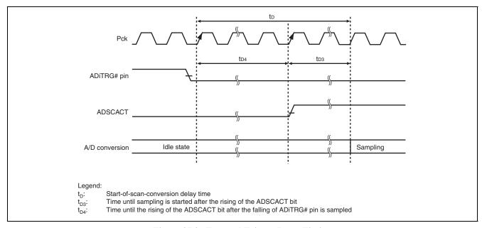
Figure 27.9 External Trigger Input Timing
