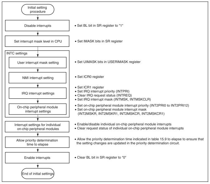
Figure 15.8 INTC Initial Setting Procedure Example
