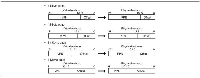
Figure 7.7 Relationship between Page Size and Address Format (TLB Compatible Mode)
