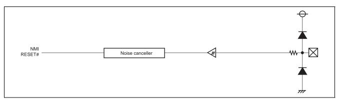
Figure 18.6 Port Peripheral Circuit Diagram (Input Port 2)
