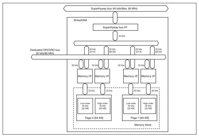
Figure 13.1 Block Diagram of SHwyRAM
