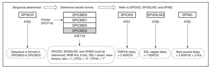
Figure 24.26 Determination Procedure of Serial Transfer Mode in Master Mode
