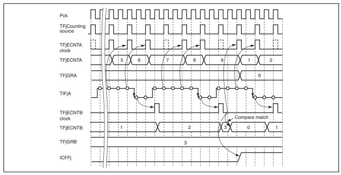
Figure 21.18 Operation Example of Measurement of Time during "H" Input Levels (TIFjA is in "H" Level When Capture is in Operation)
