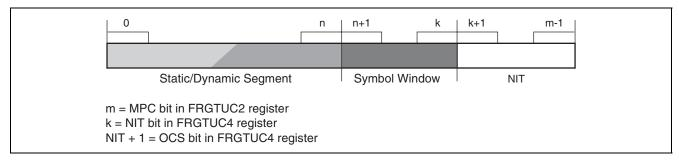
Figure 32.5 Configuration of NIT Start and Offset Correction Start
