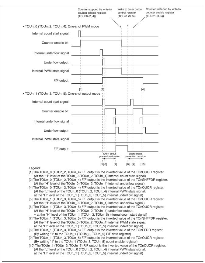
Figure 21.47 F/F Output and Register Settings with Output Forcibly Fixed by Software
