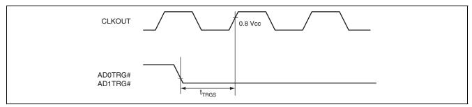
Figure 38.41 External Trigger Input Timing
