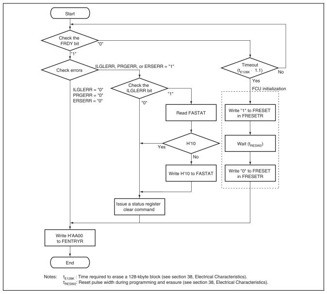
Figure 12.10 Procedure for Transition to ROM Read Mode
