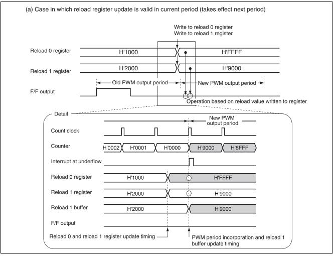
Figure 21.31 Reload 0 and Reload 1 Register Updating in PWM Output Mode (0% Duty Cycle)
