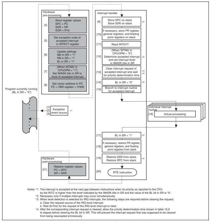
Figure 15.4 General Interrupt Operation Example 1
