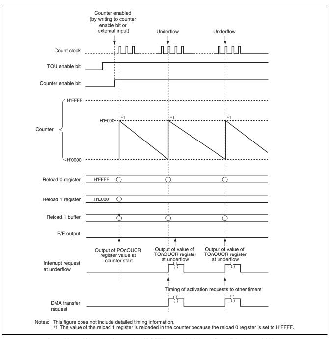
Figure 21.37 Operation Example of PWM Output Mode (Reload 0 Register: H'FFFF)
