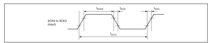
Figure 38.25 SCK Input Timing
