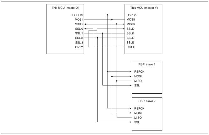
Figure 24.8 Multi-Master/Multi-Slave Configuration Example (This MCU = Master)
