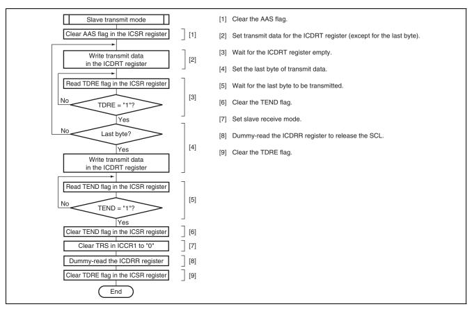
Figure 25.21 Sample Flowchart for Slave Transmit Mode
