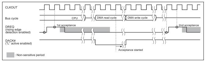
Figure 20.10 Example of DREQ Input Detection (Cycle Steal Mode 1, DACK Read Cycle Output)
