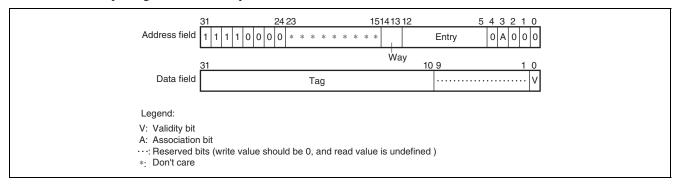
Figure 8.5 Memory-Mapped IC Address Array (Cache size = 32 Kbytes)
