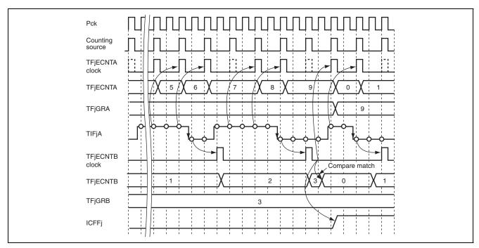
Figure 21.17 Operation Example of Measurement of Time during "H" Input Levels
