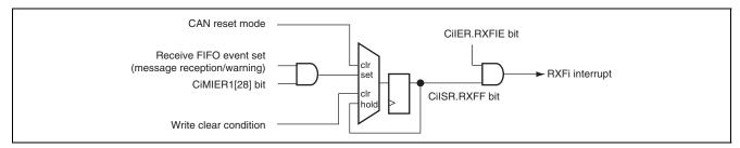
Figure 26.24 Block Diagram of CANi Receive FIFO Interrupt [RXFi]
