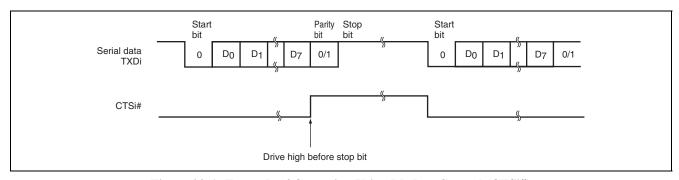
Figure 23.6 Example of Operation Using Modem Control (CTSi#)
