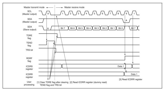
Figure 25.7 Master Receive Mode Operation Timing (1)
