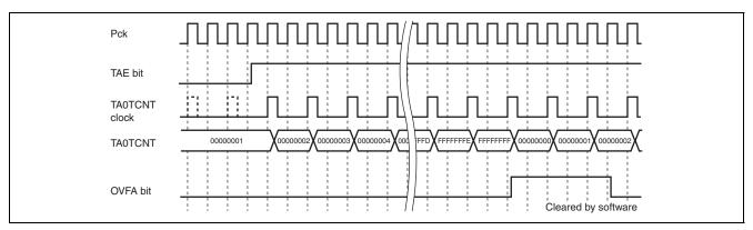
Figure 21.11 Timer A Free-Running Operation: Overflow Timing
