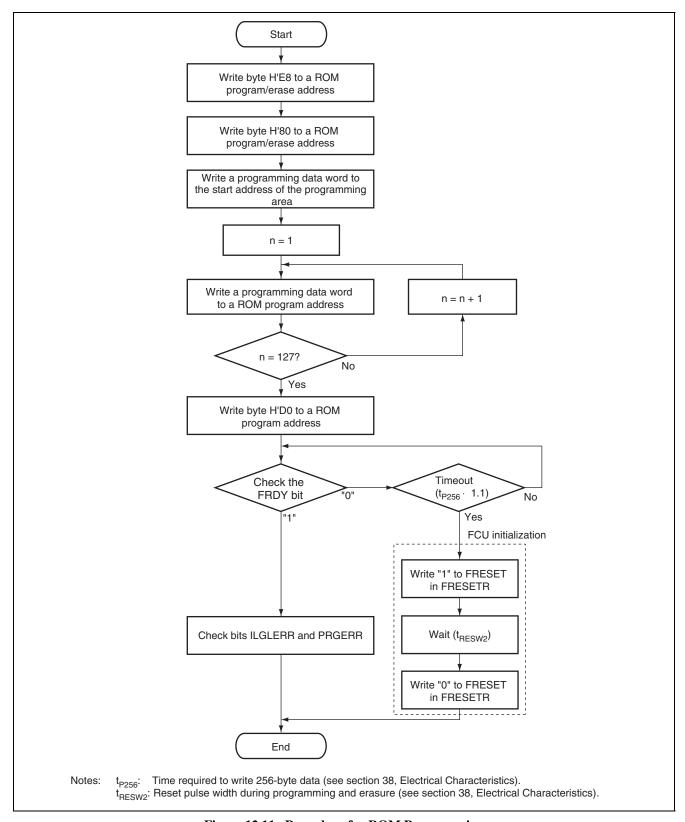
Figure 12.11 Procedure for ROM Programming
