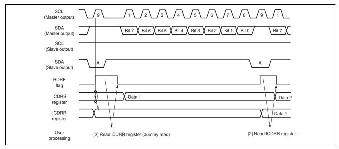
Figure 25.11 Slave Receive Mode Operation Timing (1)
