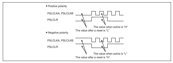
Figure 31.2 PSEL Output Signal Polarity
