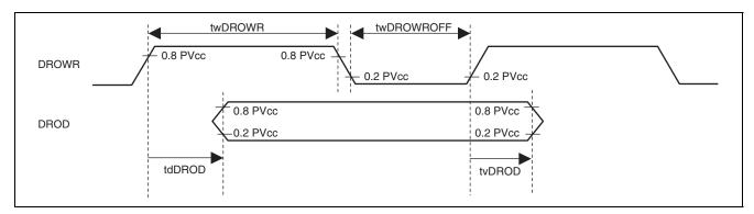
Figure 38.38 Strobe Polarity with "H" Active Selected
