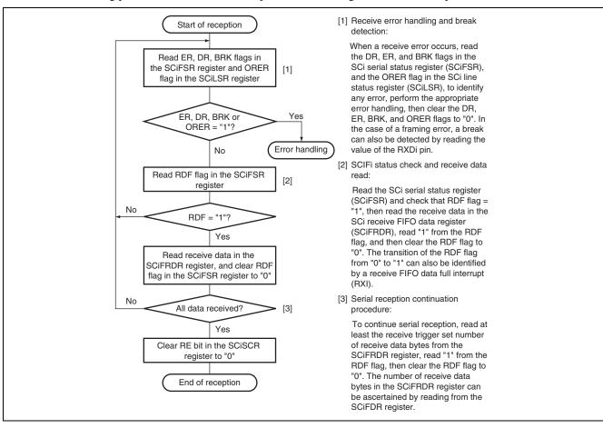
Figure 23.7 Sample Flowchart for Receiving Serial Data (1)
