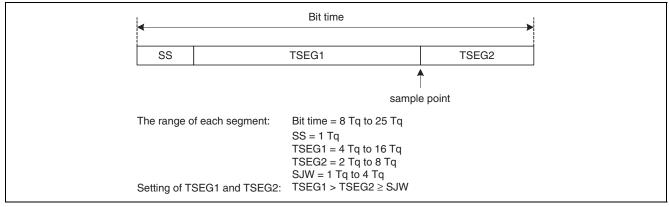
Figure 26.12 Bit Timing
