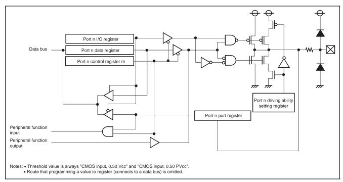
Figure 18.2 Port Peripheral Circuit Diagram (Input/Output Ports 2)
