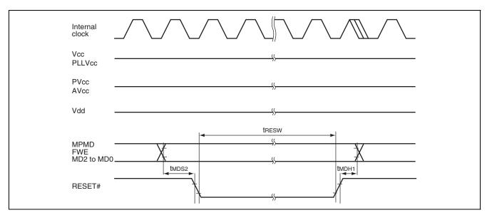
Figure 38.6 Operation Mode and Oscillation Timing during Operation
