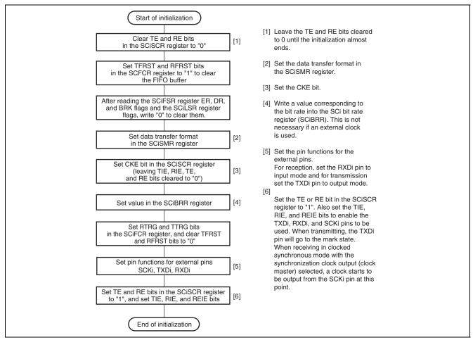
Figure 23.12 Sample Flowchart for SCIFi Initialization
