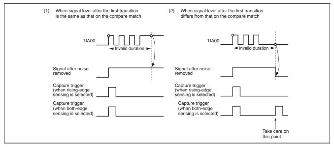
Figure 21.9 Example of Noise Cancellation in Premature-Transition Cancellation for Two Types of Waveforms
