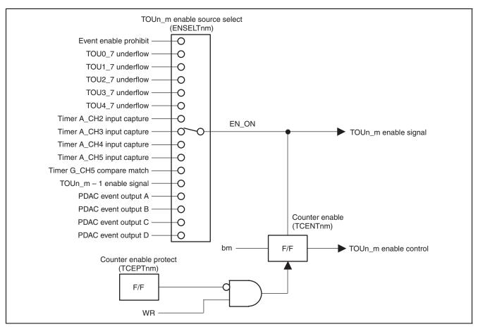
Figure 21.27 TOU Enable Circuit Configuration Diagram
