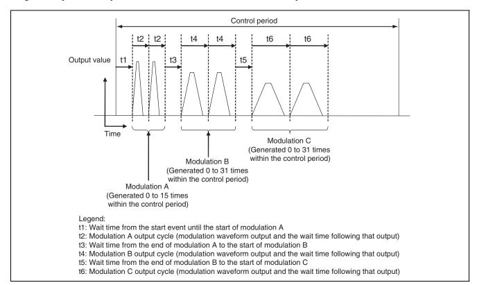
Figure 30.4 presents an operational overview of the PDAC module control period.
