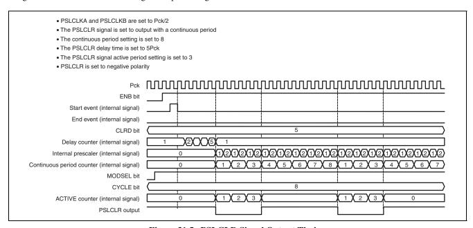
Figure 31.5 PSLCLR Signal Output Timing
