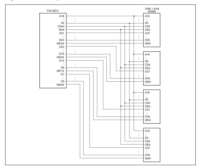
Figures 19.4 to 19.6 show examples of the connection to SRAM with data width of 32, 16, and 8 bits.
