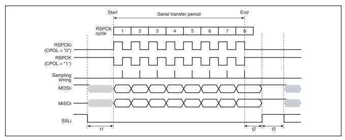
Figure 24.12 RSPI Transfer Format (CPHA = "1")
