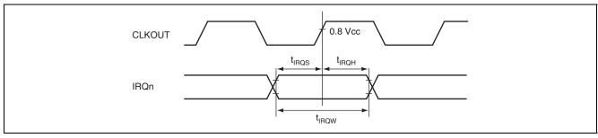
Figure 38.11 Interrupt Signal Input Timing
