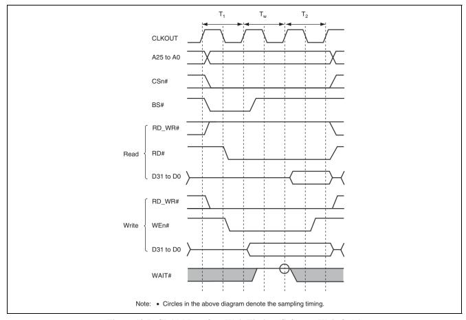
Figure 19.7 SRAM Interface Wait Timing (Software Wait Only)
