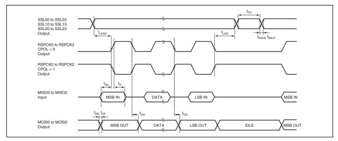
Figure 38.28 RSPI Timing (Master, CPHA = "0")
