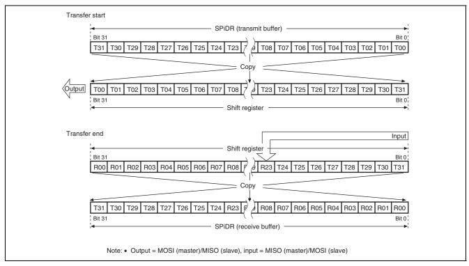
Figure 24.16 LSB First Transfer (24-Bit Data)
