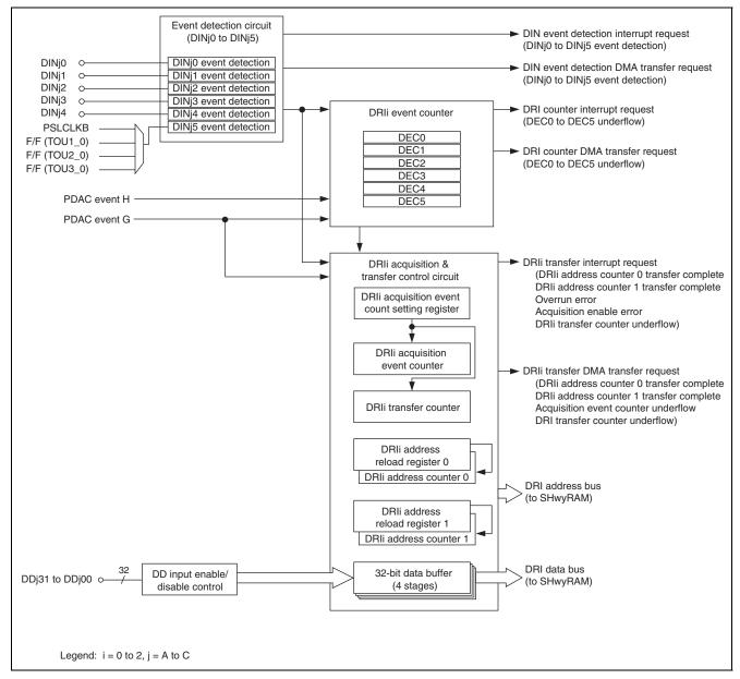
Figure 28.1 shows the block diagram of the DRIi module.
