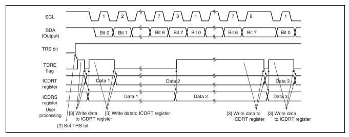
Figure 25.14 Transmit Mode Operation Timing
