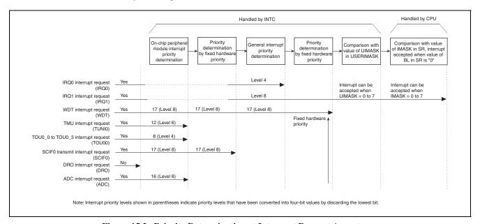
Figure 15.2 Priority Determination at Interrupt Request Acceptance
