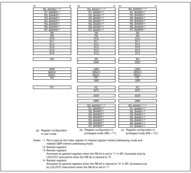
Figure 2.2 CPU Register Configuration in Each Processing Mode
