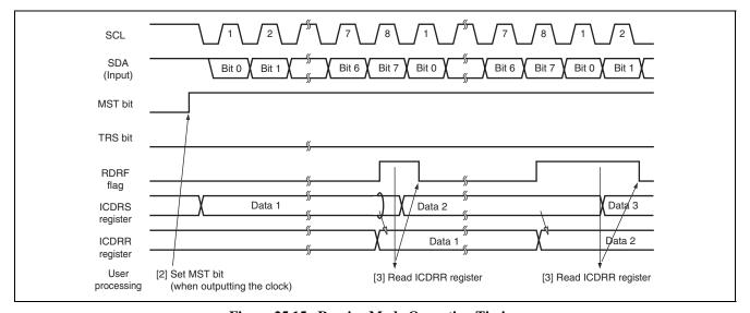
Figure 25.15 Receive Mode Operation Timing
