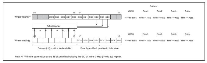
Figure 26.5 Write and Read of CiAFSR Register (i = 0 to 4)
