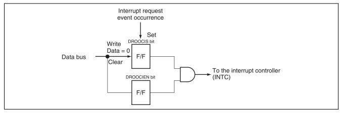
Figure 29.2 Relationship Between DROIST and DROIEN Registers
