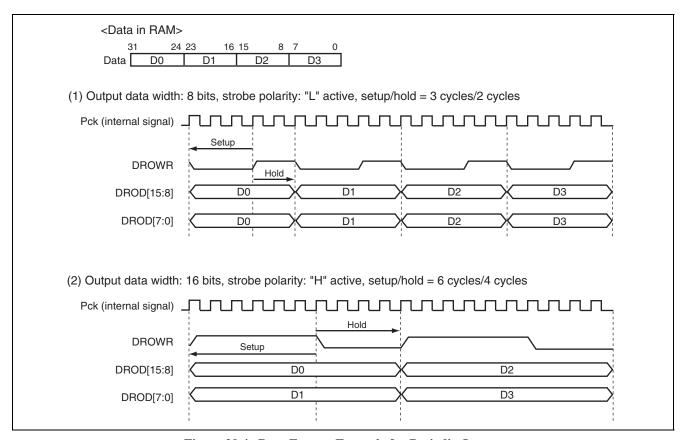
Figure 29.4 Data Format Example for Periodic Output
