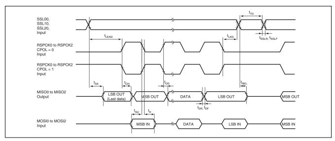
Figure 38.31 RSPI Timing (Slave, CPHA = "1")
