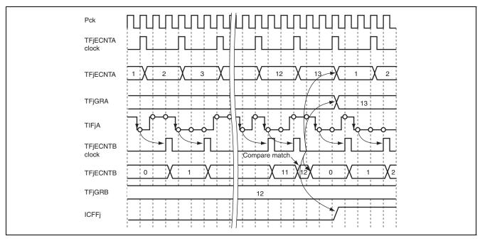
Figure 21.16 Operation Example of Valid Edge Interval Counting
