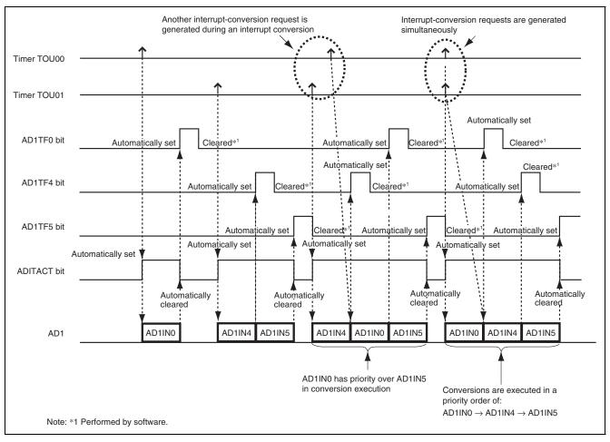
Figure 27.6 Example Operation of Interrupt Conversion
