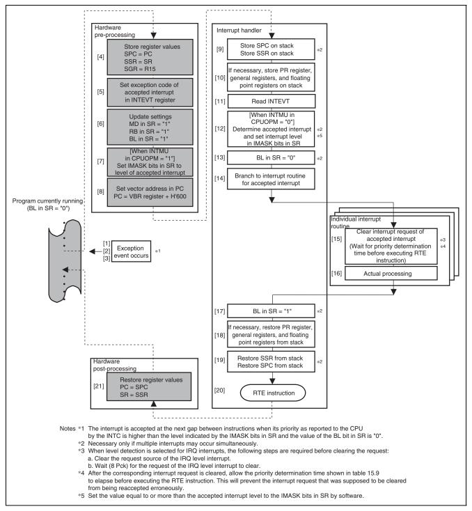
Figure 15.5 General Interrupt Operation Example 2
