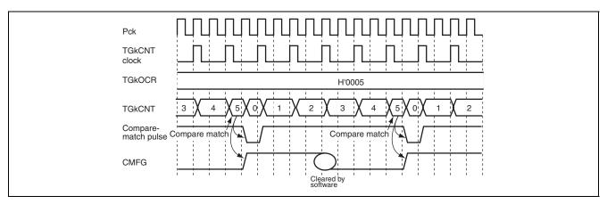
Figure 21.24 Operation Example of Counter and Compare Match
