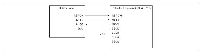
Figure 24.5 Single-Master/Single-Slave Configuration Example (This MCU = Slave, CPHA = "1")
