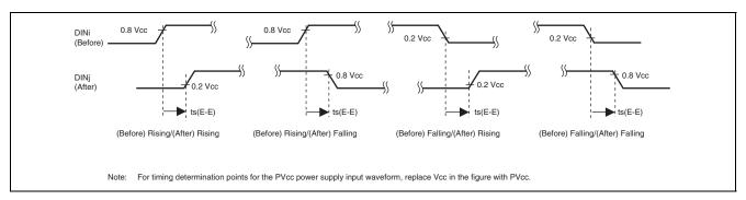
Figure 38.34 Edge Detection Timing (Edge Interval to Prevent DRI Internal Simultaneous Edge Detection Timing)
