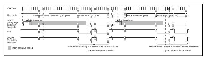
Figure 20.18 Timing Example during DACK# Signal Output Division (Cycle Steal Mode 1 or 2, DACK Write Cycle Output)
