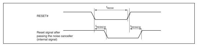
Figure 38.9 Reset Input Timing
