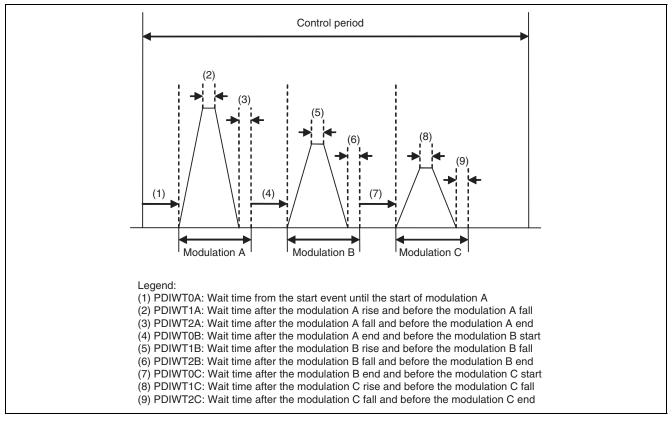
Figure 30.5 Relationship between Output Waveform and Wait Time Setting Registers in the PDAC Control Period
