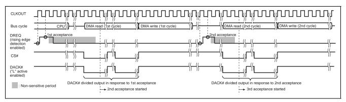
Figure 20.17 Timing Example during DACK# Signal Output Division (Cycle Steal Mode 1 or 2, DACK Read Cycle Output)
