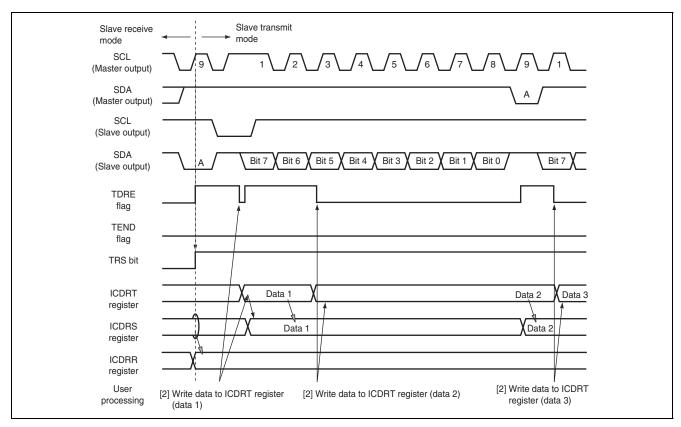
Figure 25.9 Slave Transmit Mode Operation Timing (1)
