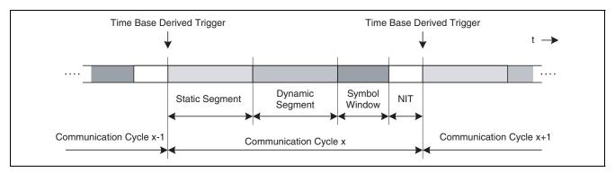
Figure 32.4 Structure of Communication Cycle
