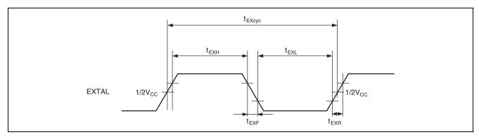
Figure 38.7 EXTAL Clock Input Timing
