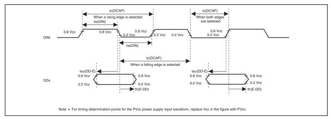
Figure 38.33 Data Acquisition Related Timing
