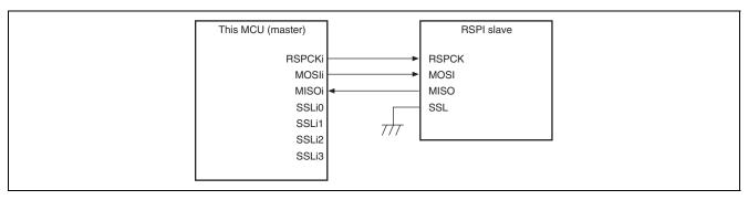
Figure 24.3 Single-Master/Single-Slave Configuration Example (This MCU = Master)
