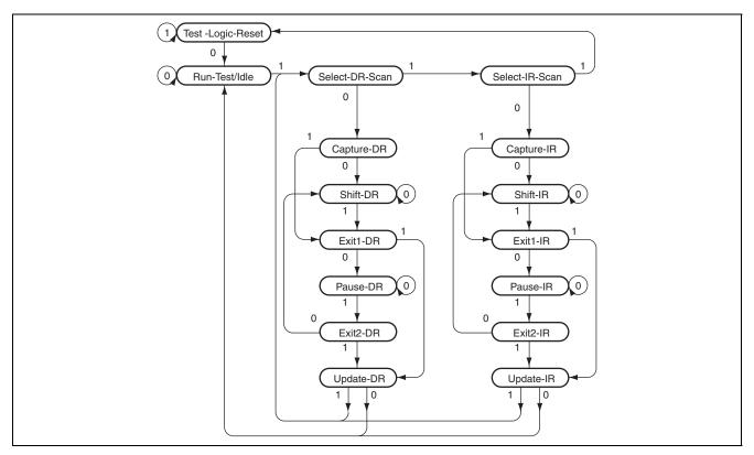
Figure 37.3 TAP Controller State Transitions
