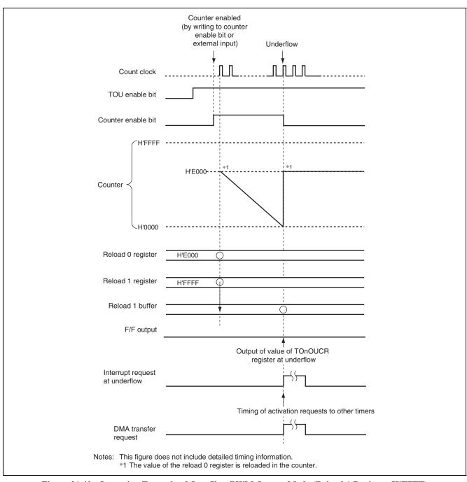
Figure 21.40 Operation Example of One-Shot PWM Output Mode (Reload 1 Register: H'FFFF)
