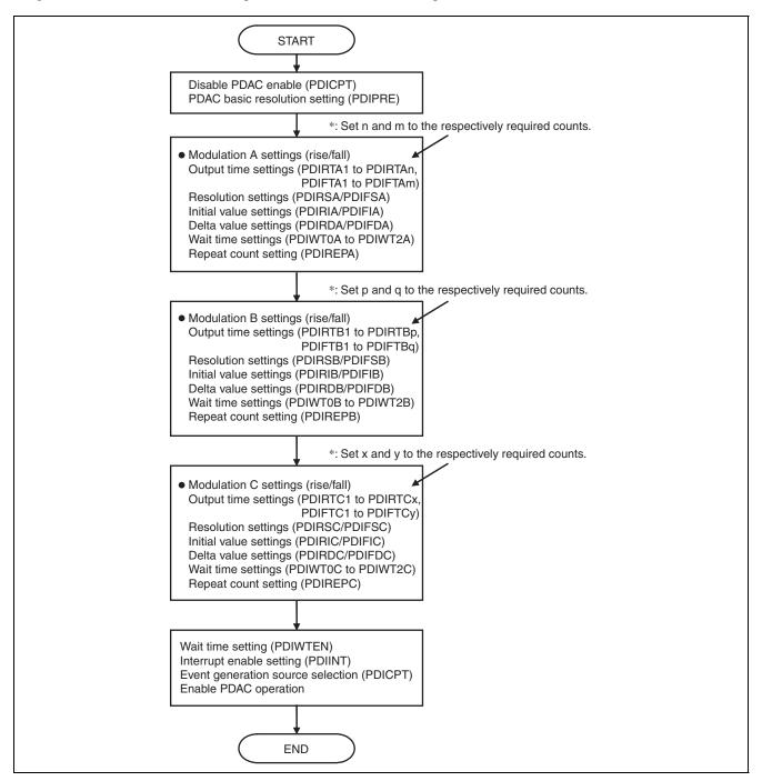
Figure 30.13 Initialization Procedure (When starting for the first time)
