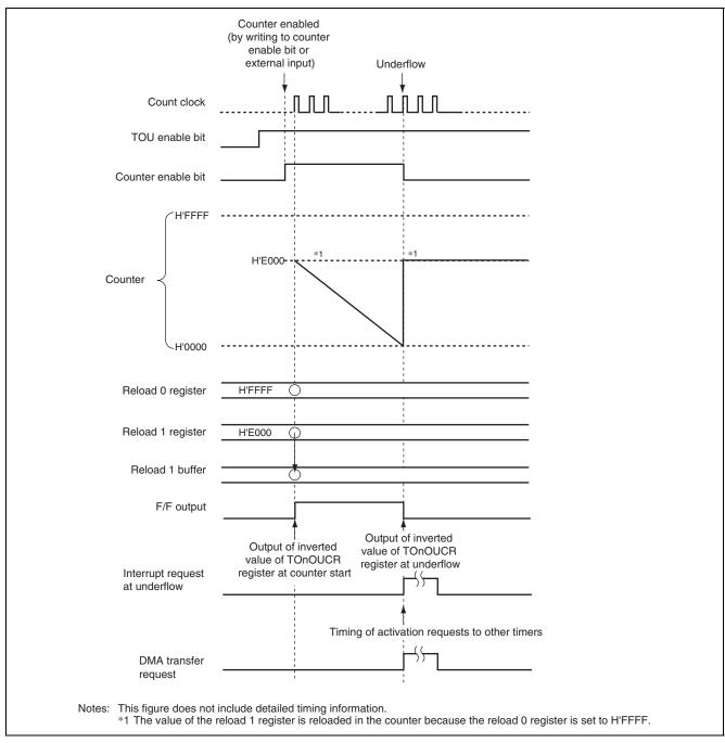
Figure 21.39 Operation Example of One-Shot PWM Output Mode (Reload 0 Register: H'FFFF)
