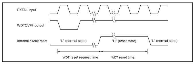
Figure 17.3 WDT Overflow Hardware Reset During Normal Operation
