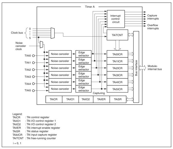
Figure 21.7 Block Diagram of Timer A
