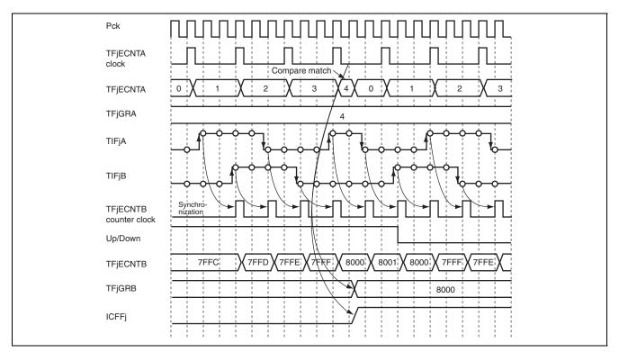
Figure 21.22 Operation Example of Four-time Multiplication Event Count
