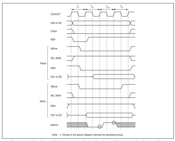
Figure 19.14 Byte Control SRAM Basic Access Timing (One Internal Wait Cycle + One External Wait)
