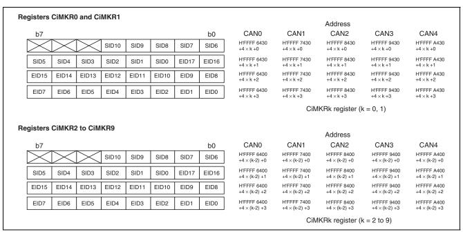
Figure 26.14 Structure of CiMKRk Register (i = 0 to 4; k = 0 to 9)
