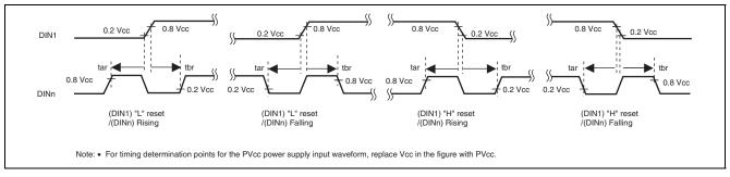
Figure 38.35 DIN1/DIN2 to DIN4 Related Timing in Special Mode (DIN1 Reset Release Edge and Preceding or Subsequent Sampling Edge Interval)
