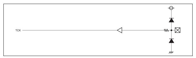
Figure 18.10 Port Peripheral Circuit Diagram (Input Port 6)
