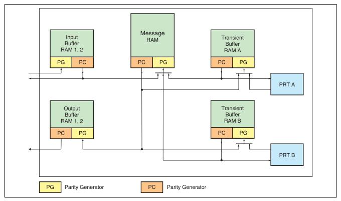
Figure 32.20 Parity Generation and Check
