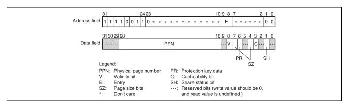
Figure 7.19 Memory-Mapped ITLB Data Array (TLB Compatible Mode)
