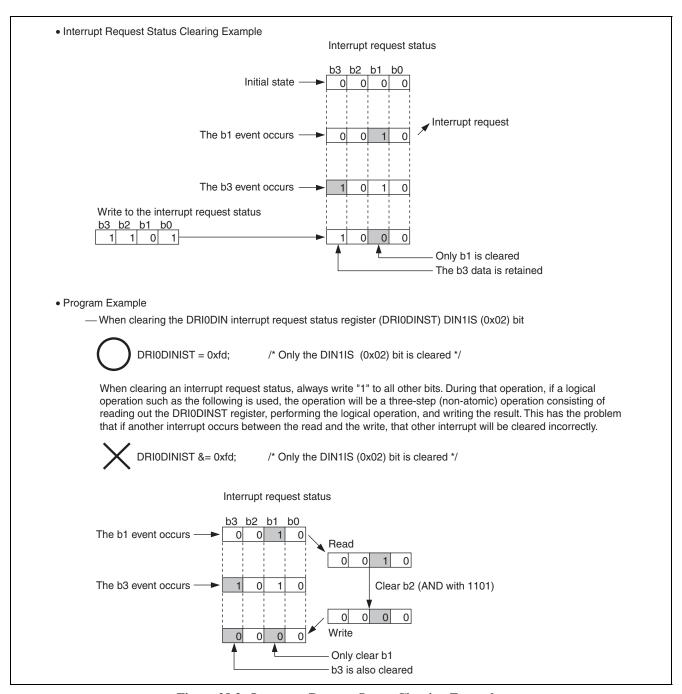
Figure 28.3 Interrupt Request Status Clearing Examples
