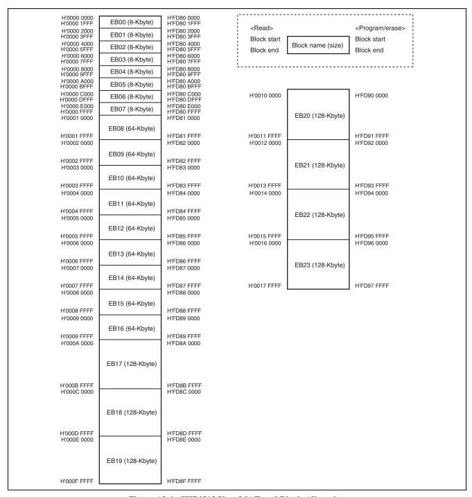
Figure 12.4 SH74513 User MAT and Block Allocation
