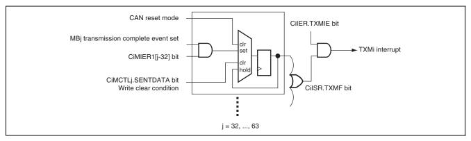
Figure 26.23 Block Diagram of CANi Transmission Complete Interrupt (Mailbox 32 to 63) [TXMi]
