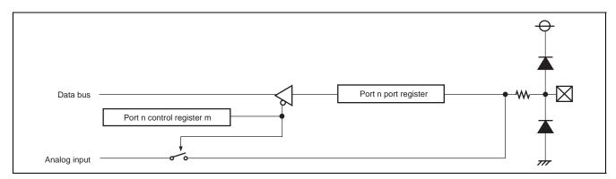
Figure 18.5 Port Peripheral Circuit Diagram (Input Port 1)
