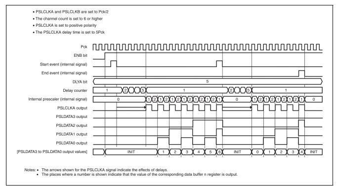
Figure 31.4 PSEL Data Output Timing
