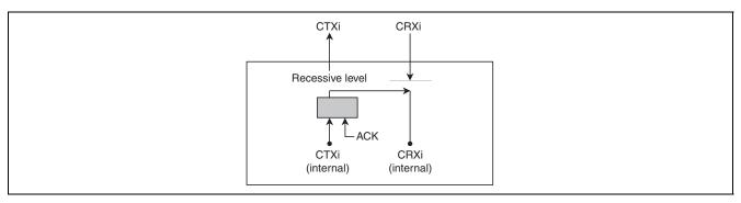
Figure 26.8 Connection when Self-Test Mode 1 is Selected
