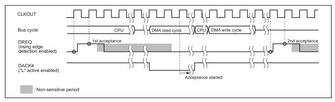
Figure 20.12 Example of DREQ Input Detection (Cycle Steal Mode 2, DACK Read Cycle Output)
