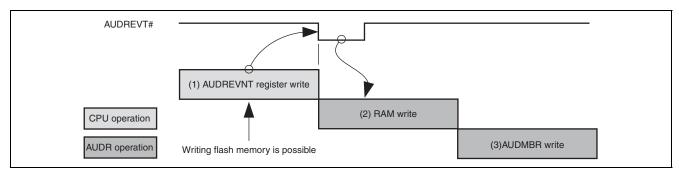
Figure 36.3 AUDR Module Usage Example (AUDR module flash memory write operation)
