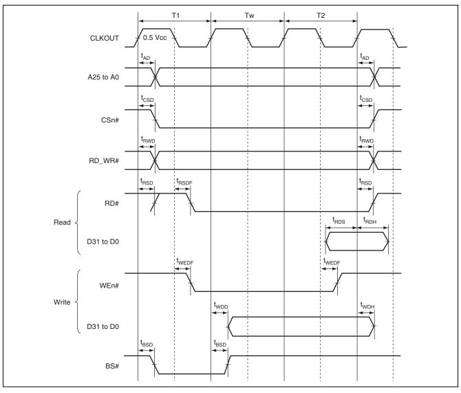
Figure 38.13 SRAM Bus Cycle (One Software Wait Cycle)
