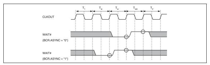
Figure 19.2 BCR.ASYNC Setting WAIT# Sampling Timing Example (Two wait cycle insertion is specified with the CSnWCR register.)
