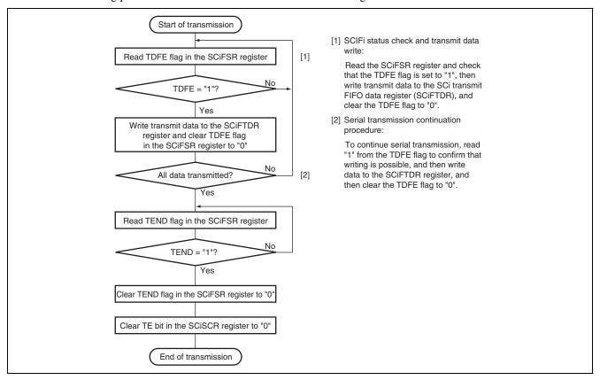
Figure 23.13 Sample Flowchart for Transmitting Serial Data
