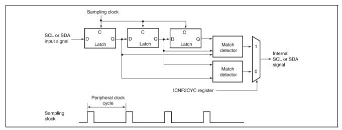
Figure 25.17 Block Diagram of Noise Filter
