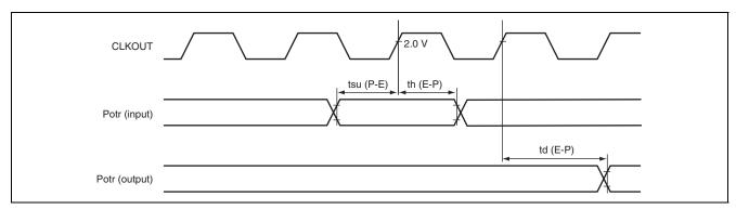
Figure 38.23 I/O Port Input/Output Timing
