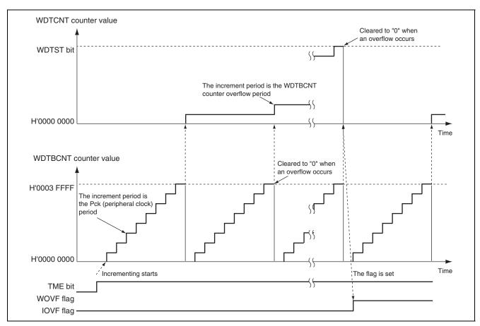
Figure 17.2 WDT Increment Operations (in interval timer mode)
