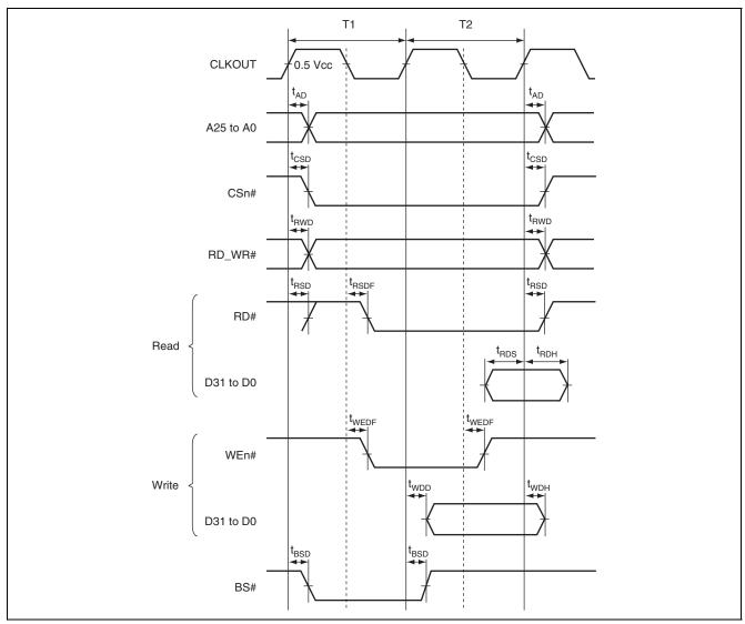
Figure 38.12 SRAM Bus Cycle (No Waits)
