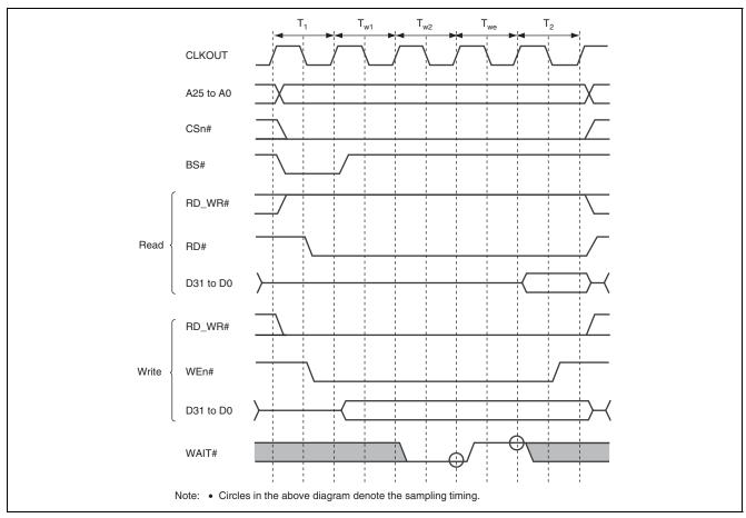
Figure 19.8 External Space Access Wait Timing (WAIT# Signal Wait Insertion)
