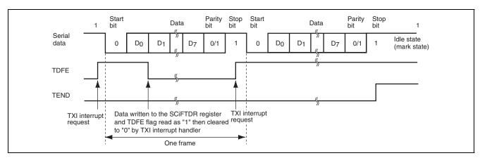
Figure 23.5 Example of Transmit Operation (8-Bit Data, Parity, 1 Stop Bit)
