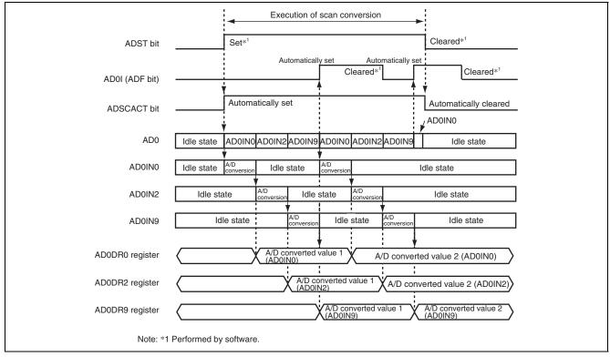
Figure 27.5 Example Operation in Continuous Scan Mode
