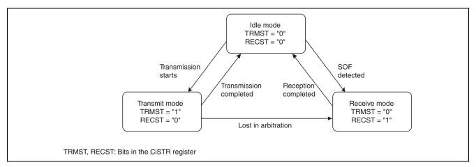
Figure 26.10 Sub Mode in CAN Operation Mode (i = 0 to 4)
