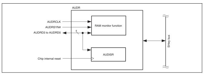
Figure 36.9 Configuration Information Retention Function Block Diagram
