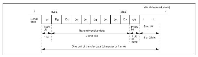
Figure 23.2 Example of Data Format in Asynchronous Communication (8-Bit Data with Parity and Two Stop Bits)
