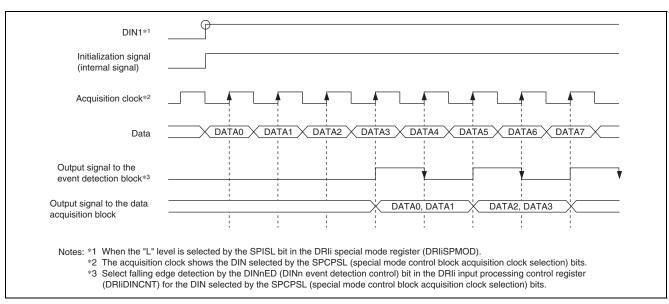
Figure 28.6 Timing Chart when Special Mode is Enabled
