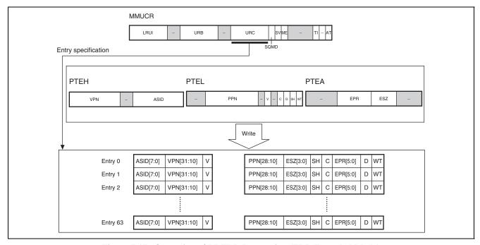
Figure 7.17 Operation of LDTLB Instruction (TLB Extended Mode)
