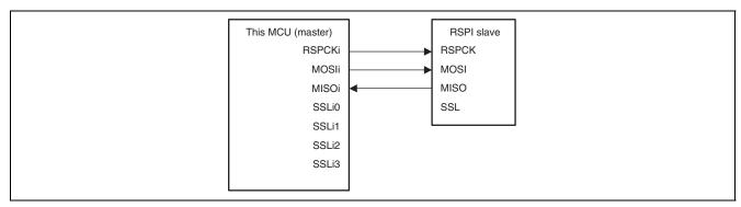
Figure 24.9 Master (Clock-Synchronous Operation)/Slave (Clock-Synchronous Operation) Configuration Example (This MCU = Master)
