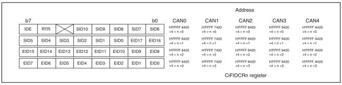
Figure 26.15 Structure of CiFIDCRn register (i = 0 to 4; n = 0, 1)
