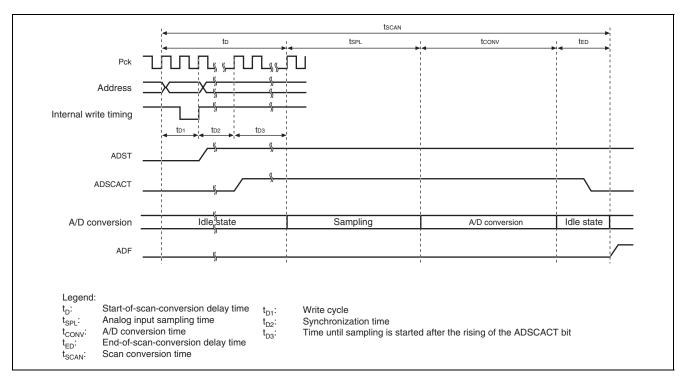
Figure 27.8 Timing Diagram for Scan Conversion (Single Channel, Single Cycle)
