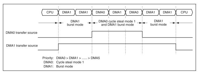
Figure 20.7 Example of Operations in Priority Order in Burst Mode
