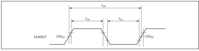
Figure 38.8 System Clock Timing
