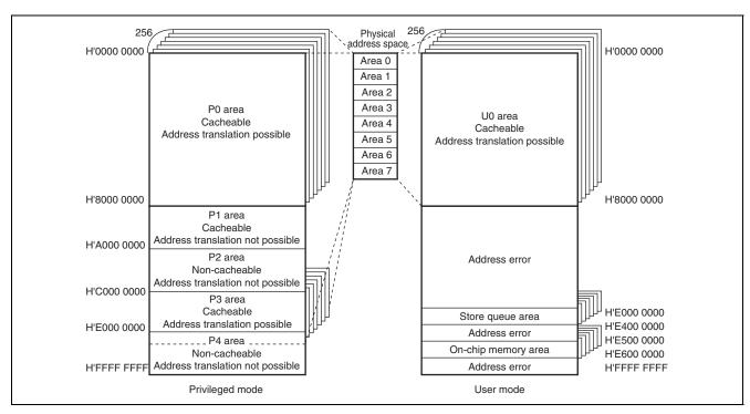
Figure 7.3 Virtual Address Space (AT in MMUCR = 1)
