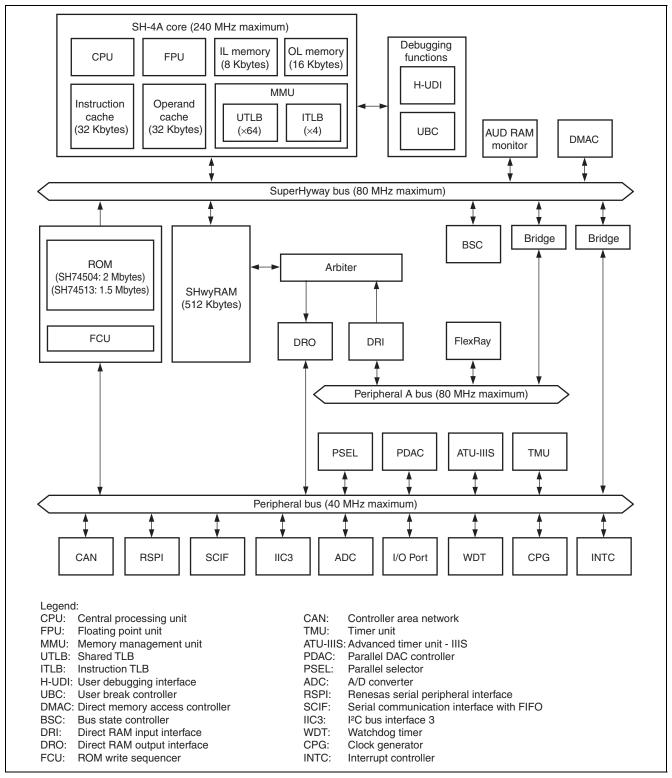
Figure 1.1 Block Diagram
