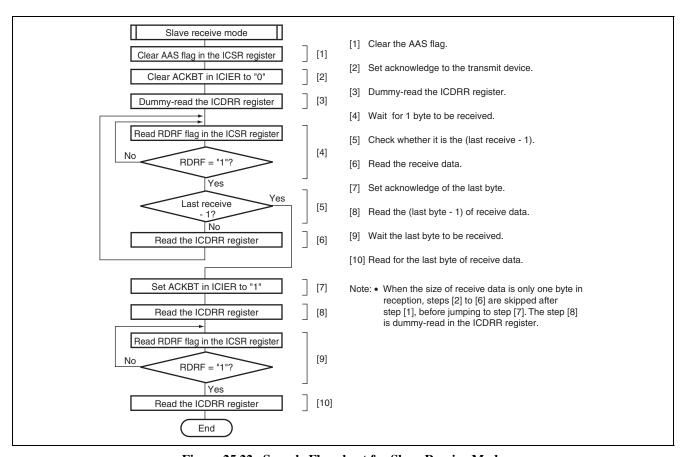
Figure 25.22 Sample Flowchart for Slave Receive Mode
