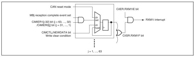
Figure 26.22 Block Diagram of CANi Reception Complete Interrupt (Mailbox 1 to 63) [RXM1i]
