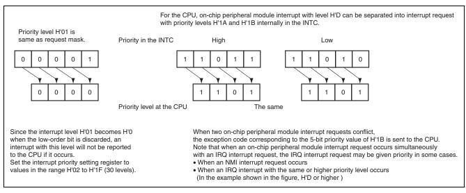
Figure 15.3 On-Chip Peripheral Module Interrupt Priority
