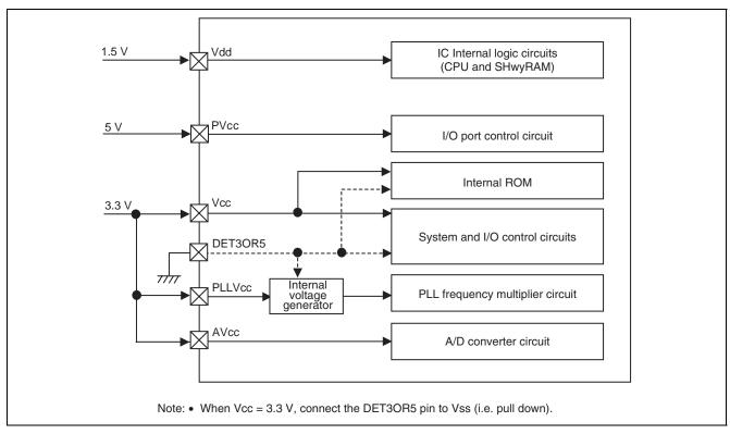
Figure 34.2 Power Supply Circuit Structure (when PVcc = 5 V, Vcc = 3.3 V)
