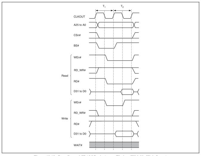
Figure 19.12 Byte Control SRAM Basic Access Timing (With No Wait States)
