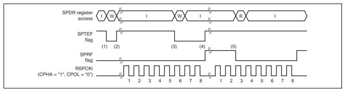
Figure 24.17 SPTEF and SPRF Bit Operation Example
