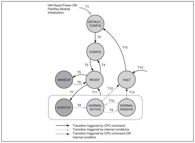
Figure 32.6 Overall State Diagram of FlexRay Communication Controller
