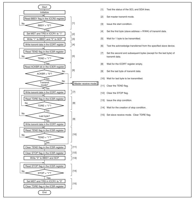
Figure 25.19 Sample Flowchart for Master Transmit Mode
