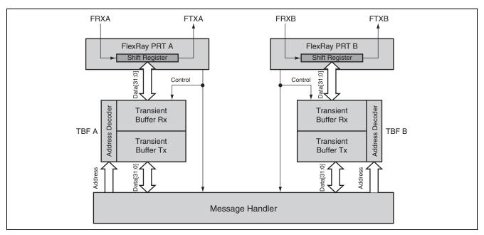
Figure 32.16 Access to Transient Buffer RAMs
