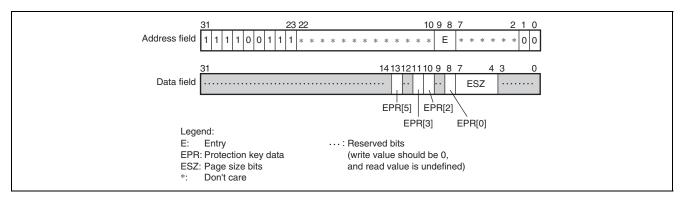
Figure 7.21 Memory-Mapped ITLB Data Array 2 (TLB Extended Mode)
