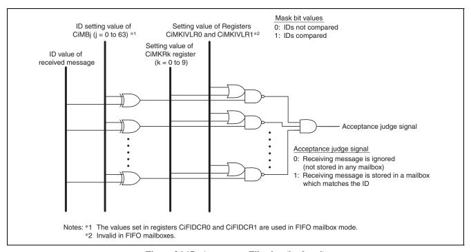
Figure 26.17 Acceptance Filtering (i = 0 to 4)
