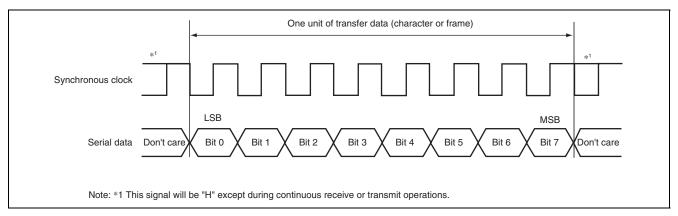
Figure 23.11 Data Format in Clock Synchronous Communication
