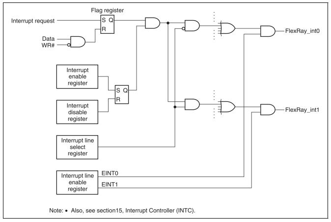
Figure 32.2 Block Diagram of FlexRay Interrupt Requests 0/1
