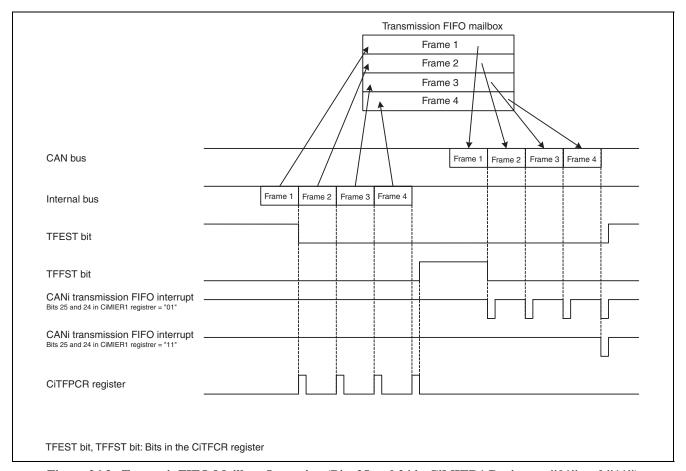
Figure 26.3 shows the transmit FIFO mailbox operation.
