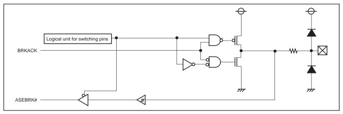
Figure 18.4 Port Peripheral Circuit Diagram (Input/Output Ports 4)
