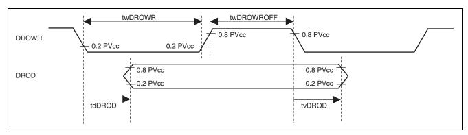
Figure 38.37 Strobe Polarity with "L" Active Selected
