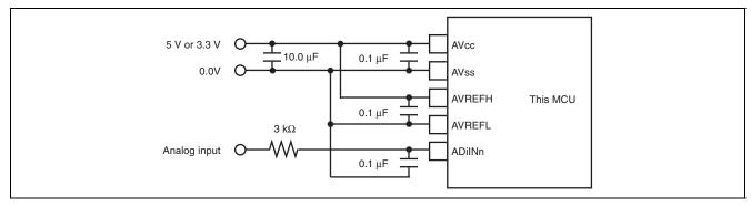
Figure 27.12 Example of Protection Circuit for Analog Input Pin
