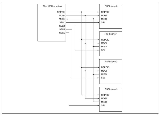
Figure 24.6 Single-Master/Multi-Slave Configuration Example (This MCU = Master)
