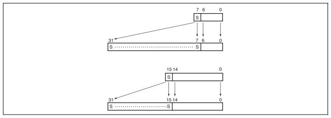
Figure 2.6 Formats of Byte Data and Word Data in Register
