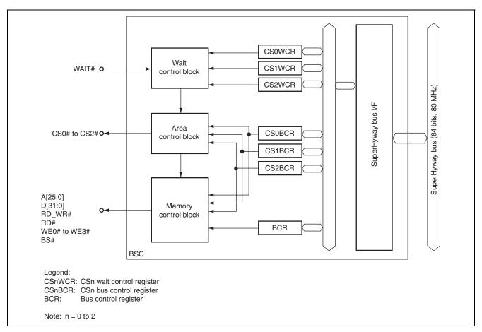
Figure 19.1 Block Diagram of BSC
