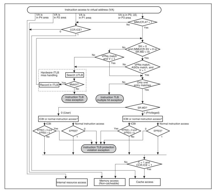
Figure 7.15 is a flowchart of memory access using the ITLB in TLB extended mode.
