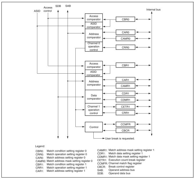
Figure 35.1 Block Diagram of UBC
