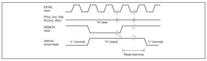
Figure 16.3 Reset During MCU Operation
