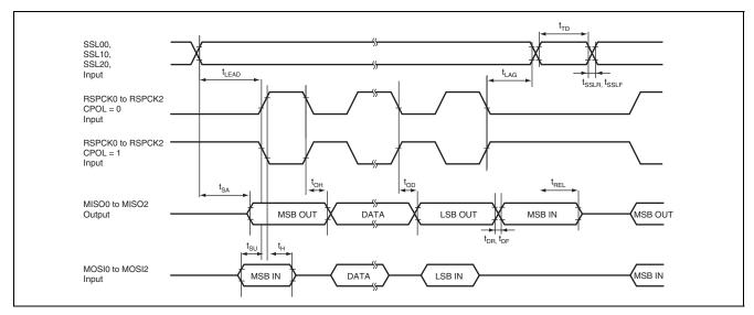
Figure 38.30 RSPI Timing (Slave, CPHA = "0")
