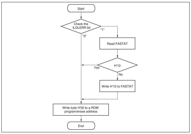
Figure 12.13 Procedure for Clearing Status Register 0
