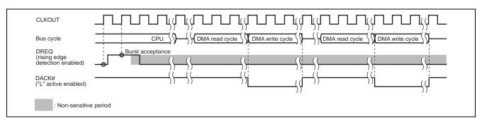
Figure 20.15 Example of DREQ Input Detection (Burst mode, DACK Write Cycle Output)
