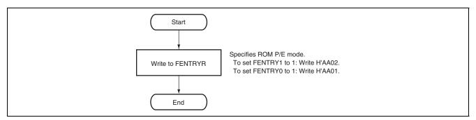
Figure 12.9 Procedure for Transition to ROM P/E Mode
