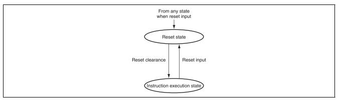
**Figure 2.8 Processing State Transitions**
