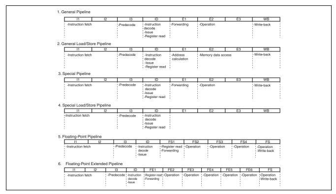
Figure 4.1 Basic Pipelines
