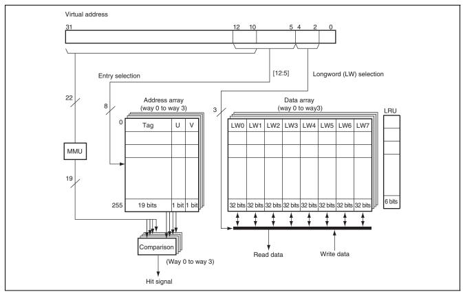
Figure 8.1 Configuration of Operand Cache (Cache size = 32 Kbytes)
