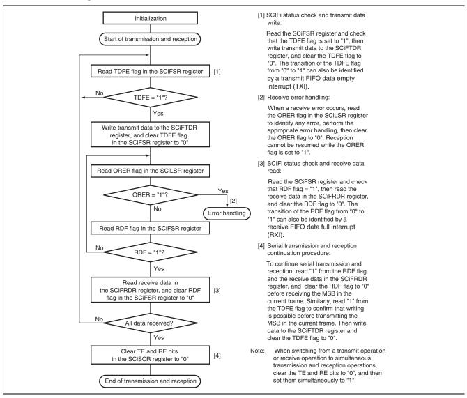
Figure 23.18 Sample Flowchart for Transmitting/Receiving Serial Data
