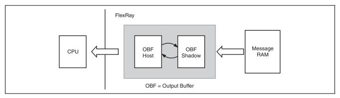
Figure 32.14 Double Buffer Structure Output Buffer
