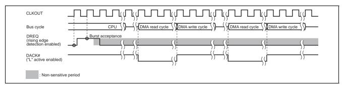
Figure 20.14 Example of DREQ Input Detection (Burst mode, DACK Read Cycle Output)
