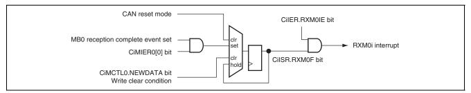
Figure 26.21 Block Diagram of CANi Reception Complete Interrupt (Mailbox 0) [RXM0i]
