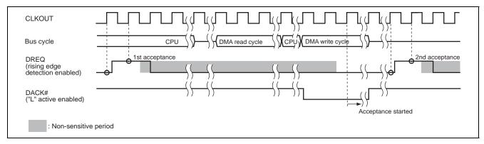
Figure 20.13 Example of DREQ Input Detection (Cycle Steal Mode 2, DACK Write Cycle Output)
