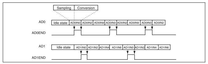
Figure 27.10 Example of AD0END and AD1END Outputs
