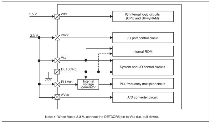
Figure 34.3 Power Supply Circuit Structure (when PVcc = Vcc = 3.3 V)
