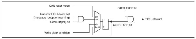
Figure 26.25 Block Diagram of CANi Transmit FIFO Interrrupt [TXFi]
