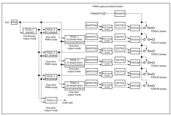
Figure 21.49 Timer Configuration Diagram
