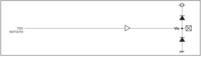
Figure 18.12 Port Peripheral Circuit Diagram (Output Port 1)
