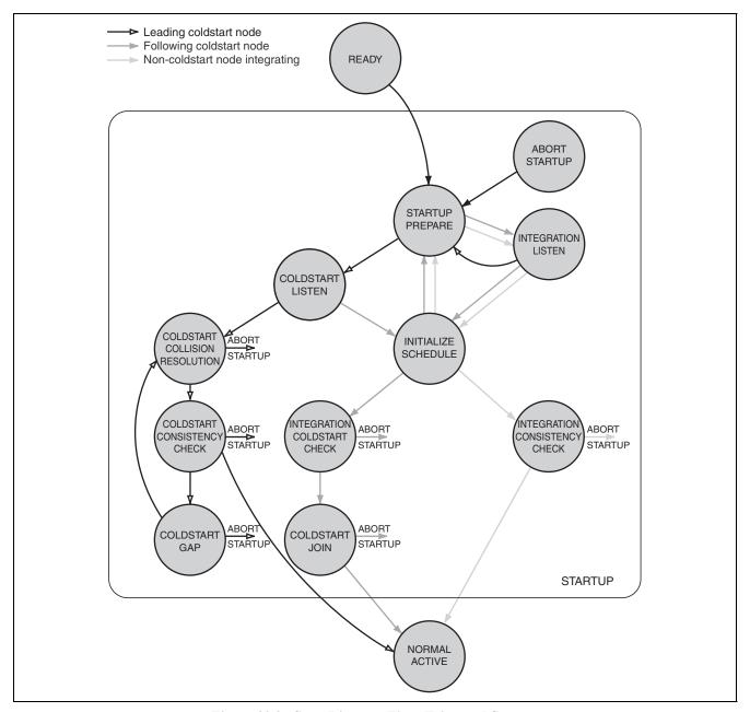
Figure 32.9 State Diagram Time-Triggered Startup
