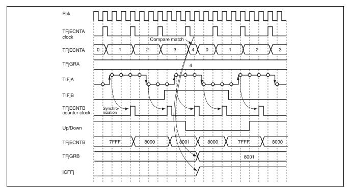
Figure 21.21 Operation Example of Up/Down Event Count
