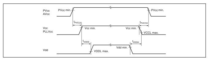
Figure 38.4 Power-On/Off Timing
