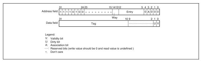
Figure 8.7 Memory-Mapped OC Address Array (Cache size = 32 Kbytes)
