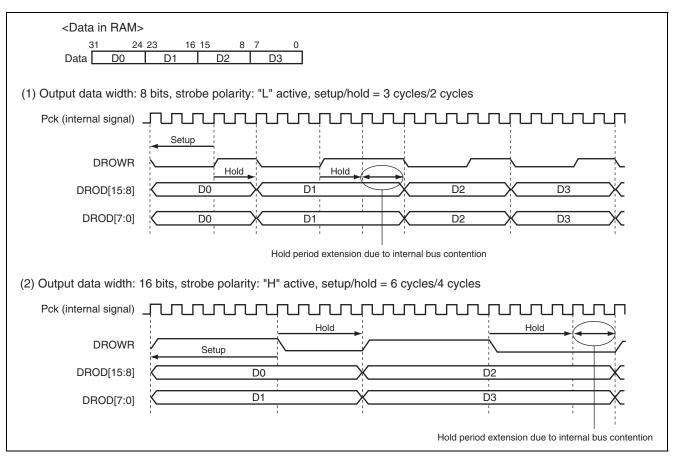
Figure 29.5 Data Format Example for Nonperiodic Output
