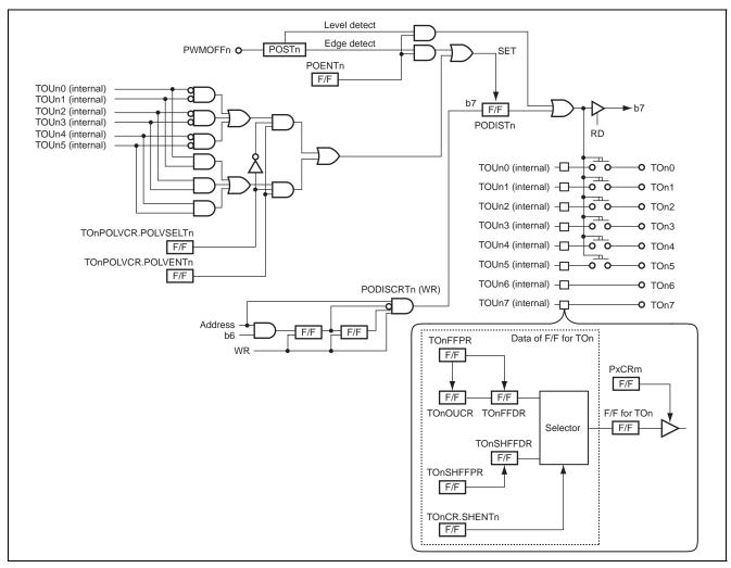
Figure 21.43 Circuit Configuration of PWM Output-Prohibit Function
