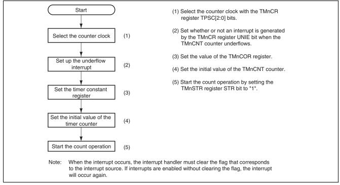
Figure 22.2 Example of Count Operation Setting Procedure
