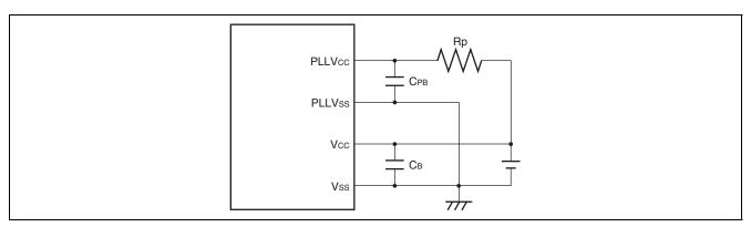
Figure 14.6 PLL Frequency Multiplier Circuit Power Supply Connection Notes
