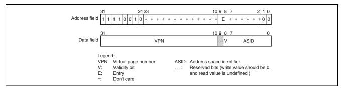
Figure 7.18 Memory-Mapped ITLB Address Array
