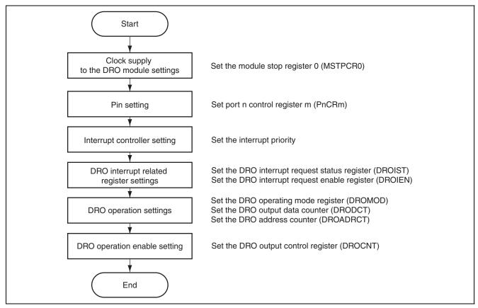
Figure 29.3 DRO Setup Example
