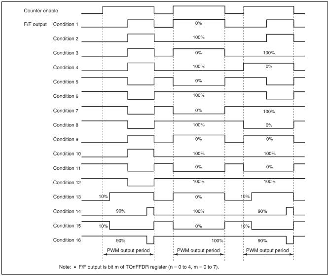
Figure 21.42 Example of F/F Output with 0% or 100% Duty Cycle in One-Shot PWM Output Mode
