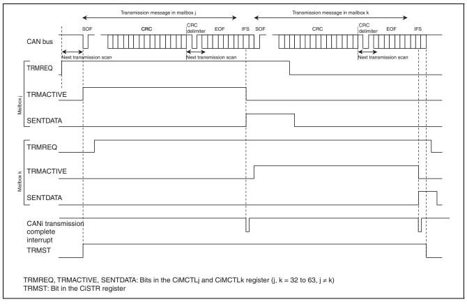
Figure 26.20 Operation Example of Data Frame Transmission (i = 0 to 4)
