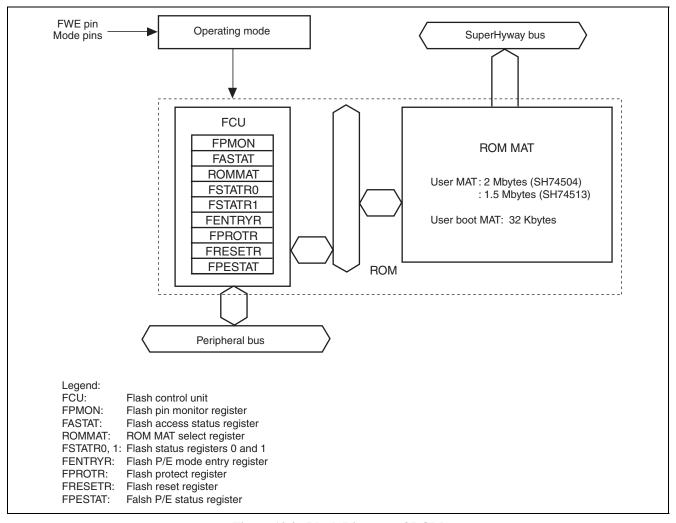
Figure 12.2 Block Diagram of ROM
