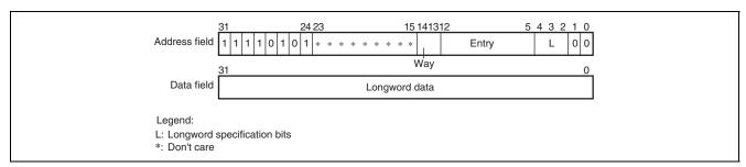
Figure 8.8 Memory-Mapped OC Data Array (Cache size = 32 Kbytes)
