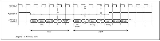
Figure 36.5 Read Operation Example (byte read)
