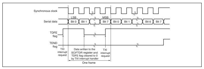
Figure 23.14 Example of SCIFi Transmit Operation
