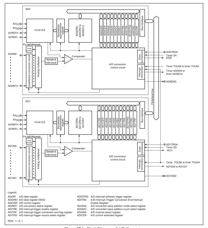
Figure 27.1 shows a block diagram of the A/D converter.
