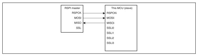
Figure 24.10 Master (Clock-Synchronous Operation)/Slave (Clock-Synchronous Operation) Configuration Example (This MCU = Slave, CPHA = "1")
