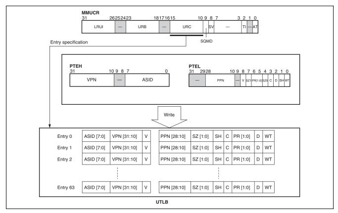
Figure 7.16 Operation of LDTLB Instruction (TLB Compatible Mode)
