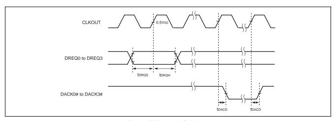
Figure 38.20 DMAC Timing
