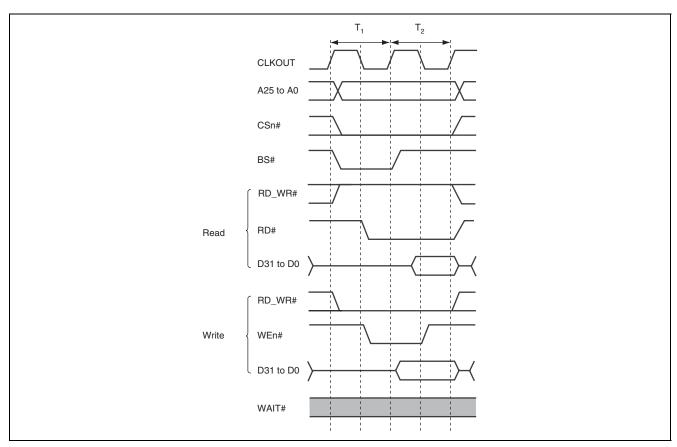
Figure 19.3 Basic Timing of SRAM Interface (No Wait)
