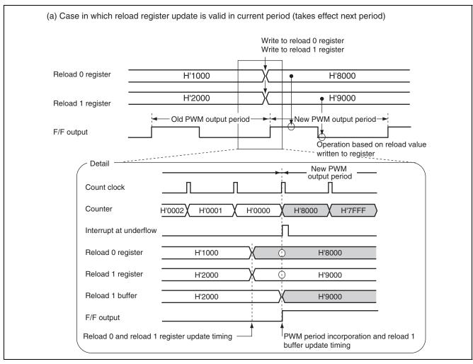
Figure 21.30 Reload 0 and Reload 1 Register Updating in PWM Output Mode
