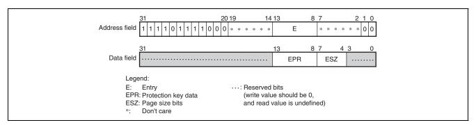
Figure 7.25 Memory-Mapped UTLB Data Array 2 (TLB Extended Mode)
