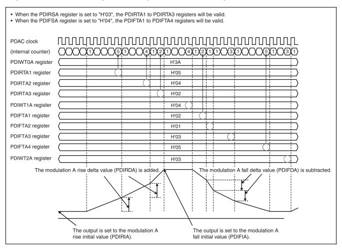
Figure 30.16 Modulation Waveform Output Timing (Example: Modulation A)
