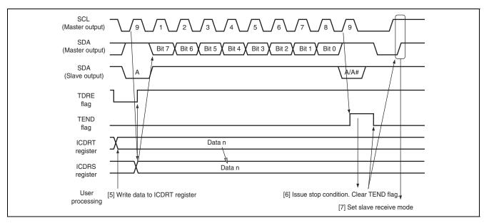
Figure 25.6 Master Transmit Mode Operation Timing (2)
