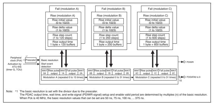
Figure 30.1 Block Diagram of PDAC
