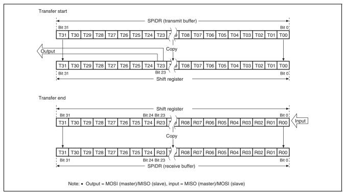
Figure 24.14 MSB First Transfer (24-Bit Data)
