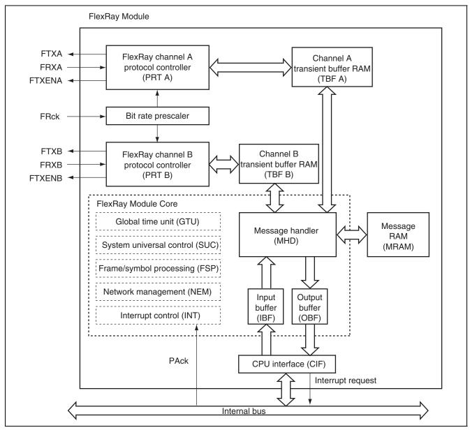
Figure 32.1 Block Diagram of FlexRay Module
