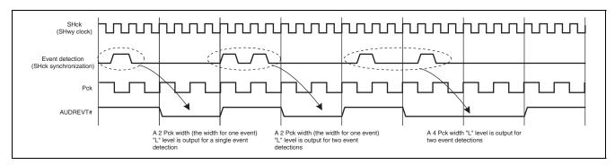
Figure 36.8 AUDR Event Detection and AUDREVT# Pin Operation
