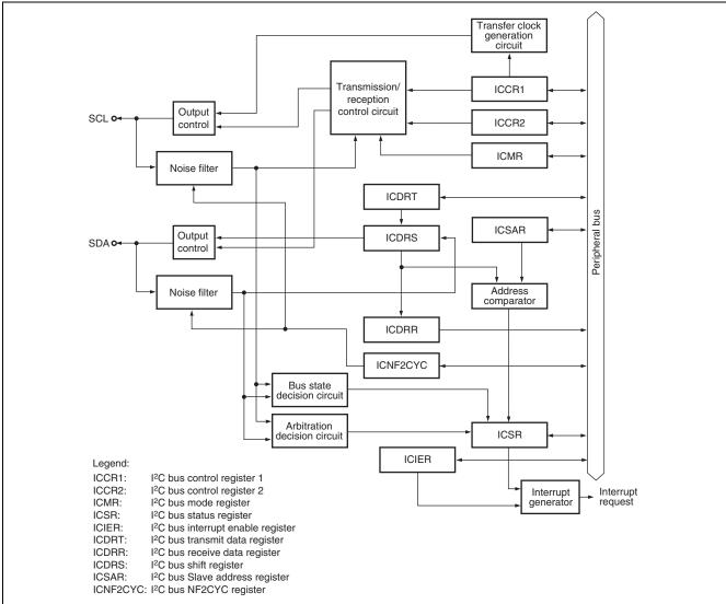
Figure 25.1 Block Diagram of I<sup>2</sup>C Bus Interface 3
