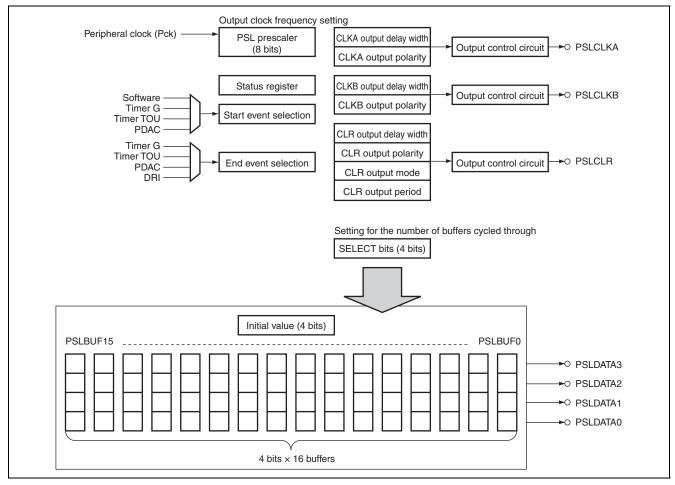
Figure 31.1 Block Diagram of PSEL
