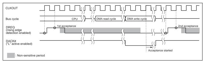
Figure 20.11 Example of DREQ Input Detection (Cycle Steal Mode 1, DACK Write Cycle Output)
