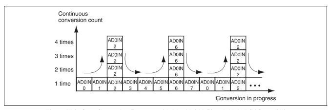
Figure 27.2 Scan Conversion Sequence with Bits AD0ADS2 and AD0ADS6 Set to "1"
