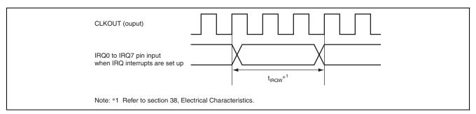
Figure 15.10 Time Requested to Detect Interrupts from IRQ
