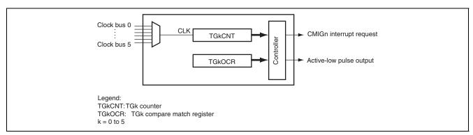
Figure 21.23 Block Diagram of Timer G
