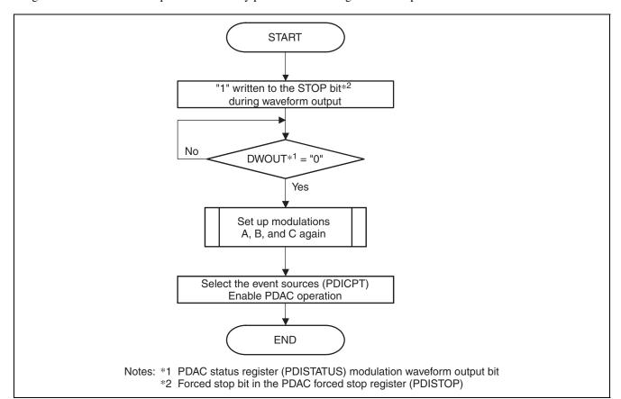
Figure 30.15 shows an example of the recovery procedure following a forced stop.
