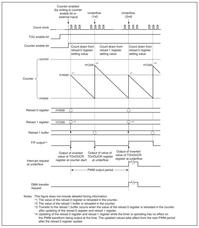
Figure 21.28 Operation Example of PWM Output Mode
