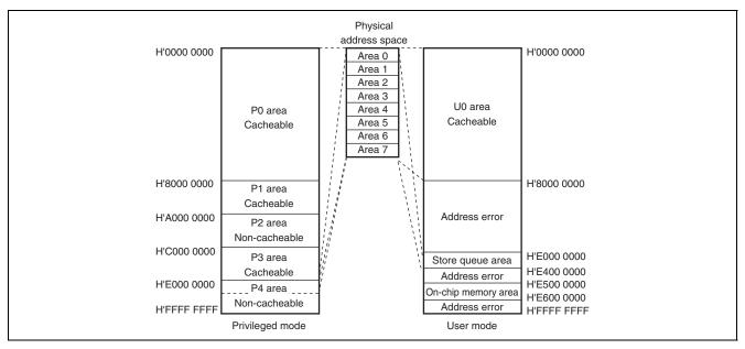
Figure 7.2 Virtual Address Space (AT in MMUCR = 0)
