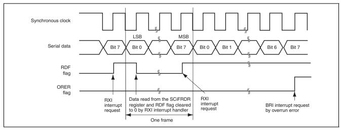
Figure 23.17 Example of SCIFi Receive Operation
