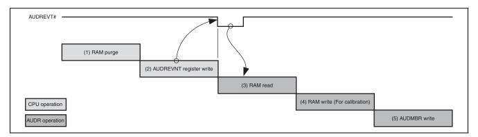
Figure 36.2 AUDR Module Usage Example (RAM monitor/calibration procedure)
