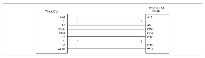
Figure 19.6 Example of 8-Bit Data-Width SRAM Connection
