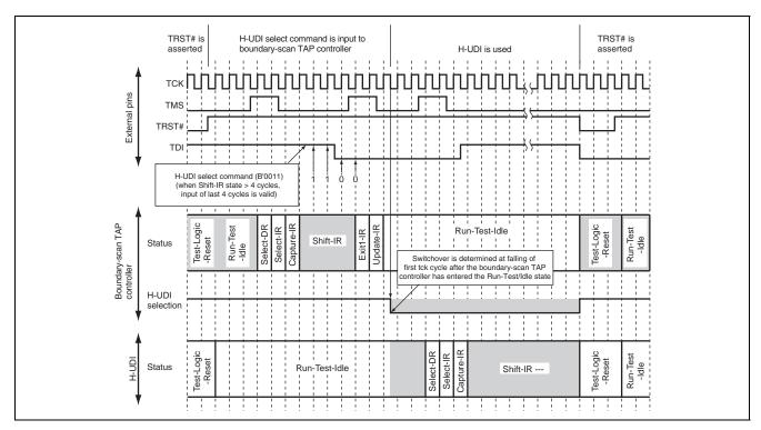
Figure 37.2 Sequence for Switching from Boundary-Scan TAP Controller to H-UDI
