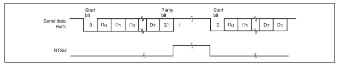
Figure 23.10 Example of Operation Using Modem Control (RTSi#)
