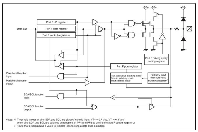
Figure 18.3 Port Peripheral Circuit Diagram (Input/Output Ports 3)
