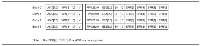
Figure 7.13 ITLB Configuration (TLB Extended Mode)
