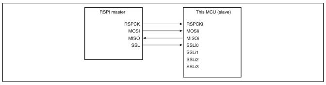
Figure 24.4 Single-Master/Single-Slave Configuration Example (This MCU = Slave)
