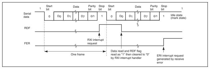
Figure 23.9 Example of SCIFi Receive Operation (8-Bit Data, Parity, 1 Stop Bit)
