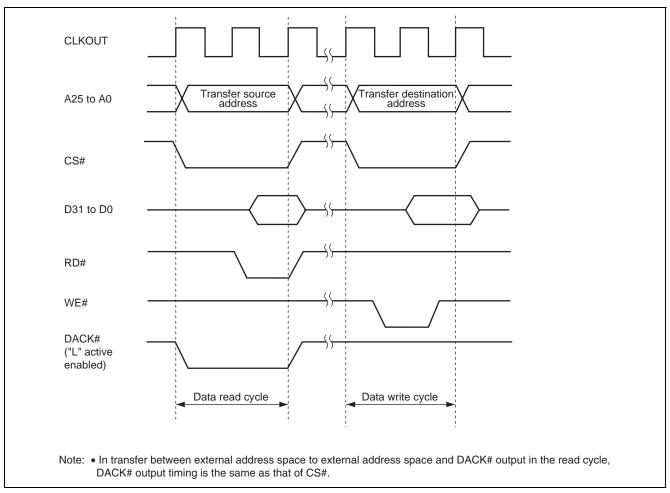
Figure 20.16 Example of DACK# Signal Output Timing (Source: External Address Space; Destination: External Address Space)
