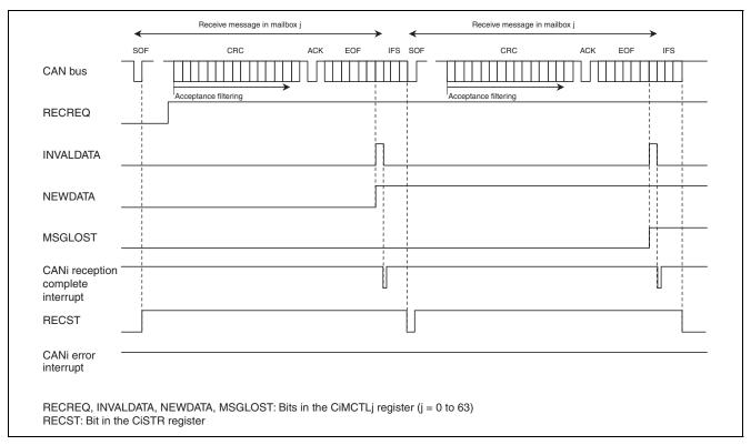
Figure 26.18 Operation Example of Data Frame Reception in Overwrite Mode (i = 0 to 4)
