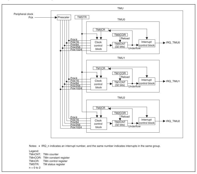
Figure 22.1 Block Diagram of TMU
