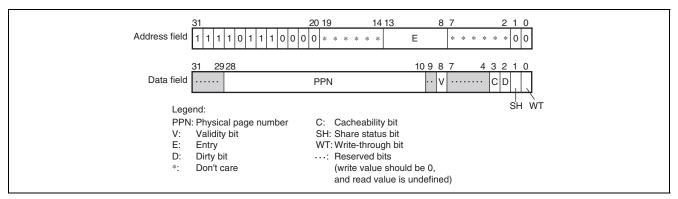
Figure 7.24 Memory-Mapped UTLB Data Array 1 (TLB Extended Mode)
