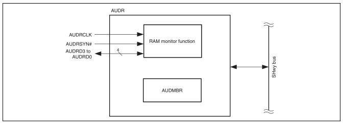
Figure 36.10 Synchronous Communication (AUDR message board register) Block Diagram
