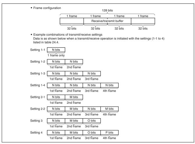
Figure 24.2 Frame Configurations and Example Combinations of Transmit/Receive Settings
