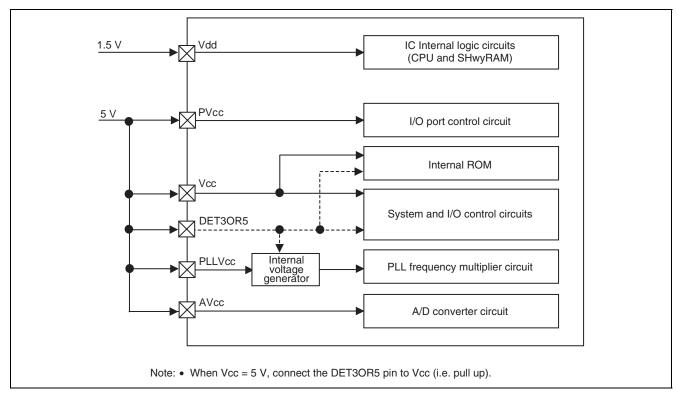
Figure 34.1 Power Supply Circuit Structure (when PVcc = Vcc = 5 V)
