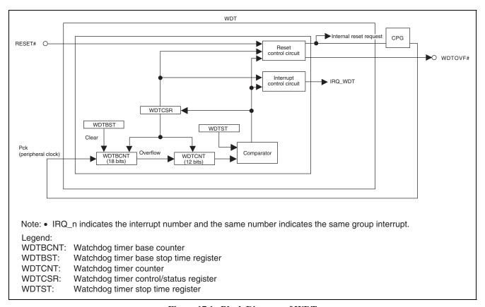
Figure 17.1 Block Diagram of WDT
