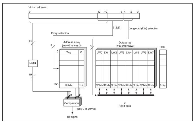
Figure 8.2 Configuration of Instruction Cache (Cache size = 32 Kbytes)
