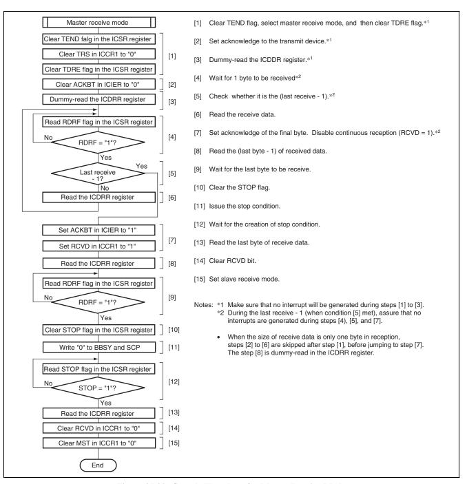
Figure 25.20 Sample Flowchart for Master Receive Mode
