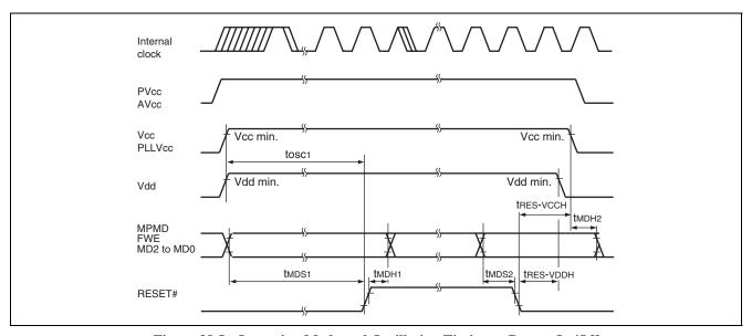
Figure 38.5 Operation Mode and Oscillation Timing at Power-On/Off
