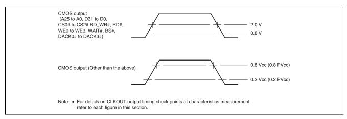
Figure 38.3 Output Timing Check Points at Characteristics Measurement
