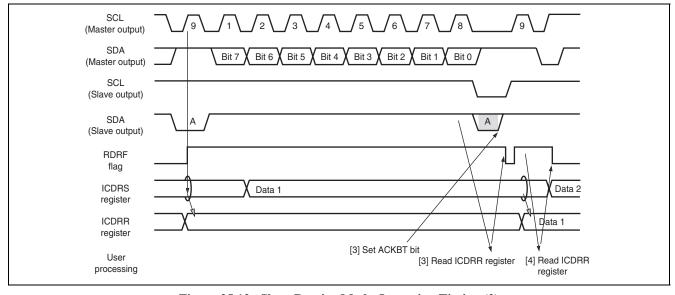
Figure 25.12 Slave Receive Mode Operation Timing (2)
