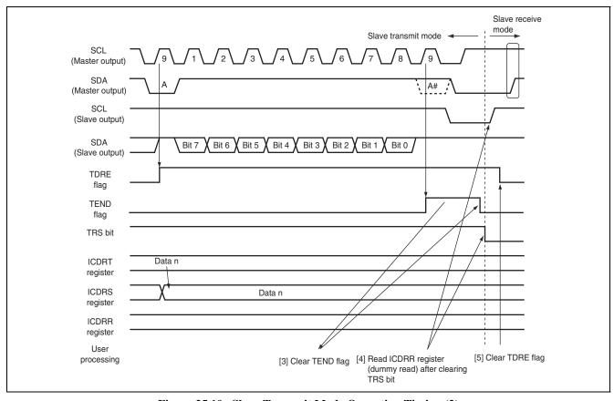
Figure 25.10 Slave Transmit Mode Operation Timing (2)
