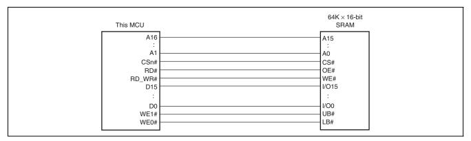
Figure 19.11 16-Bit Data Width Byte Control SRAM Connection Example
