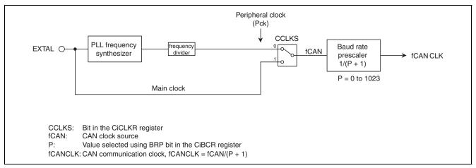
Figure 26.11 Block Diagram of CAN Clock Generator (i = 0 to 4)
