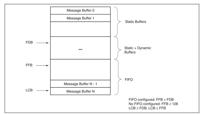
Figure 32.3 shows an example of the message buffer structure configured by bits FDB, FFB, and LCB.
