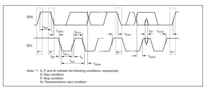
Figure 38.32 IIC3 Module Input/Output Timing
