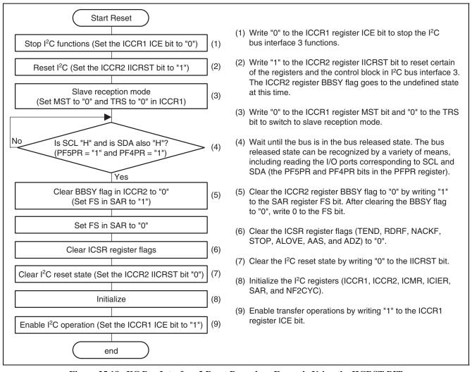
Figure 25.18 I<sup>2</sup>C Bus Interface 3 Reset Procedure Example Using the IICRST BIT
