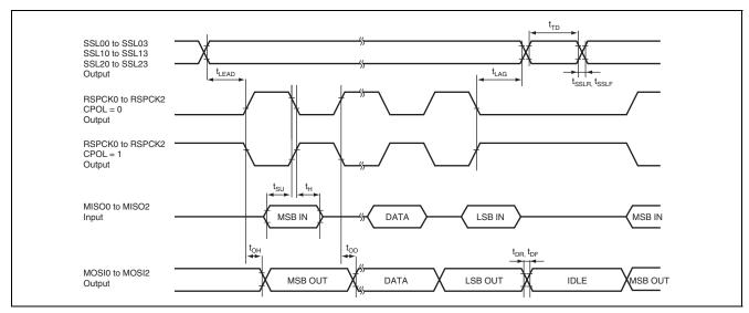
Figure 38.29 RSPI Timing (Master, CPHA = "1")
