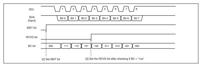
Figure 25.16 Operation Timing For Receiving One Byte (MST = "1")
