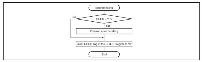
Figure 23.16 Sample Flowchart for Receiving Serial Data (2)
