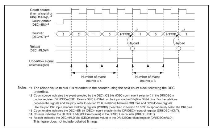
Figure 28.10 DEC Continuous Mode Count Example
