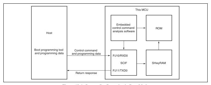
Figure 12.6 System Configuration in Boot Mode
