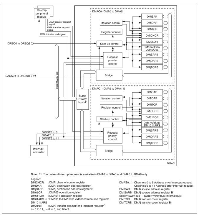
Figure 20.1 Block Diagram of DMAC
