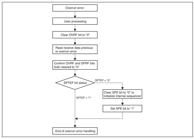
Figure 24.31 Error Handling (Overrun Error)
