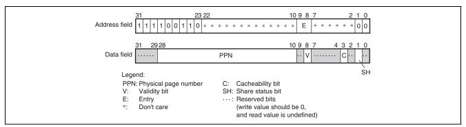
Figure 7.20 Memory-Mapped ITLB Data Array 1 (TLB Extended Mode)
