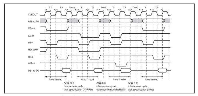
Figure 19.15 Inter-Access Cycle Wait Insertion
