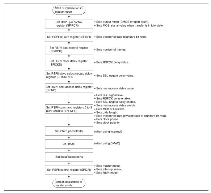
Figure 24.21 Example of Initialization Flowchart in Master Mode
