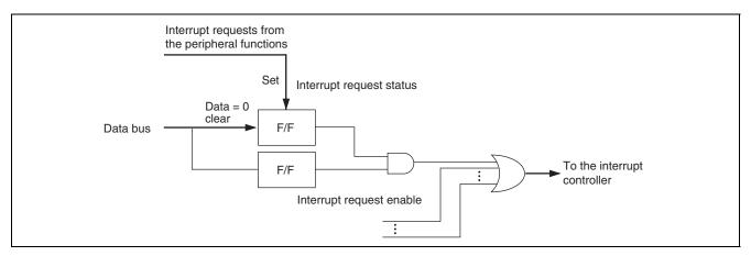
Figure 28.2 Interrupt Request Status Register and Interrupt Request Enable Register
