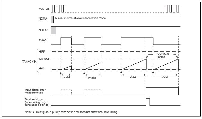
Figure 21.4 Operation of Noise Canceler in Minimum-Time-at Level Cancellation Mode
