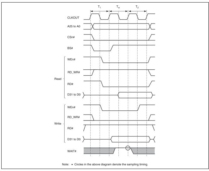
Figure 19.13 Byte Control SRAM Basic Access Timing (One Internal Wait Cycle)
