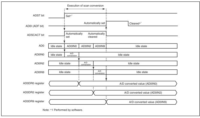
Figure 27.4 Example Operation in Single-Cycle Scan Mode
