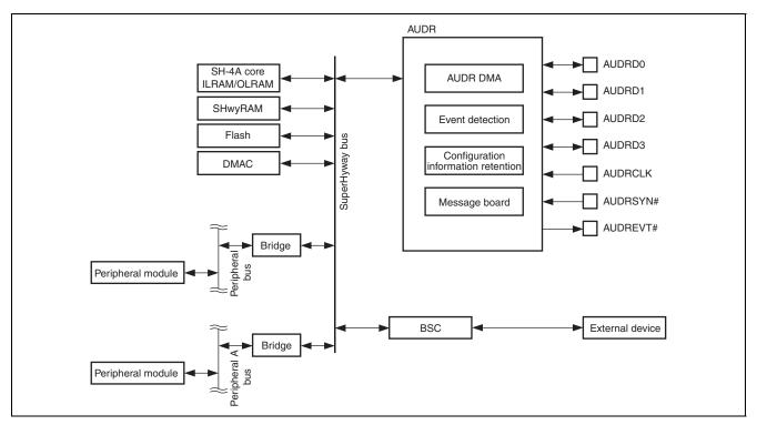
Figure 36.1 Block Diagram of AUDR
