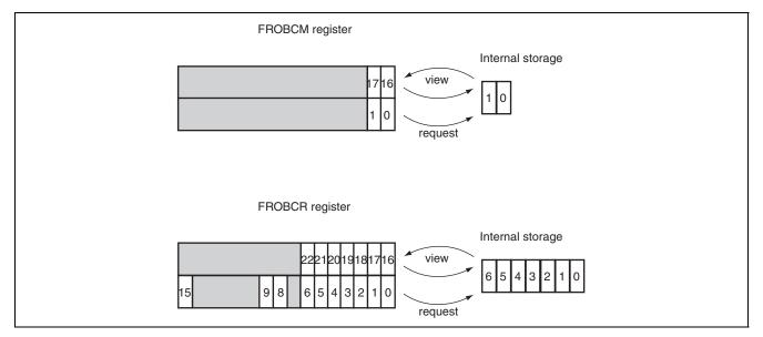
Figure 32.15 Swapping of Bits in Registers FROBCM and FROBCR
