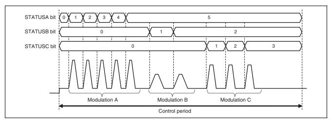
Figure 30.8 Modulation Status Information Within the PDAC Control Period
