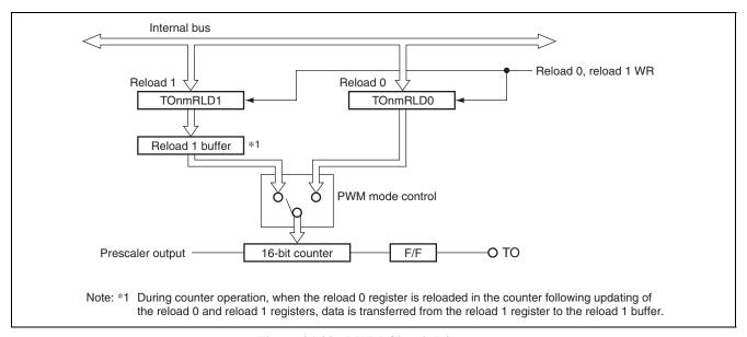
Figure 21.29 PWM Circuit Diagram
