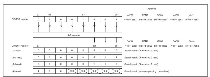
Figure 26.4 shows the write and read of registers CiCSSR and CiMSSR.
