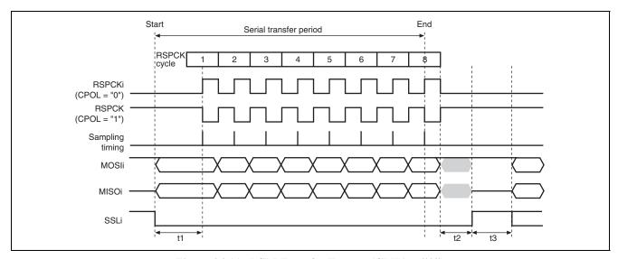
Figure 24.11 RSPI Transfer Format (CPHA = "0")
