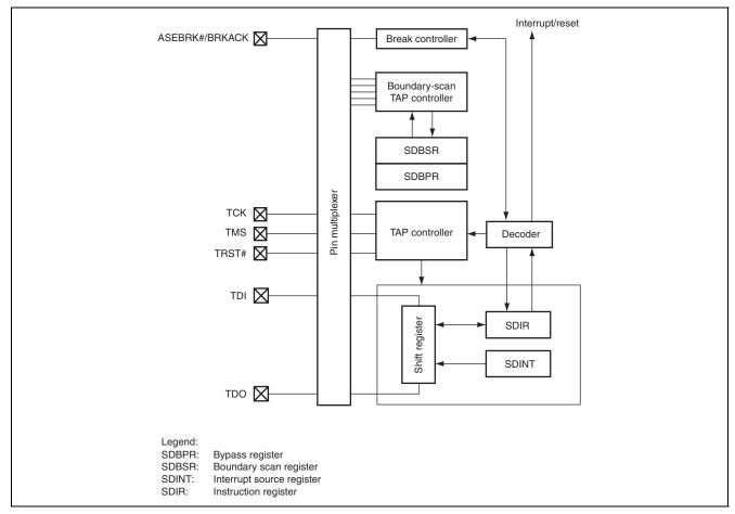
Figure 37.1 Block Diagram of H-UDI
