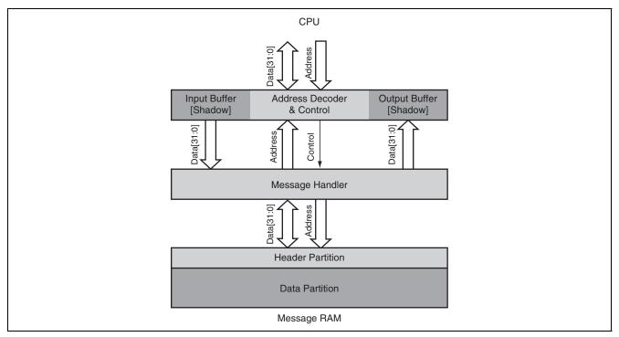
Figure 32.11 CPU Access to Message RAM
