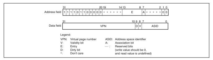
Figure 7.22 Memory-Mapped UTLB Address Array
