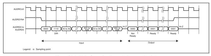
Figure 36.6 Write Operation Example (long word write)
