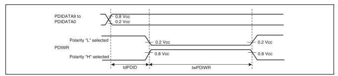
Figure 38.39 PDAC Output Timing
