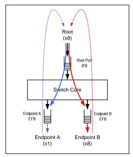
Figure 4.3 PCI Express Switch Static Rate Mismatch
