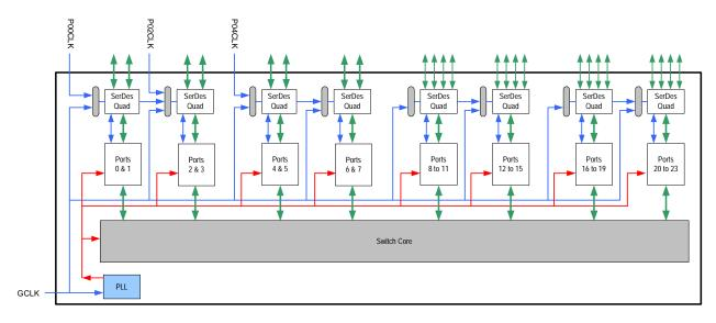
Figure 2.2 Logical Representation of PES32NT24BG2 Clocking Architecture
