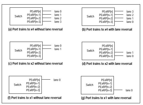
Figure 7.2 Lane Reversal for Highest Achievable Link Width of x4
