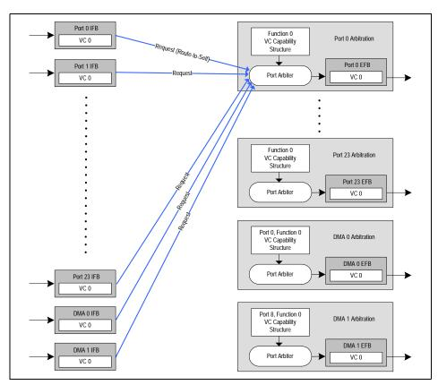
Figure 4.2 Architectural Model of Arbitration
