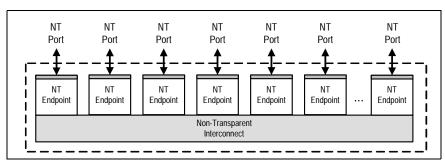
Figure 1.10 Non-Transparent Switch with Non-Transparent Ports
