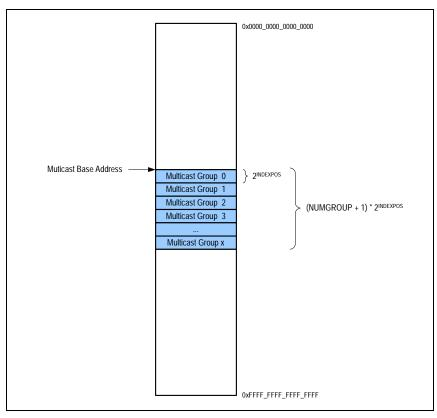
Figure 17.1 Multicast Group Address Ranges
