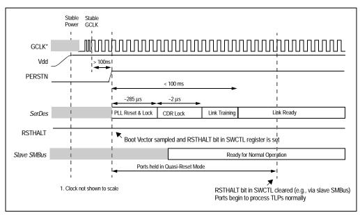
Figure 3.2 Fundamental Reset Using RSTHALT to Keep Device in Quasi-Reset State
