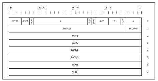
Figure 15.10 Immediate Data Transfer DMA Descriptor Format
