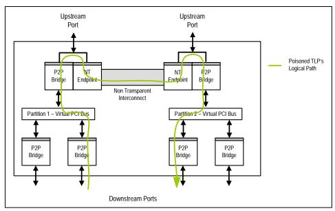
Figure 14.16 Poisoned TLP Error Propagation Example
