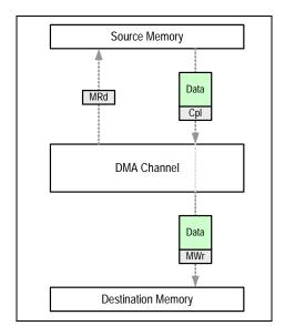
Figure 15.1 DMA Data Transfer
