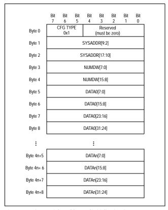
Figure 12.3 Sequential Double-word Initialization Sequence Format
