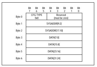
Figure 12.2 Single Double-word Initialization Sequence Format
