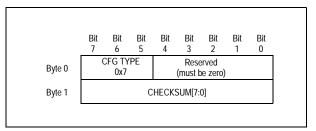
Figure 12.8 Configuration Done Sequence Format
