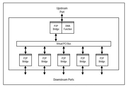
Figure 1.12 Switch Partition with DMA function
