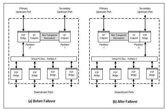
Figure 1.15 Non-Transparent Switch Failover Usage
