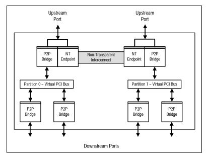
Figure 14.13 Basic Non-Transparent PES32NT24xG2 Configuration
