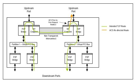
Figure 14.12 Example of ACS Peer-to-Peer Request Re-direct Applied by the NT Function
