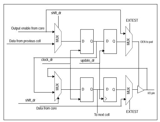
Figure 25.5 Diagram of Bidirectional Cell
