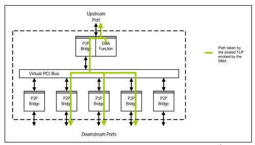
Figure 15.12 Path Taken by a TLP Emitted by the DMA When it is Multicasted<sup>1</sup>
