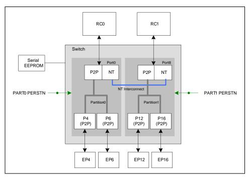
Figure 26.14 Active/Active System Configuration Before Failover Event
