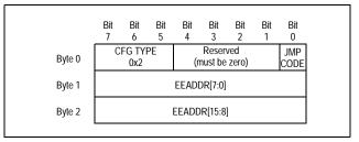
Figure 12.4 Jump Configuration Block
