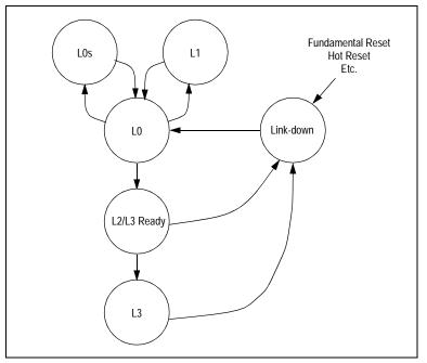
Figure 7.4 PES32NT24xG2 ASPM Link State Transitions
