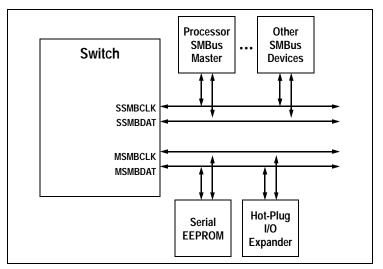
Figure 12.1 Split SMBus Interface Configuration
