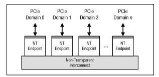
Figure 1.6 Generalized Multi-Port Non-Transparent Interconnect
