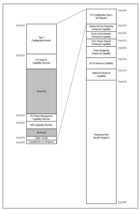
Figure 19.1 PCI-to-PCI Bridge Configuration Space Organization
