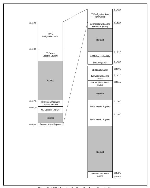
Figure 19.4 DMA Function Configuration Space Organization
