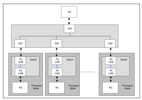
Figure 26.10 System Configuration Immediately after Switch Fundamental Reset
