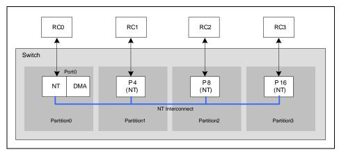
Figure 26.19 PES32NT24xG2 with Port 0 Configured in NT Function with DMA Mode and Ports 4, 8, and 16 in NT Function Mode
