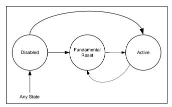
Figure 5.1 Allowable Partition State Transitions
