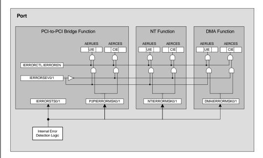
Figure 4.7 Internal Error Logic in Each PES32NT24xG2 Port
