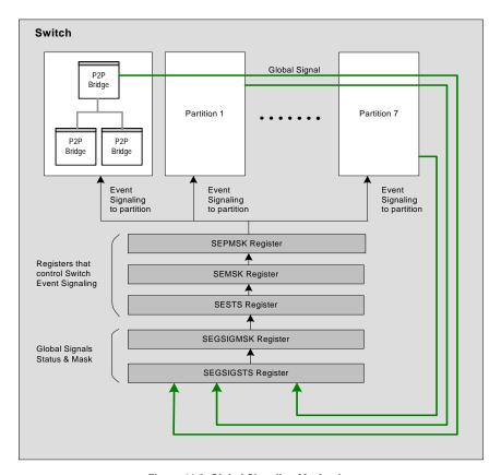
Figure 16.2 Global Signaling Mechanism
