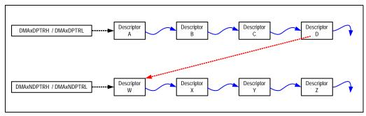
Figure 15.11 DMA Chaining Example
