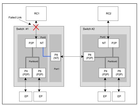
Figure 26.17 System Configuration after RC2 Modifies Port 8 in Switch #2 to Downstream Switch Port Mode in Partition 0
