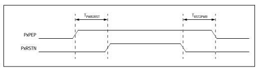
Figure 11.4 Power Enable Controlled Reset Output Mode Operation
