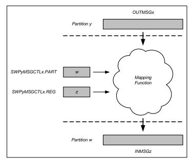
Figure 14.10 Logical Representation of Message Register Operation
