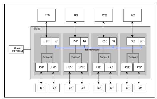
Figure 26.7 Multiprocessor System Interconnection Using the PES32NT24xG2
