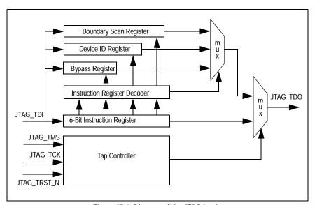
Figure 25.1 Diagram of the JTAG Logic
