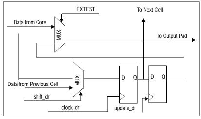
Figure 25.4 Diagram of Output Cell
