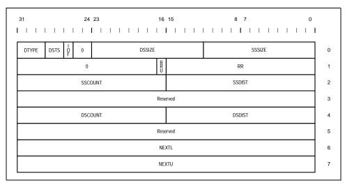
Figure 15.8 Stride Control DMA Descriptor Format
