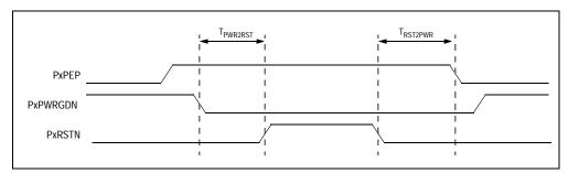
Figure 11.5 Power Good Controlled Reset Output Mode Operation
