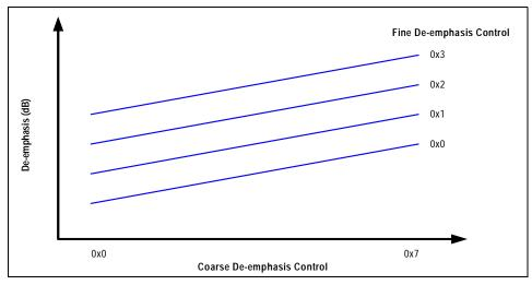
Figure 8.1 Relationship Between Coarse and Fine De-emphasis Controls
