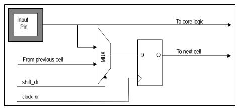
Figure 25.3 Diagram of Observe-only Input Cell
