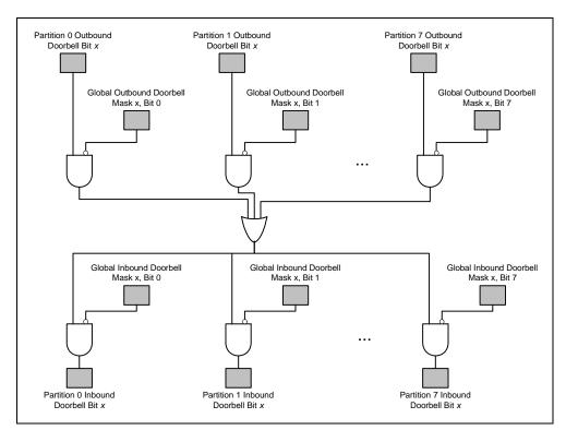
Figure 14.9 Logical Representation of Doorbell Operation
