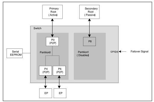
Figure 26.12 Active/Passive System Configuration Before Failover Event
