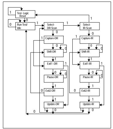
Figure 25.2 State Diagram of the TAP Controller
