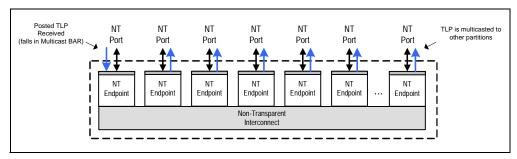
Figure 1.18 Example of Non Transparent Multicast
