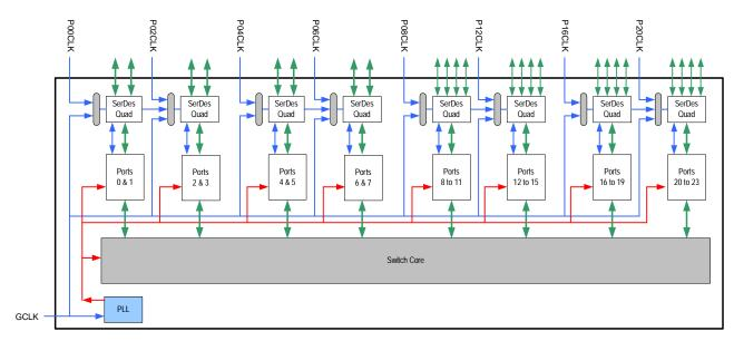
Figure 2.1 Logical Representation of PES32NT24AG2 Clocking Architecture
