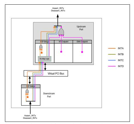
Figure 10.1 Logical Representation of INTx Aggregation
