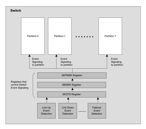
Figure 16.1 Switch Event Detection and Signaling Mechanism
