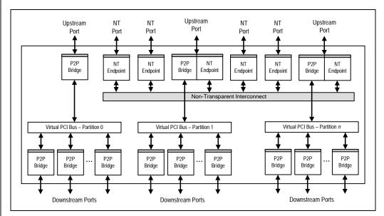
Figure 1.11 Non-Transparent Switch with Non-Transparent Ports
