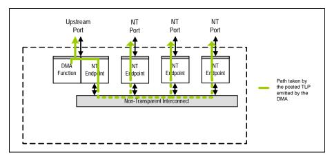
Figure 15.13 Path Taken by a TLP Emitted by the DMA When it is NT Multicasted
