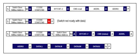
Figure 12.12 CSR Register Read Using SMBus Block Write/Read Transactions with PEC Disabled
