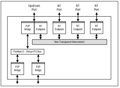
Figure 1.9 Non-Transparent Switch with Non-Transparent Ports
