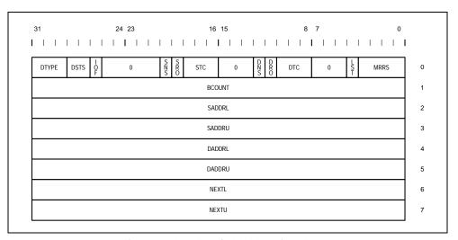
Figure 15.9 Data Transfer DMA Descriptor Format
