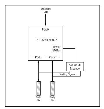
Figure 11.1 Hot-Plug on Switch Downstream Slots Application
