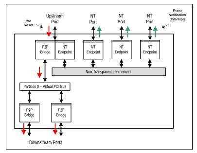
Figure 1.16 Example of Switch Event Mechanism
