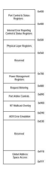
Figure 19.2 Proprietary Port Specific Register Organization
