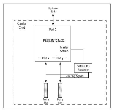
Figure 11.3 Hot-Plug with Carrier Card Application
