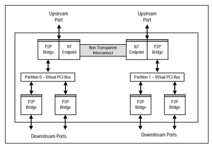
Figure 1.8 Non-Transparent Switch with Non-Transparency Between Partitions
