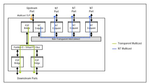
Figure 17.3 Transparent and Non-Transparent Multicast
