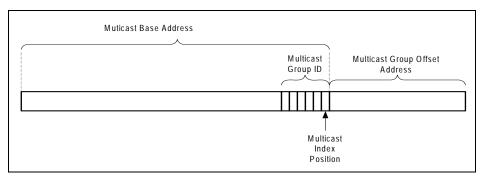
Figure 17.2 Multicast Group Address Region Determination
