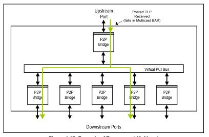
Figure 1.17 Example of Transparent Multicast
