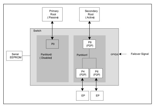
Figure 26.13 Active/Passive System Configuration after Failover Event
