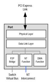
Figure 1.2 Logical Representation of a Port with PCI-to-PCI bridge, NT, and DMA Functions
