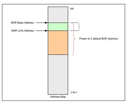
Figure 14.1 BAR Limit Operation
