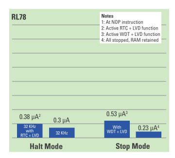
Figure 2 – RL78 Standby Current Consumption
