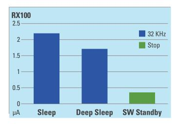
Figure 3 – RX100 Standby Current Consumption
