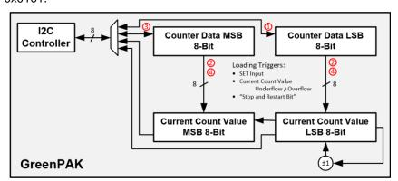
Figure 11: 16-Bit I2C Counter Block Diagram
