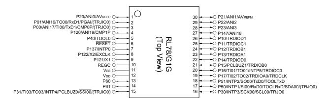
Caution Connect the REGC pin to Vss pin via a capacitor (0.47 to 1  $\mu$ F).
