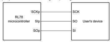
Simplified SPI (CSI) mode connection diagram (during communication at same potential) (Slave Transmission of slave select input function (CSI00))
