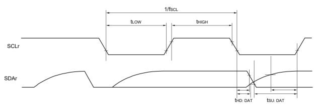
Caution Select the normal input buffer and the N-ch open drain output (VDD tolerance) mode for the SDAr pin and the normal output mode for the SCLr pin by using port input mode register g (PIMg) and port output mode register h (POMh).
