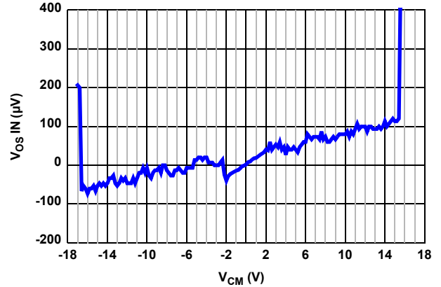
FIGURE 19. V_{OsIN} vs INPUT COMMON MODE VOLTAGE
