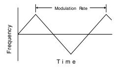
Modulation Frequency = Input Frequency/10000
