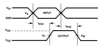
FIGURE 4. THREE-STATE HIGH TIMING DIAGRAMS
