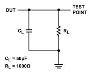
FIGURE 6. THREE-STATE HIGH LOAD CIRCUIT
