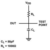
FIGURE 5. THREE-STATE LOW LOAD CIRCUIT
