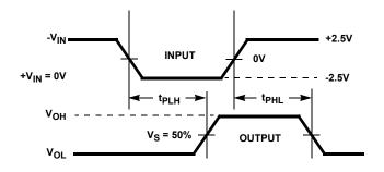
FIGURE 1. PROPAGATION DELAY TIMING DIAGRAM
