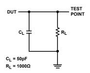
FIGURE 3. PROPAGATION DELAY LOAD CIRCUIT
