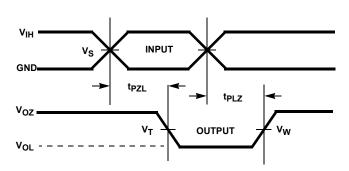
FIGURE 2. THREE-STATE LOW TIMING DIAGRAM
