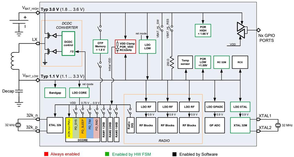
Figure 7. Power management unit: buck configuration
