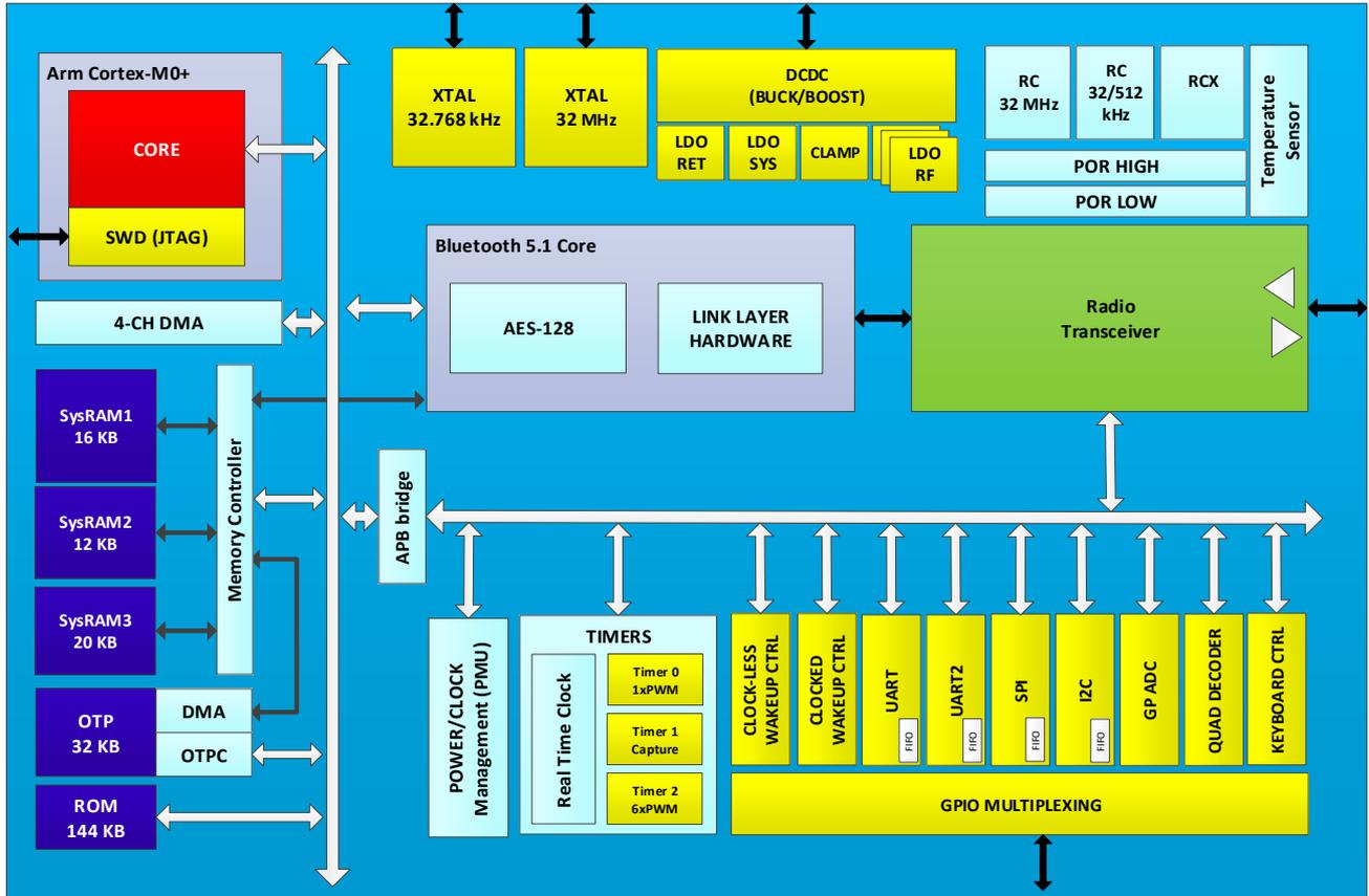
Figure 2. DA14531 block diagram
