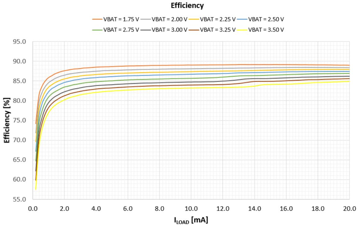
Figure 76. DCDC efficiency in buck configuration
