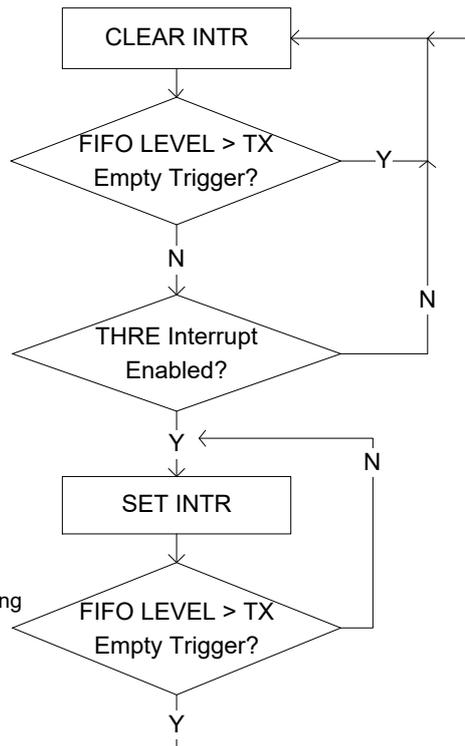
Figure 47. Flowchart of interrupt generation for programmable THRE Interrupt mode
