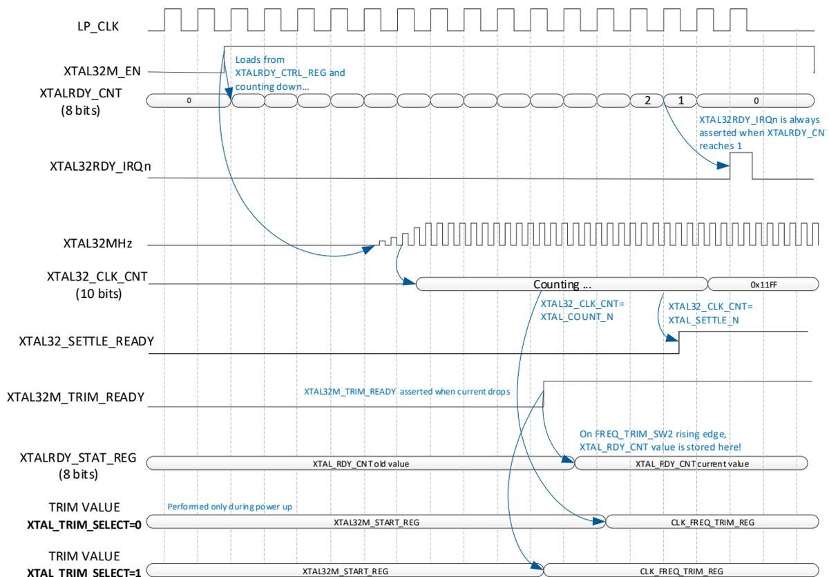
Figure 29. Automated mechanism for XTAL32M trim and settling
