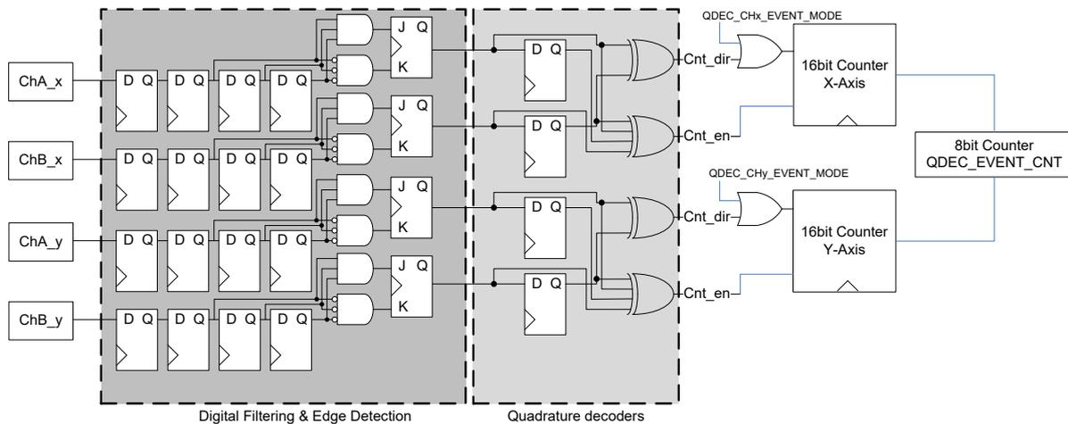
Figure 54. Digital filtering and edge detection circuit
