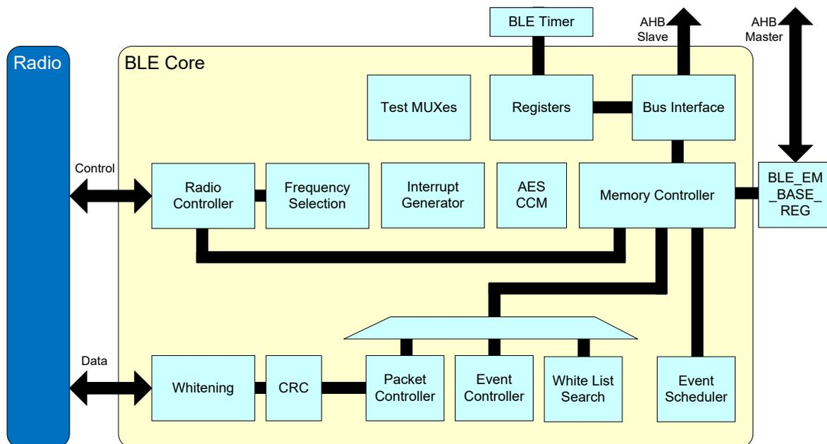
Figure 78. Bluetooth® LE core block diagram
