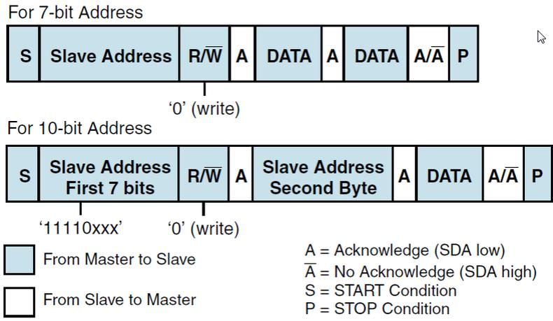
Figure 39. Master-transmitter protocol
