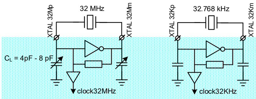
Figure 27. Crystal oscillator circuits
