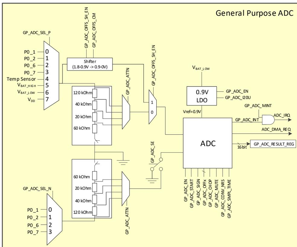
Figure 71. Block diagram of GPADC
