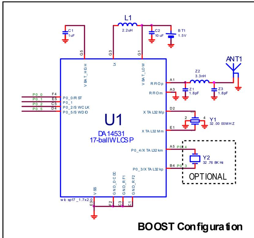
Figure 5. Boost configuration system diagram
