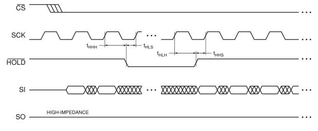
Figure 14-5. HOLD Timing – Serial Output
