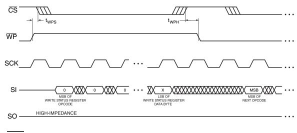
Figure 14-4. HOLD Timing – Serial Input
