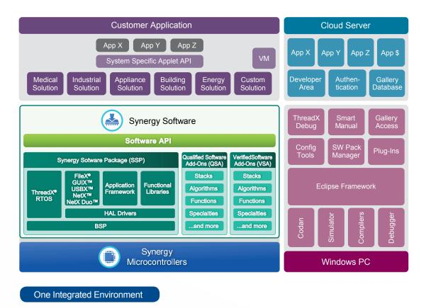
Developers use a single integrated environment comprised of the SSP, ISDE, Cloud and applications.
