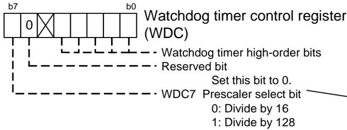
If the CSPRO bit = 1 (count source protection mode enabled), the on-chip oscillator is selected for the count source, in which case the clock frequency division by the prescaler is not performed no matter how WDC7 is set.
