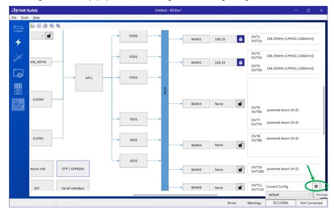
In the Configurations sub-window, configs can be renamed and more configs can be added. For this example, "default" config will be renamed to "config0". Click inside the box, delete "default", and then type in the new name, "config0".
