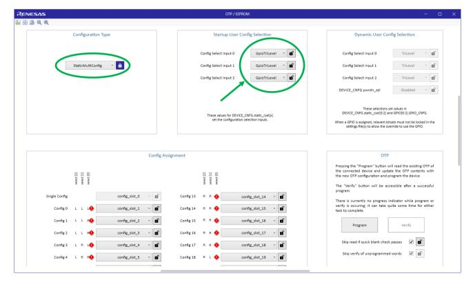
Forcing a CSEL to Low, Mid, or High will ignore the voltage state of the pin at power on. For this example, Config Select Input 1 and 2 will be set to "Low". Now only the first 3 slots need defining as these 3 slots have CSEL2 and CSEL1 set to L. Even though CSEL are set to L, they can still have other functions assigned.
