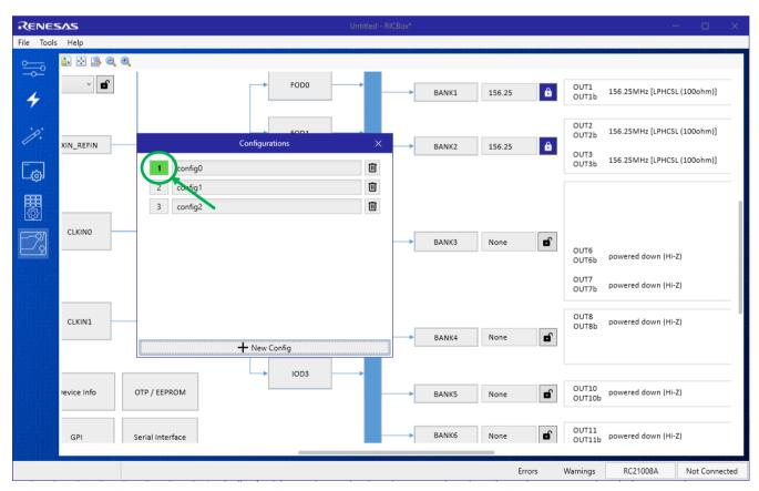
Click on the "2" to make changes and configure "config1" to meet the application needs. Do the same for "config2".
