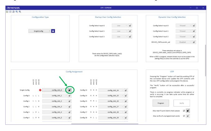
In the Configuration Type section, choose "StaticMultiConfig" from the pull-down menu. The "Startup User Config Selection" area is now enabled. By default, all Config Select input are set to "GpioTri Level". Tri Level refers to VDDD for High, VDDD/2 for Mid, and 0 for L. With 3 CSEL bits, there can be a total of 3 x 3 x 3 different configs. As a result, all config slots must be given a config.
