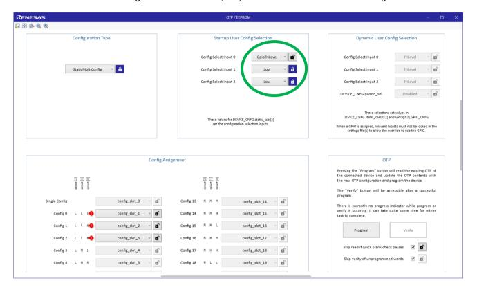
For each enabled pull-down box, select a config.
