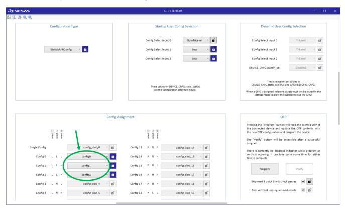
Configs may go into any slot. Also, any given config should have a more descriptive name. For example, "config0" could become "3 x 156.25MHz".
