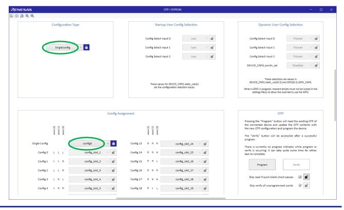
To switch over to "StaticMultiConfig", the Single Config selection must be cleared. This can be accomplished by clicking the blue lock icon. This will unlock the field back to default which is no config.
