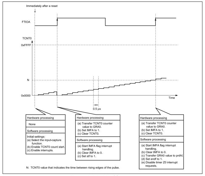
Figure 3.1 Principle of Operation
