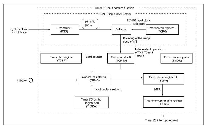
Figure 2.1 Block Diagram of Timer Z0
