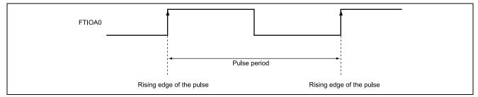
Figure 1.1 Input Pulse Period Measurement
