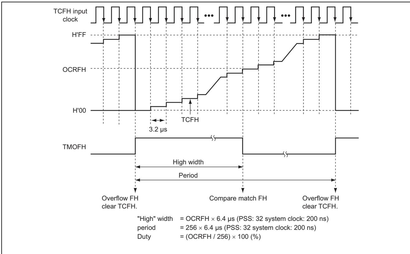
Figure 3 Method to Set Period and Duty of PWM Waveform Output
