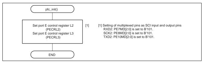
Figure 13 Flow for Setting Up the Pin Function Controller
