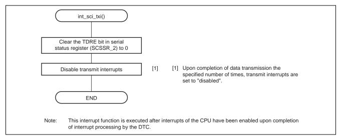
Figure 14 Flow for Handling Transmit Interrupts in Clock Synchronous Mode
