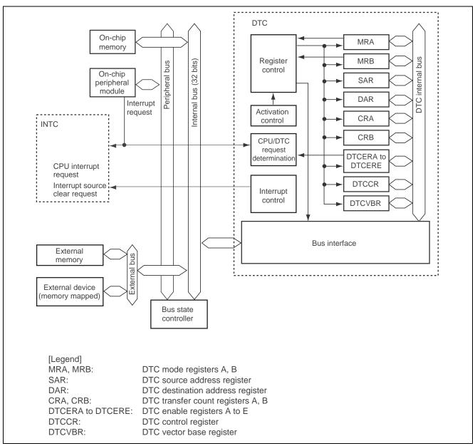
Figure 3 Block Diagram of the DTC
