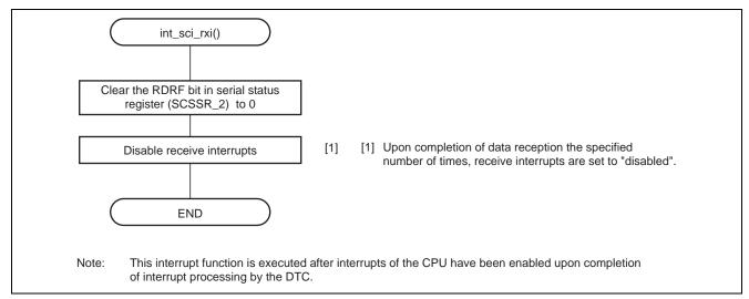
Figure 15 Flow for Handling Receive Interrupts in Clock Synchronous Mode
