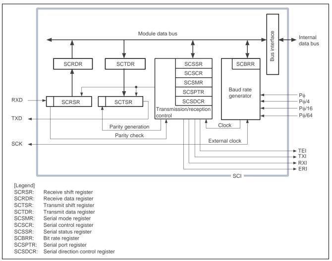
Figure 2 Block Diagram of the SCI
