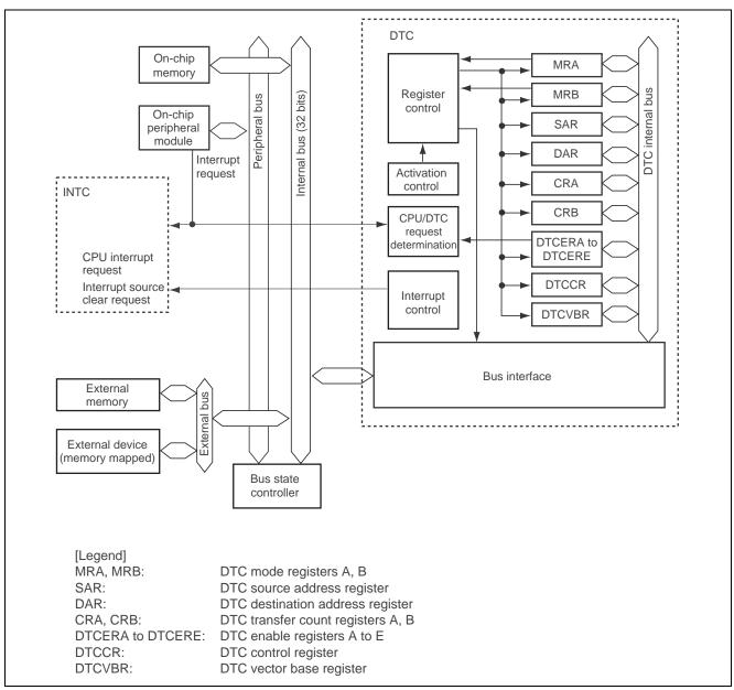
Figure 3 Block Diagram of the DTC
