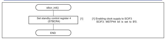
Figure 9 Flow of Setting for Release from Module-Standby Mode
