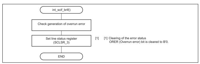
Figure 16 Flow for Handling Receive Error Interrupts in Asynchronous Mode
