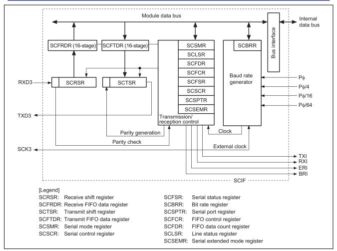
Figure 2 Block Diagram of the SCIF
