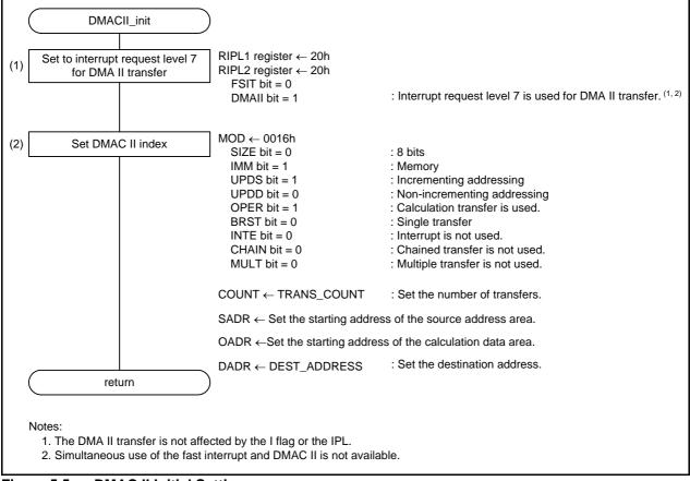
Figure 5.5 DMAC II Initial Setting
