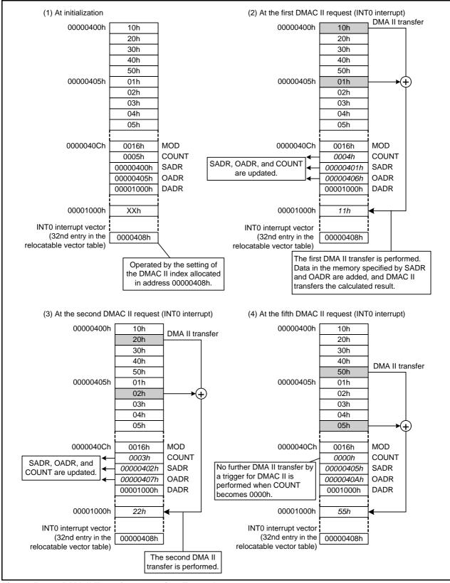
Figure 5.1 DMA II Transfer Operation Example
