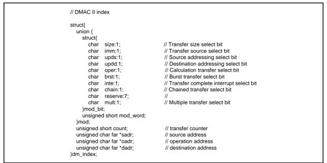
Figure 5.2 Structure/Union Used in the Sample Code
