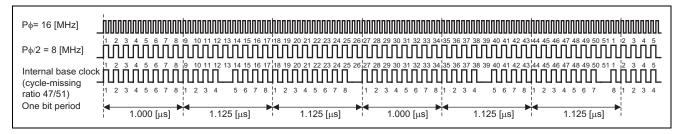
Figure 4 Example of Internal-Base-Clock Generation When  $P\phi = 16$  MHz and ACS3 to 0 = B'0011
