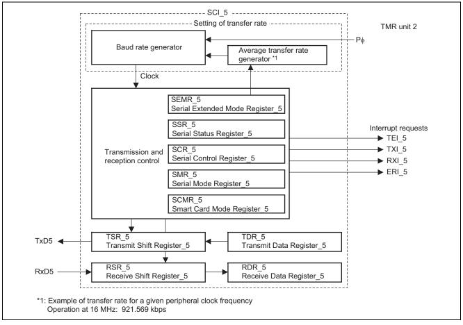
Figure 2 Block Diagram of SCI\_5
