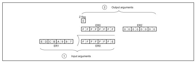
Figure 1 Example of Software DIVIDE64
