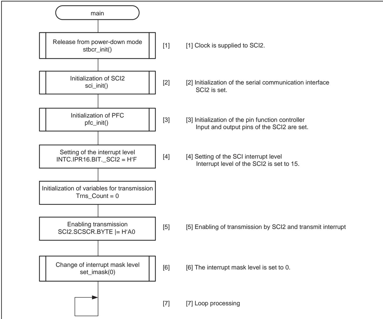
Figure 4 Flow of Processing by the Sample Task
