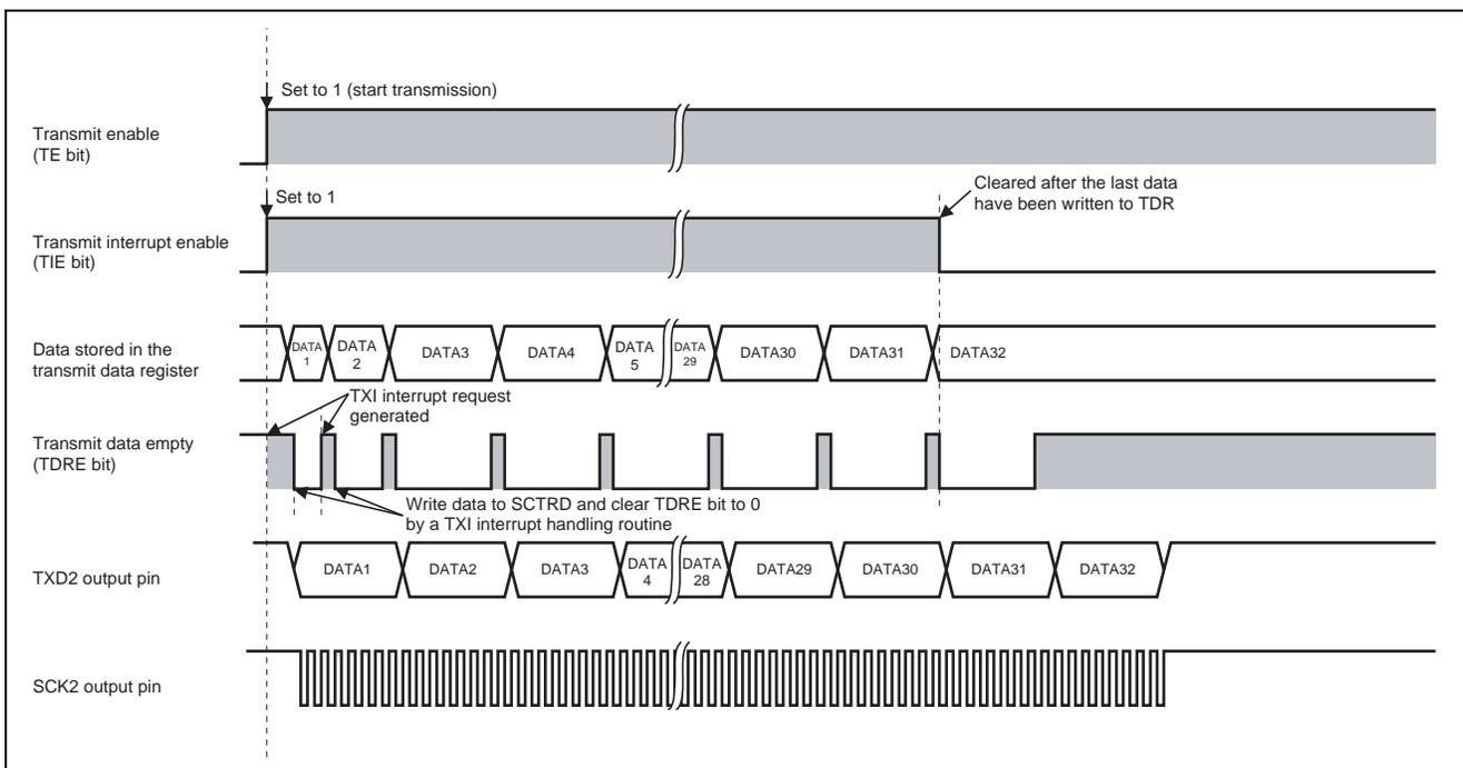
**Figure 3 Operations for Data Transmission**
