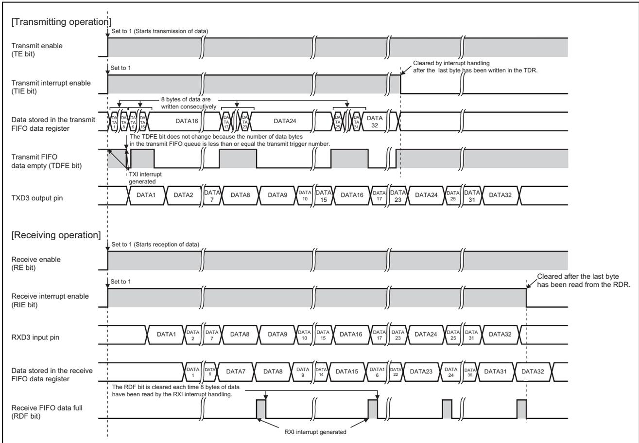
**Figure 3 Operations for Data Transmission and Reception**
