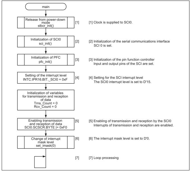
Figure 4 Flow of Processing by the Sample Program
