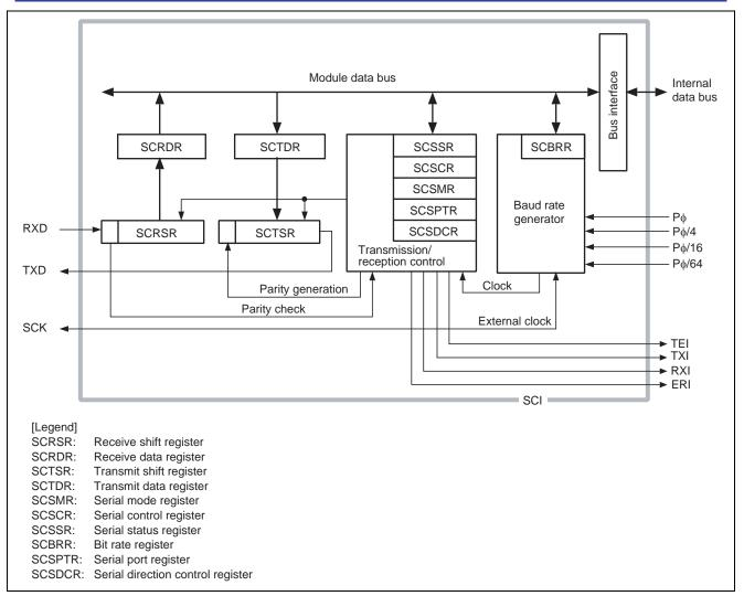
Figure 2 Block Diagram of the SCI
