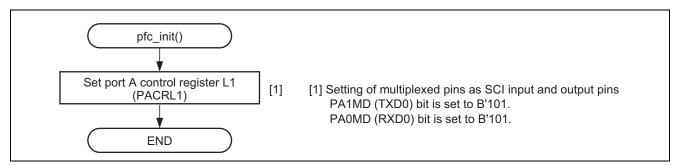
Figure 6 Flow for Setting up the Pin Function Controller
