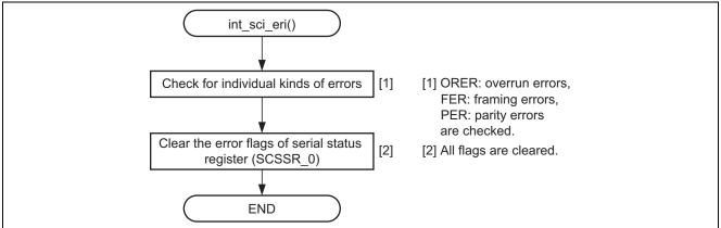
Figure 10 Flow for Handling Receive Error Interrupts
