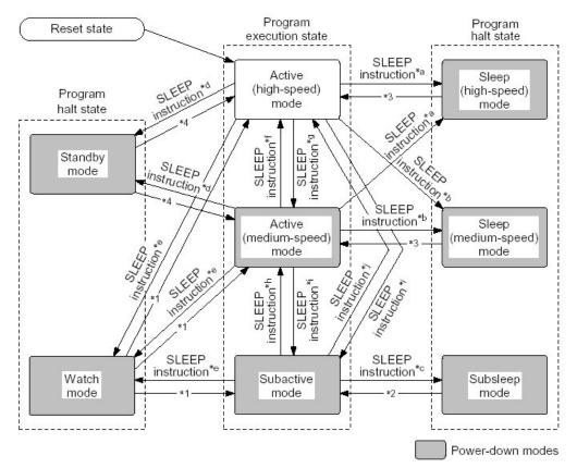
All the SLEEP instructions are stated from \*a to \*e as the figure above. For example, to transit Active (high-speed) mode to Sleep (high-speed) mode, SLEEP instruction \*a is executed. In the sample program, the routine for transition \*a is ModeA(), the routine for transition \*b is ModeB(), and so on.(*Please refer to the Hardware Manual for detail about the Mode Transition Condition and Interrupt sources.*)
