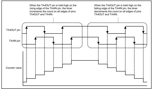
Figure 1.1 Overview of Quadrupled Processing
