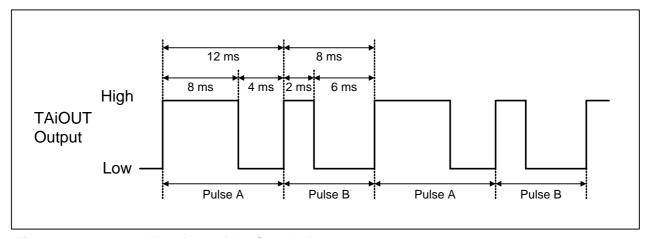
Figure 4.1 Output Waveform of the Sample Program
