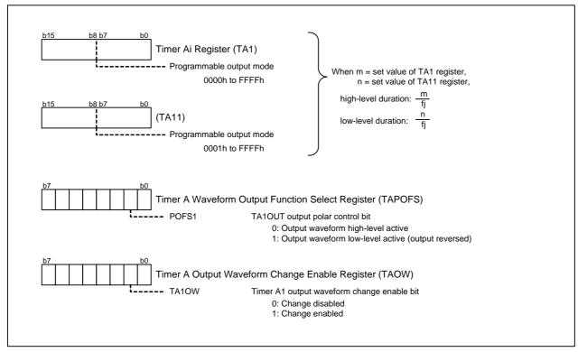
Figure 5.2 Procedure for Setting Register in Programmable Output Mode of Timer A (2/2)
