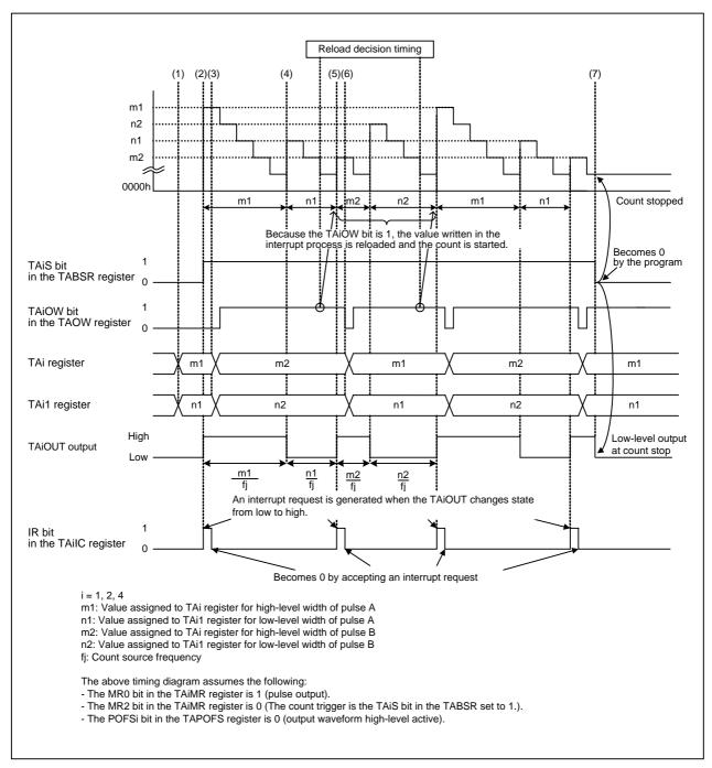
Figure 4.2 Operation Example in Programmable Output Mode
