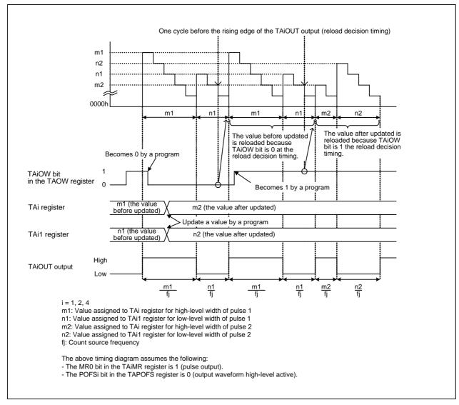
Figure 3.1 Example of Programmable Output
