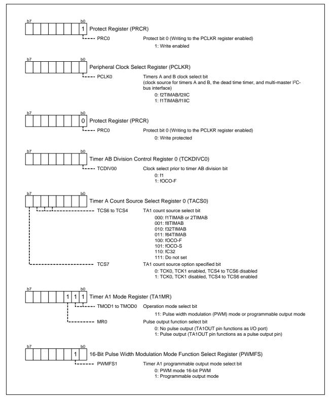
Figure 5.1 Procedure for Setting Register in Programmable Output Mode of Timer A (1/2)
