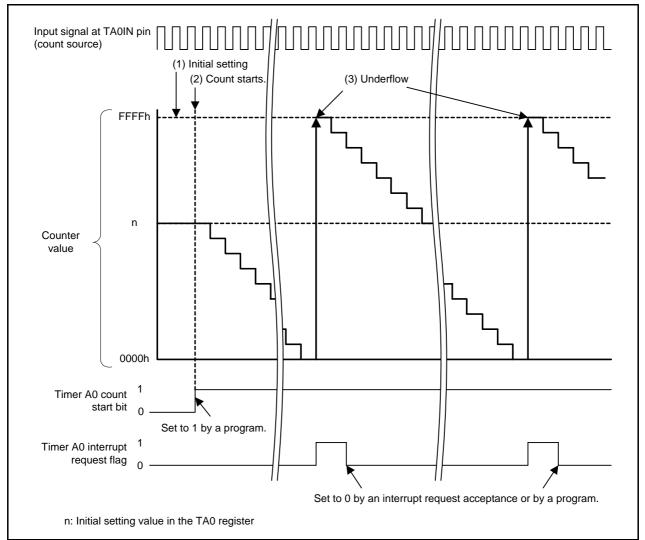
Figure 5.1 shows the Timer A0 Operation in Event Counter Mode Using Free-running Count Operation.
