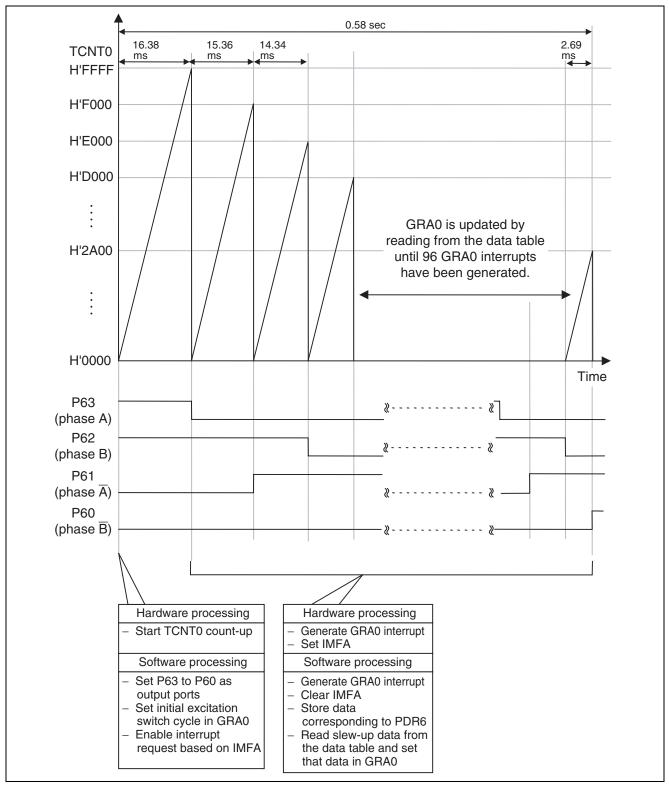
Figure 8 Principle of Slew-up Control during Forward Rotation
