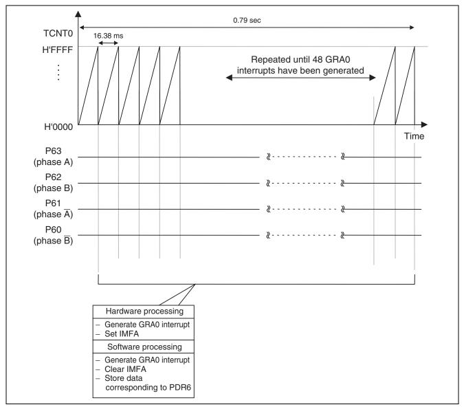
Figure 11 Principle of Stop Control
