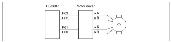
Figure 1 Connections for Controlling a Two-Phase Stepper Motor
