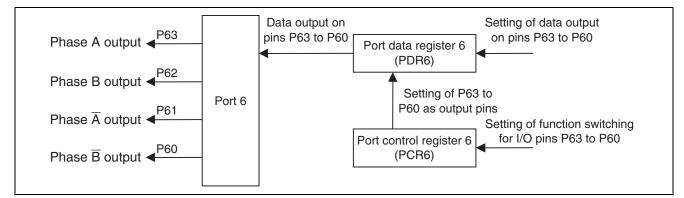
Figure 4 Block Diagram of Port 6 Functions
