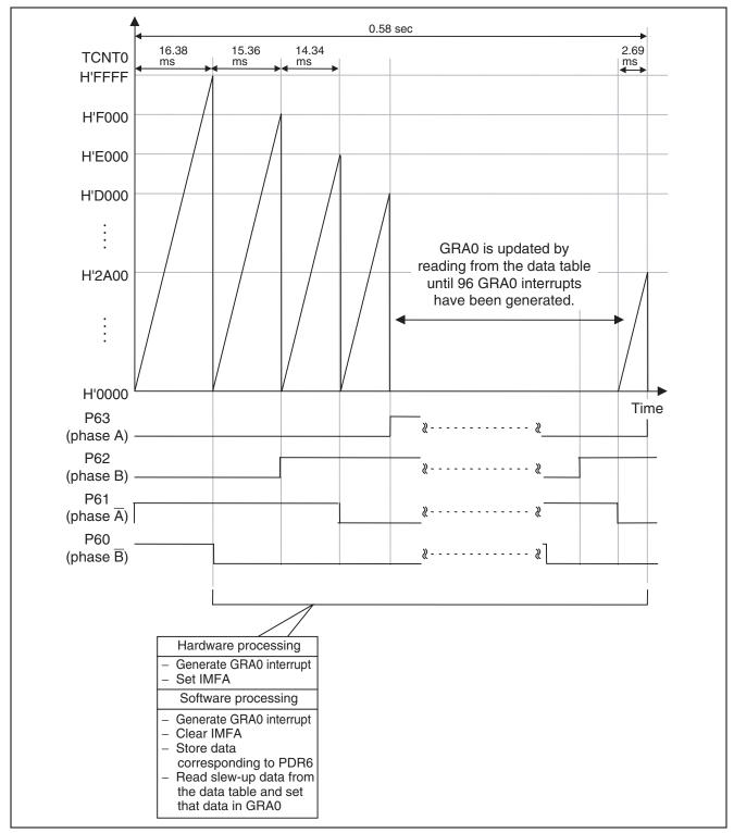
Figure 12 Principle of Slew-up Control during Reverse Rotation
