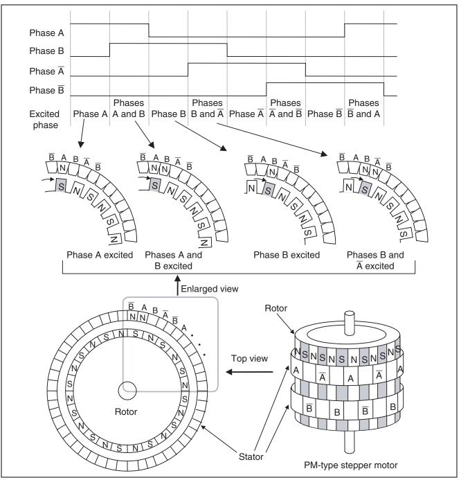
Figure 5 Example of Stepper Motor Operation
