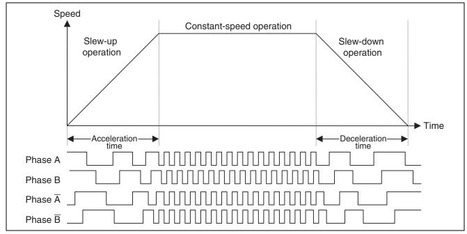
Figure 6 Example of Slew-up and Slew-down Operation
