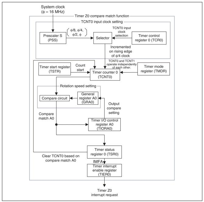
Figure 3 Block Diagram of Timer Z0
