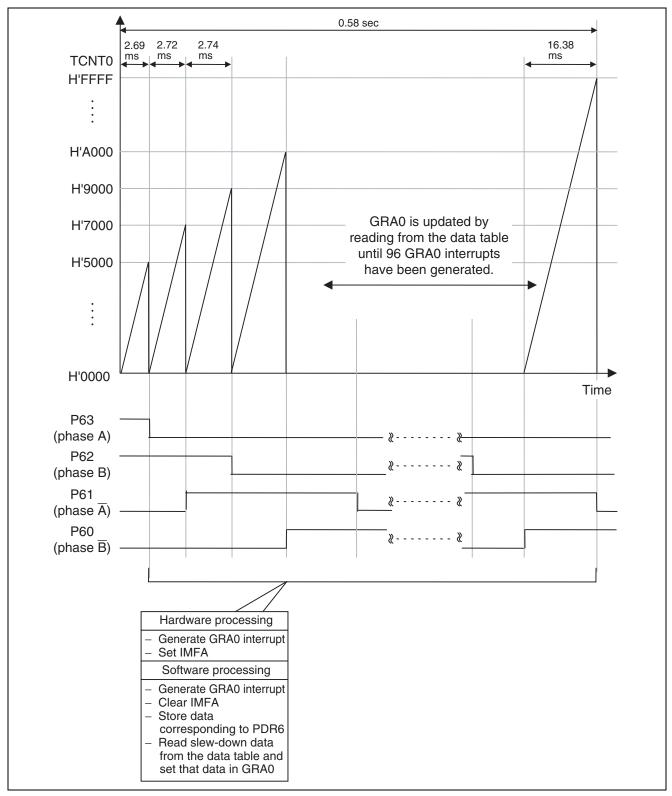
Figure 10 Principle of Slew-down Control during Forward Rotation
