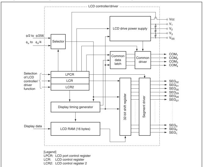
Figure 2.1 Block Diagram of LCD Controller/Driver
