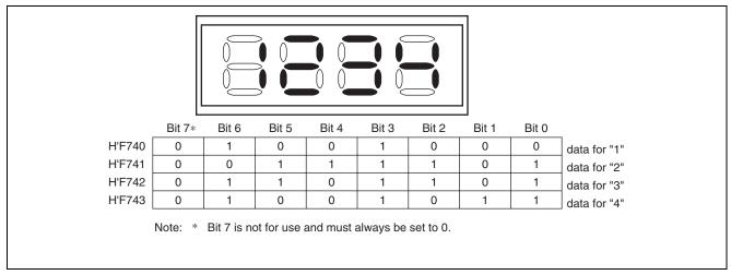
Figure 2.4 Relation between LCD Display and LCD RAM Settings
