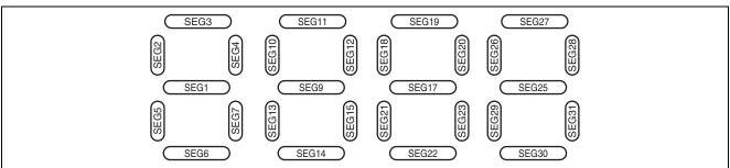
Figure 2.2 Correspondence between Segment Signals and Segments on the 4-Digit 7-Segment LCD Used in this Sample Task
