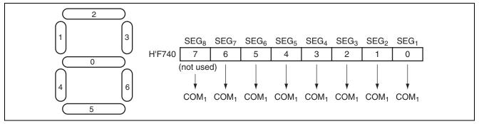
Figure 2.5 Relationship between LCD Lit/Unlit States and LCD RAM Settings
