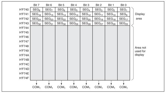
Figure 2.3 LCD RAM Mapping under Static Driving
