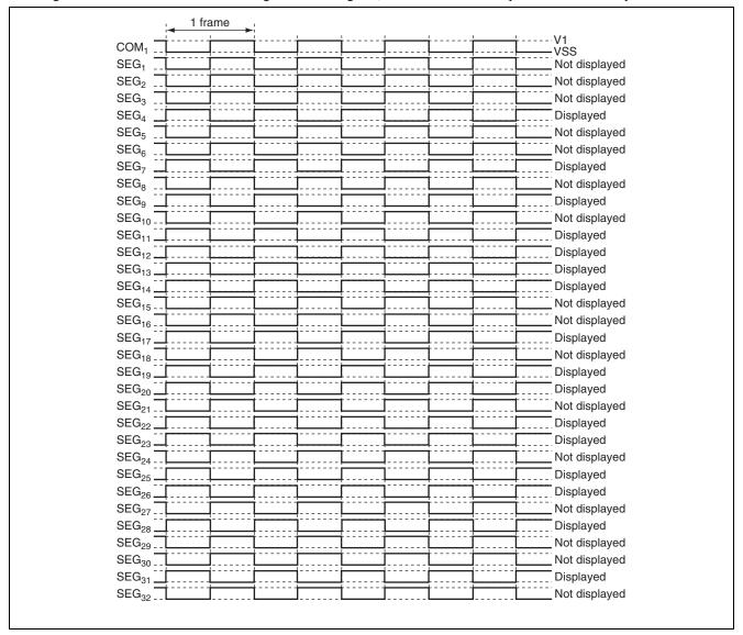
Figure 3.1 Waveforms of Segment Drive Signals
