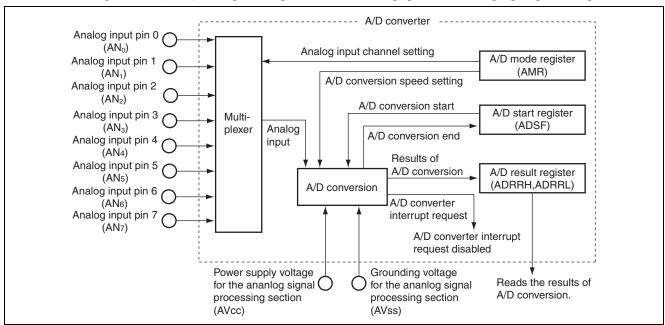
Figure 2.1 Block Diagram of the A/D Converter
