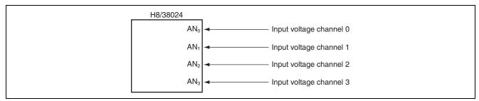
Figure 1.1 Voltage Measurement by 4-Channel A/D Conversion
